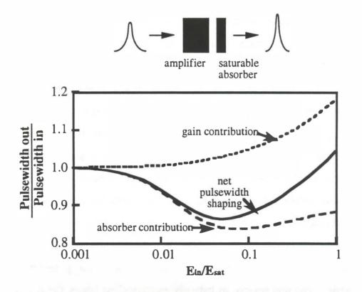
Figure 3.5. Pulse shaping in single pass propagation through gain and saturable absorber cascade.
