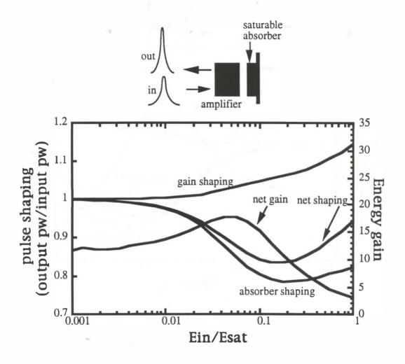
Figure 4.4. Calculated round trip pulse propagation in a uniform laser gain and absorber segment for varied input pulse energy normalized to  $E_{sat}$  the gain segment input.  $G_0 = 17$ ,  $G_{abs} = 0.02$ , and  $\sigma = 3$ .
