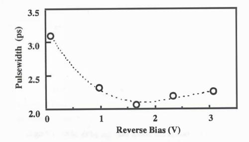
Figure 2.10. Pulsewidth dependence on modulated electrode DC reverse bias.
