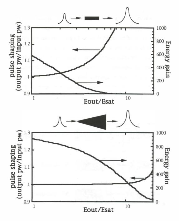
Figure 4.7. Calculated pulse shaping and energy gain in uniform and flared (flare ratio = 32) single pass highly saturated amplifiers, plotted vs. output energy to emphasize the output pulse energies being generated.
