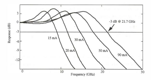
Figure B.2. Modulation response at several different bias currents.
