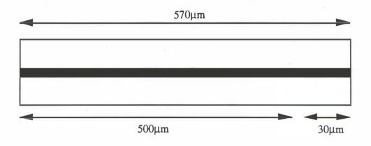
Figure 2.5. A typical segmented laser used in the external cavity mode-locking experiments.
