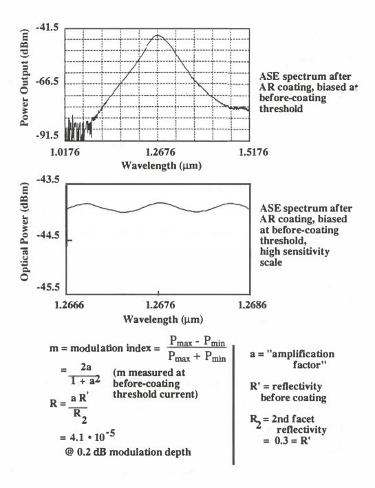
Figure A.2. Determination of AR-coated facet reflectivity from ASE spectrum.
