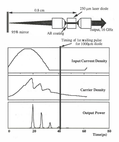
Figure 2.3. Analysis of multiple pulse formation in an actively mode-locked external cavity laser.
