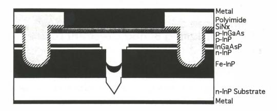
Figure B.1. Schematic of the SIBC laser structure.
