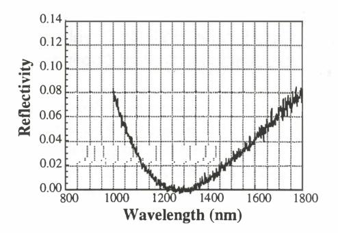
Figure A.1. Reflectivity of single-layer AR coating on Si, with center wavelength = 1300 nm.
