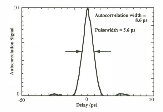
Figure 3.10. Autocorrelation of pulses from passively mode-locked ROW array laser.
