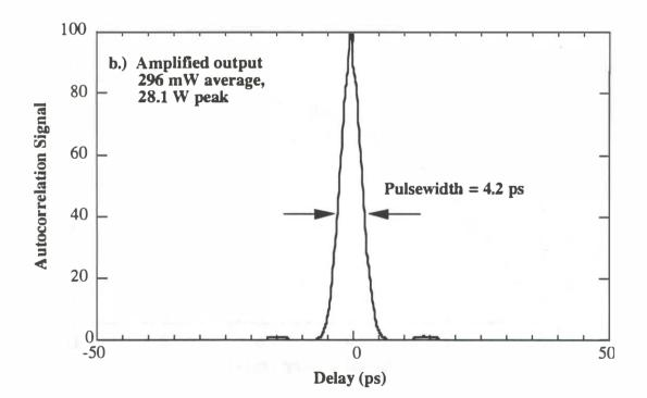
Figure 4.16. Autocorrelation of highest power amplified pulses.
