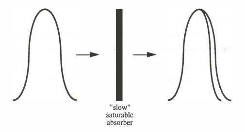
Figure 1.3. Pulse shaping resulting from passage through a "slow" saturable absorber. The leading edge of the pulse is steepened by the saturable absorption, but the absorption recovers too slowly to affect the trailing edge.
