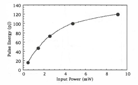
Figure 4.15. Amplified pulse energy for varied input power to the broad area flared MOPA amplifier.
