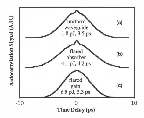
Figure 4.9. Autocorrelations, pulse energies, and pulsewidths obtained from passively mode-locked multisection lasers with (a) uniform, (b) flared absorber, and (c) flared gain waveguides.
