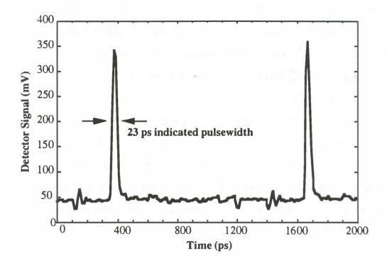
Figure 3.12. Sampling oscilloscope of pulses from hybridly mode-locked ROW array laser.
