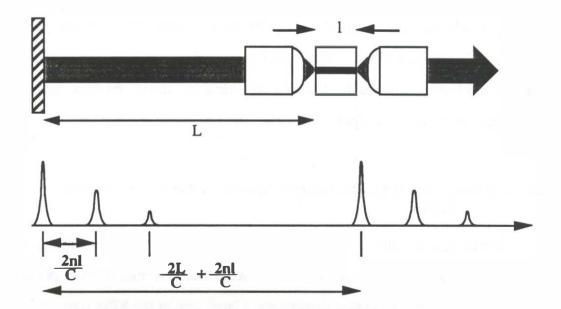
Figure 2.1. Multiple pulse output from a mode-locked semiconductor laser.
