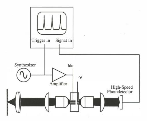
Figure 3.11. Oscilloscope connection for measurement of hybridly mode-locked ROW array laser.
