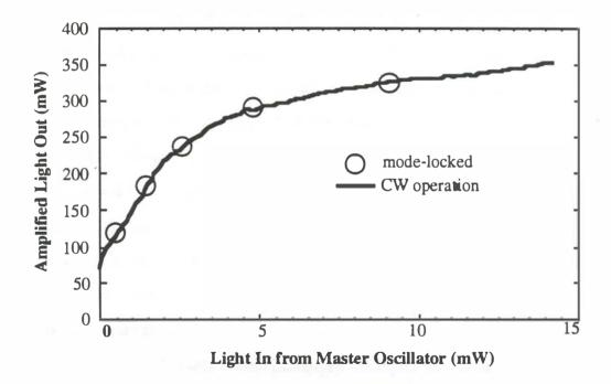
Figure 4.11. Amplifier output power vs. input level, CW and mode-locked.
