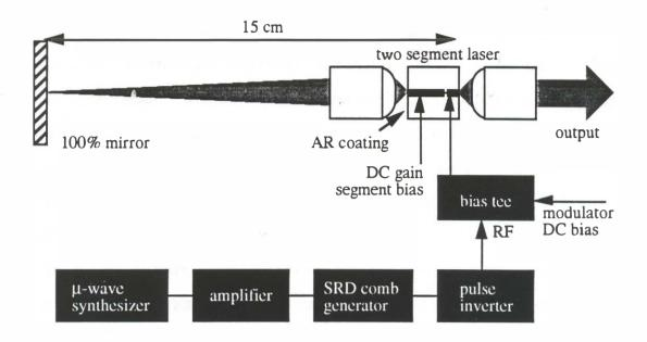
Figure 2.6. Diagram of actively mode-locked two segment external cavity laser experiment.
