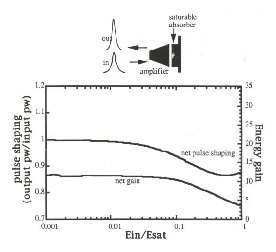
Figure 4.6. Calculated round trip pulse propagation in a flared laser gain and absorber segment for varied input pulse energy normalized to  $E_{sat}$  in the single mode part of the gain.  $G_0 = 17$ ,  $G_{abs} = 0.02$ , and  $\sigma = 1$ , with a flare ratio of 3.
