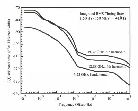
Figure 2.13. Sideband noise measured from single-pulse external cavity mode-locked laser, taken at several different harmonics.
