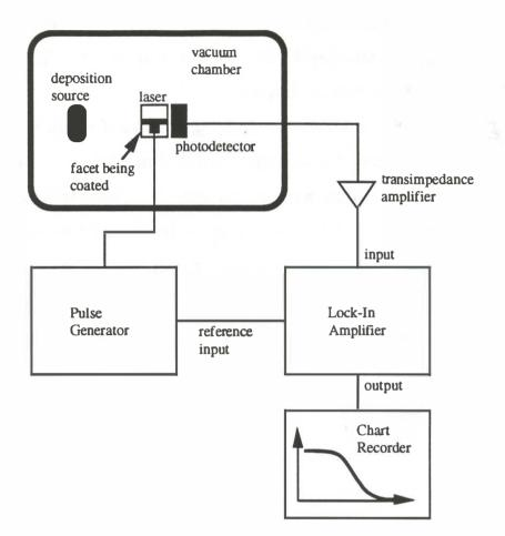
Figure A.3. Apparatus for in-situ monitoring of laser facet coating thickness.
