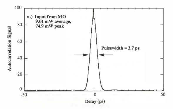
Figure 4.13. Autocorrelation of pulses injected into flared broad-area MOPA amplifier.
