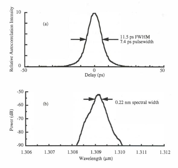
Figure 2.12. Autocorrelation and optical spectrum of transform-limited pulses generated using external grating feedback.
