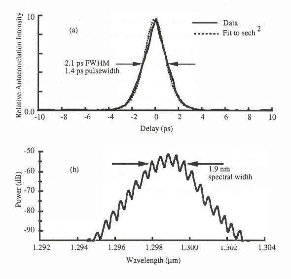
Figure 2.11. Autocorrelation (a) and optical spectra (b) of shortest pulses observed.
