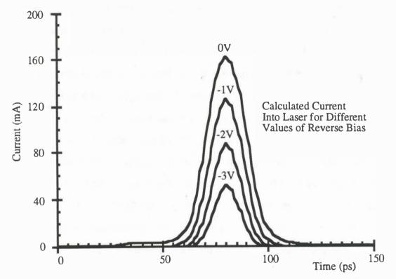
Figure 2.9. Dependence of modulation current waveforms on reverse bias to the gain modulator.
