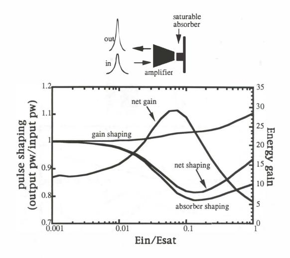
Figure 4.5. Calculated round wip pulse propagation in a flared laser gain and absorber segment for varied input pulse energy normalized to  $E_{sat}$  in the single mode part of the gain.  $G_0 = 17$ ,  $G_{abs} = 0.02$ , and  $\sigma = 3$ , with a flare ratio of 3.
