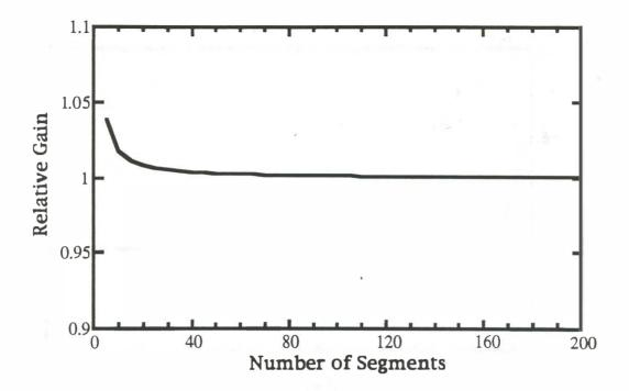
Figure 4.1. Solution for flared amplifier saturated gain vs. number of segments used in calculation. Amplifier flare ratio = 3,  $G_0=100$ ,  $E_{in}=1.0E_{sat}$ . The results are normalized to actual gain = 7.6003.
