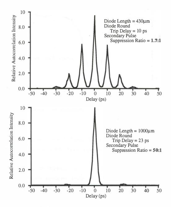
Figure 2.8. Comparison of pulse output from devices of 450 µm and 900 µm cleaved lengths.
