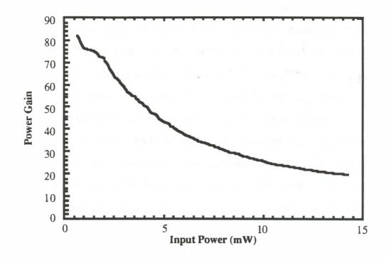
Figure 4.12. CW power gain from the broad-area flared amplifier vs. injected power.
