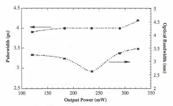
Figure 4.14. Amplified pulsewidths and bandwidths for varied output powers.
