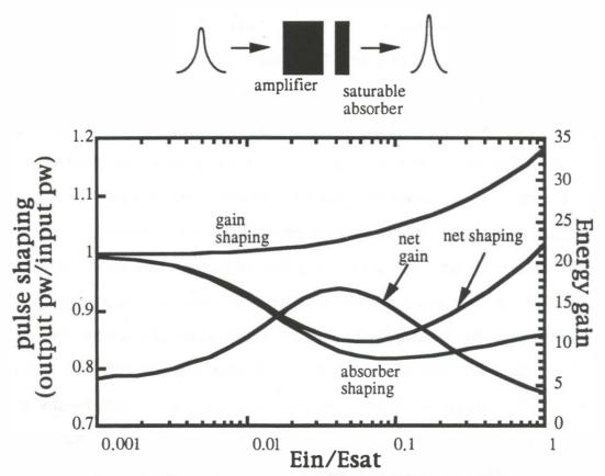
Figure 4.3. Calculated unidirectional propagation through a uniform laser gain and absorber segment for varied input pulse energy normalized to  $E_{sat}$  the gain segment input.  $G_0 = 130$ ,  $G_{abs} = 0.04$ , and  $\sigma = 3$ .
