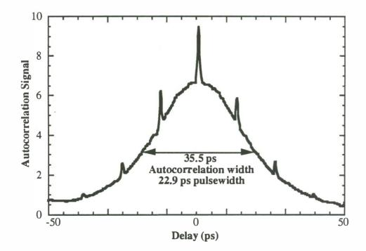
Figure 3.9. Autocorrelation of pulses from actively mode-locked ROW array laser.
