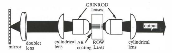
Figure 3.7. Schematic of the ROW array external cavity mode-locked laser.
