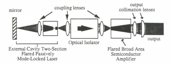
Figure 4.10. Diagram of the flared waveguide mode-locked MOPA laser.
