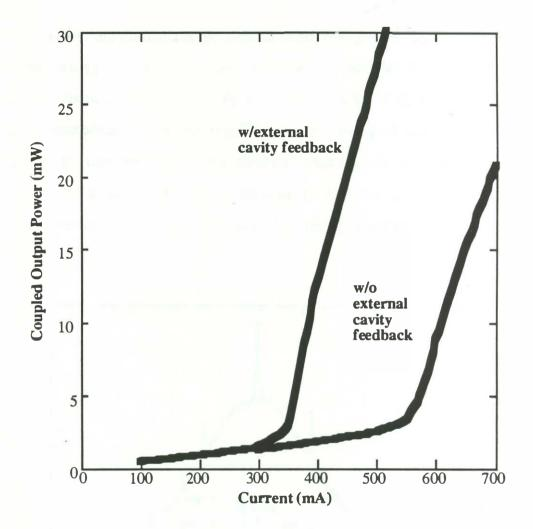
Figure 3.8. ROW array external cavity laser light vs. current characteristics.
