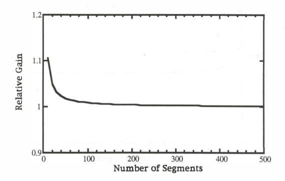
Figure 4.2. Solution for flared amplifier saturated gain vs. number of segments used in calculation. Amplifier flare ratio = 32,  $G_0=100$ ,  $E_{in}=1.0E_{sat}$ . The results are normalized to actual gain = 11.830.
