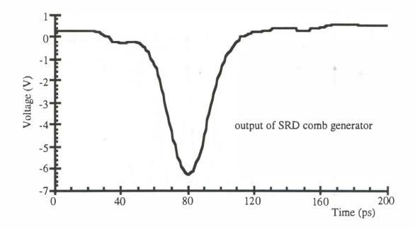
Figure 2.7. Output of the SRD comb generator used to gain modulated the laser experiments.
