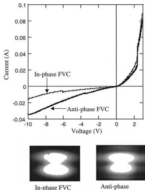
Fig. 2.  $I$ - $V$  curves of in-phase and anti-phase FVC's and the electroluminescence images under 80-mA forward current.
