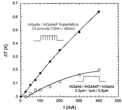
**Fig.6** Experimental  $|T_c - T_H|$  versus current for  $100 \times 200 \mu\text{m}^2$  single-stage HIT coolers with bulk InGaAsP ( $\lambda_{\text{gap}}=1.3 \mu\text{m}$ ) barrier and with superlattice barrier (20 periods of 10nm InGaAs and 40nm InGaAsP).
