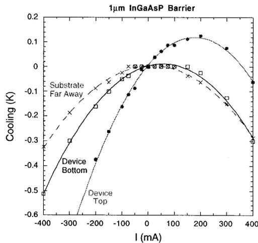
**Fig.5** Temperature on top and on the bottom of the device as well as the substrate temperature far away from the device as a function of current. All temperatures are relative to the value at zero current. The device is a single-stage HIT cooler with bulk InGaAsP ( $\lambda_{\text{gap}}=1.3 \mu\text{m}$ ) barrier layer.
