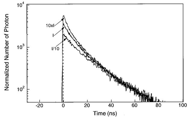
FIG. 3. Time-resolved PL at 1.348 eV on structure B samples at 10 K with different excitation intensities. The data are normalized with the tail exponential parts. The dashed line on top of the middle trace is the double-exponential fit.
