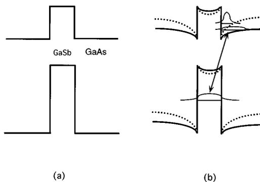
FIG. 1. Schematic drawings of the spatial dependence of the conduction and valence bands for the staggered band lineup (a) and including a space-charge-induced band-bending effect (b). The dashed line in (b) shows a stronger band-bending effect.
