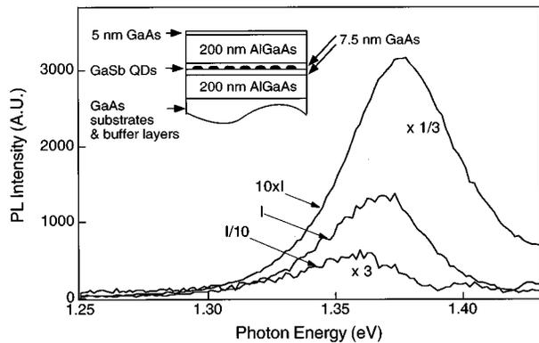
FIG. 2. Quantum dot photoluminescence spectra of structure B with different excitation intensities. Inset shows the schematic diagram of structure B.
