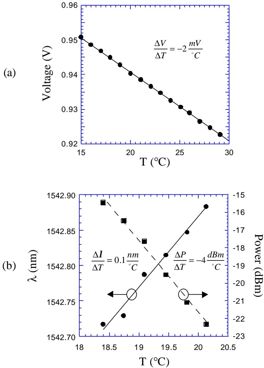
**Figure 6.3** Temperature dependent properties of some optoelectronic devices (a) A p-i-n InP diode under constant current has a temperature dependent voltage. (b) The wavelength and optical power of a DFB laser diode are also temperature dependent.
