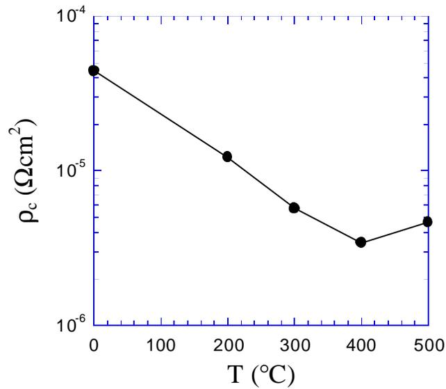
**Figure 5.12** Contact resistivity versus alloying temperature for Ti/Pt/Au contacts to p-type InGaAs ( $2 \times 10^{19} \text{cm}^{-3}$ ). Samples were alloyed for 20 seconds and measured by the TLM method.
