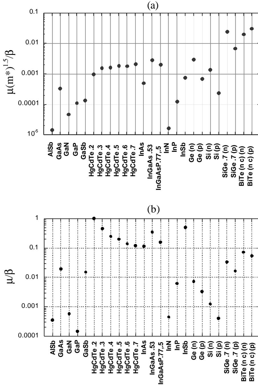
**Figure 3.1 (a)** The material parameter  $m^*m^*)^{1.5}/b$  for different compounds indicates the prospects of various semiconductors for low-barrier thermionic or thermoelectric cooling.  $m$  is the mobility in the barrier layer,  $b$  is the thermal conductivity, and  $m^*$  is the carrier effective mass. **(b)** The modified material parameter neglecting the effective mass.
