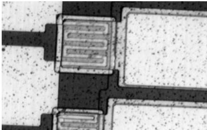
**Figure 6.2** SEM image of a cooler with a patterned Pt-heater on top. The Pt metal was electrically isolated from the top of the cooler with a thin layer of  $\text{SiN}_x$ .
