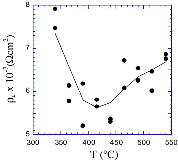
**Figure 5.9** Contact resistivity versus RTA alloying temperature for Ni/AuGe/Ni/Au contacts to InGaAs ( $3 \times 10^{18} \text{ cm}^{-3}$ ). Samples were alloyed for 1 second and measured by the TLM method.
