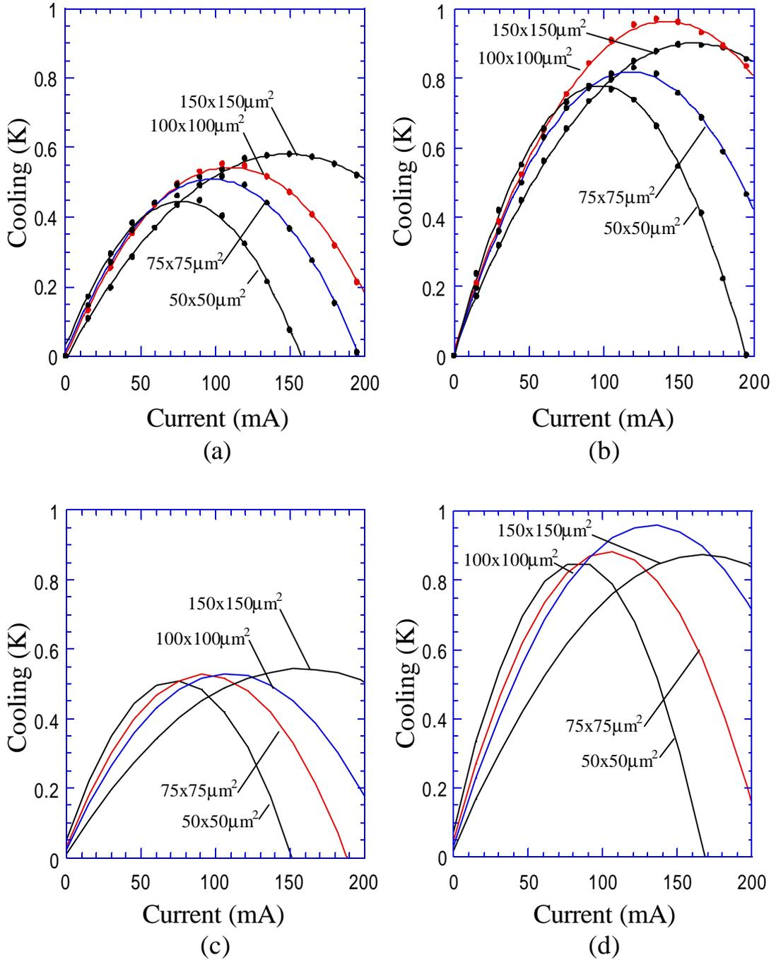
**Figure 6.24** (a) Measured cooling versus current bias at 25°C and at (b) 70°C. (c) Corresponding simulation results at 25°C and at (d) 70°C. Measurement and simulations performed by D. Vashae.
