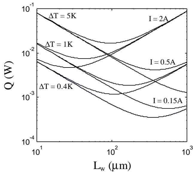
**Figure 5.5** Cooling power lost versus gold wire length for various bias currents and temperature differences. The electrical and thermal conductivities of gold were taken as  $45.5 \times 10^4 \Omega^{-1} \text{cm}^{-1}$  and  $3.17 \text{ W/cm}\cdot\text{K}$  respectively.
