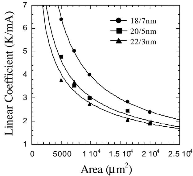
**Figure 6.13** Linear coefficients versus area for different periods of a 2- $\mu\text{m}$ -thick InGaAs/InP superlattice. The coefficients are larger for the periods containing more InP.
