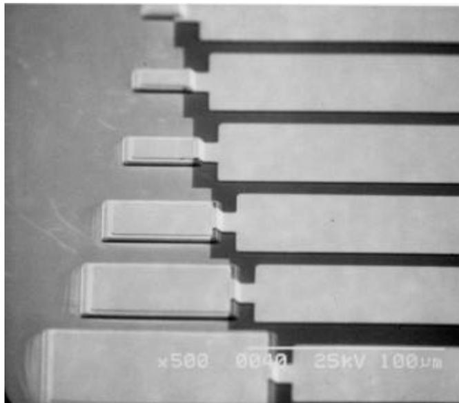
**Figure 5.6** SEM image of the surface of a third-generation processed sample. The dark staircase region on the right side of the mesas is the SiN<sub>x</sub> used to electrically isolate the side contacts from the substrate. The metal lines run for 250 μm.
