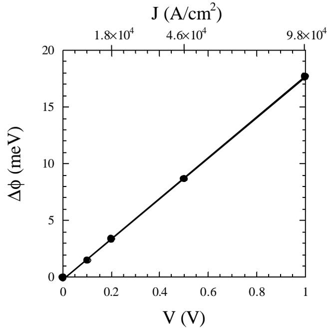
**Figure 3.5** Calculated barrier lowering as a function of voltage bias for an InGaAs/InP superlattice. The linear relationship is due to the linear conduction regime in the heterobarriers.
