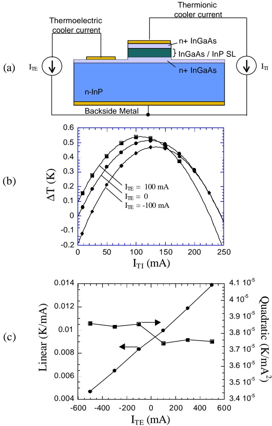
**Figure 6.17** (a) TITE device structure and geometry. (b) Cooling versus thermionic cooler current for three different thermoelectric currents, and (c) the corresponding linear and quadratic coefficients versus thermoelectric current.
