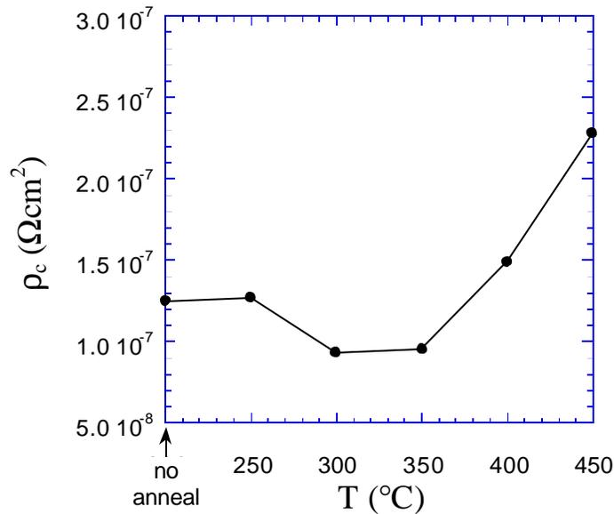
**Figure 5.11** Contact resistivity versus alloying temperature for Ti/Pt/Au contacts to *n*-type InGaAs ( $2 \times 10^{19} \text{cm}^{-3}$ ). Samples were alloyed for 20 seconds and measured by the TLM method.
