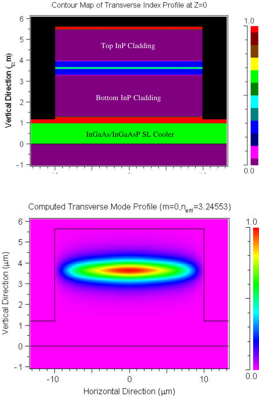
**Figure 7.11** Contour map of transverse index profile and corresponding simulation of modal confinement in the ridge waveguide. A bottom InP cladding thickness of 2  $\mu\text{m}$  was sufficient to prevent modal leakage into the cooler superlattice.
