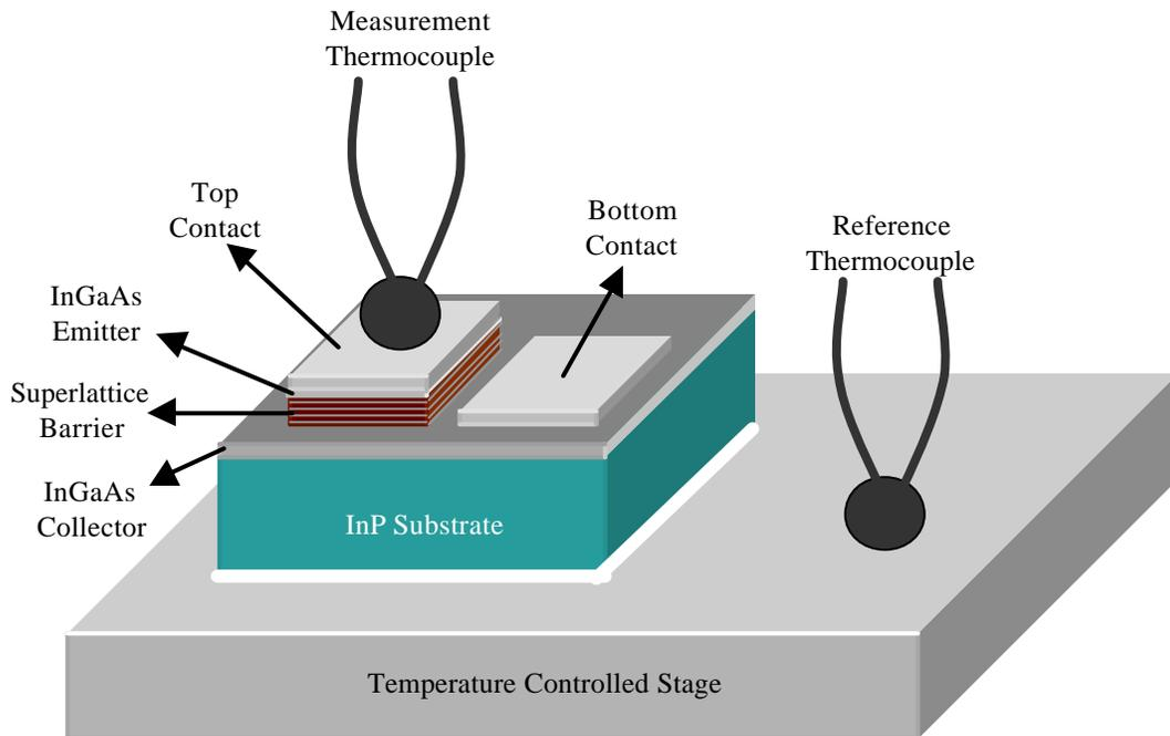
**Figure 6.1** Micro-thermocouple characterization set-up. The stage is kept at constant temperature while two micro-thermocouples are used in a differential measurement of temperature for various current biases. The external or integrated wire bond is not shown.
