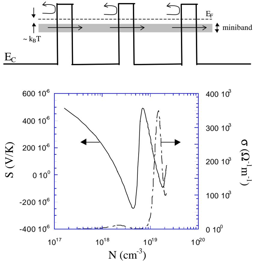
**Figure 2.12** Calculated Seebeck coefficient and electrical conductivity for three periods of 3nm/5nm InAlAs/InGaAs. The Seebeck coefficient changes sign for certain doping levels. The simplified diagram above illustrates the concept of manipulating the miniband conduction for electron filtering.
