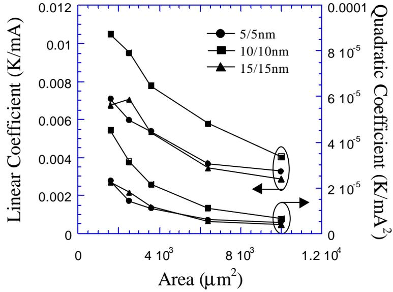
**Figure 6.12** Linear and Quadratic coefficients versus area for different periods of a 1- $\mu\text{m}$ -thick InGaAs/InGaAsP superlattice. Both coefficients are higher for the 10/10nm period indicating a lower superlattice effective thermal-conductivity.
