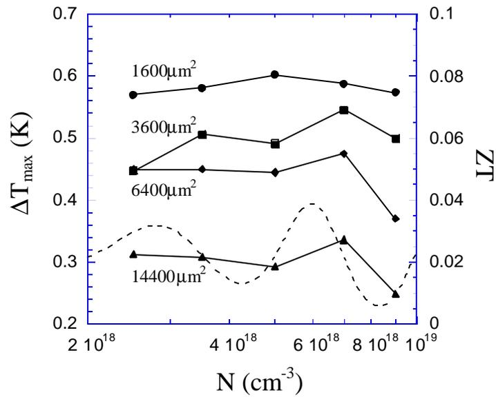
**Figure 6.15** Maximum cooling versus doping (solid lines) for a 2- $\mu\text{m}$ -thick 22/3nm InGaAs/InP superlattice. The theoretical ZT is shown by the dashed line and is related to  $\Delta T_{\text{max}}$  through Equation 6.6. A similar qualitative behavior is evident indicating thermionic cooling effects are present.
