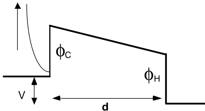
**Figure 1.2** Conduction band diagram of a heterostructure integrated thermionic (HIT) cooler under an applied bias.
