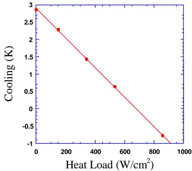
**Figure 7.21** Measured maximum cooling versus heat load for a 2- $\mu\text{m}$ -thick  $40 \times 40 \mu\text{m}^2$  SiGeC thin film cooler [21]. The heat sink temperature was  $70^\circ\text{C}$ . From X. Fan and G. Zeng
