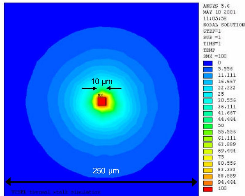
**Figure 7.18** Thermal image of surface temperature from a 3-D ANSYS simulation of substrate heat flow for the long wavelength VCSEL structure. The pillar diameter was  $10\ \mu\text{m}$ , the bottom DBR was  $7.7\ \mu\text{m}$  thick, and the GaAs substrate was  $300\ \mu\text{m}$  thick.
