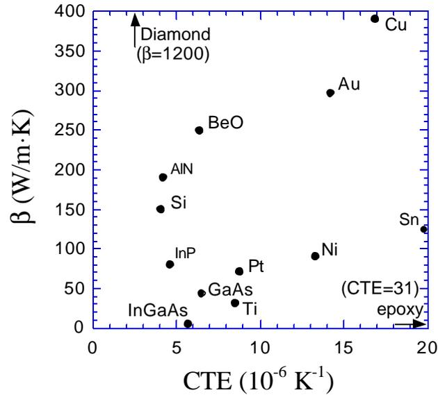
**Figure 5.13** Thermal conductivity and coefficient of thermal expansion for materials relevant to substrate transfer processes.
