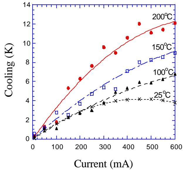
**Figure 7.20** Cooling versus current and heat sink temperature for a 3- $\mu\text{m}$ -thick,  $50 \times 50 \mu\text{m}^2$ , 12/3nm SiGe/Si superlattice cooler [20]. From X. Fan and G. Zeng.
