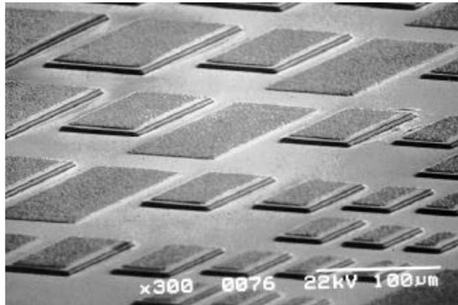
**Figure 5.2** SEM image of the surface of a processed thermionic cooler sample. The mesa heights are  $1.5 \mu\text{m}$  and the areas range from  $20 \times 40 \mu\text{m}^2$  to  $100 \times 200 \mu\text{m}^2$ .
