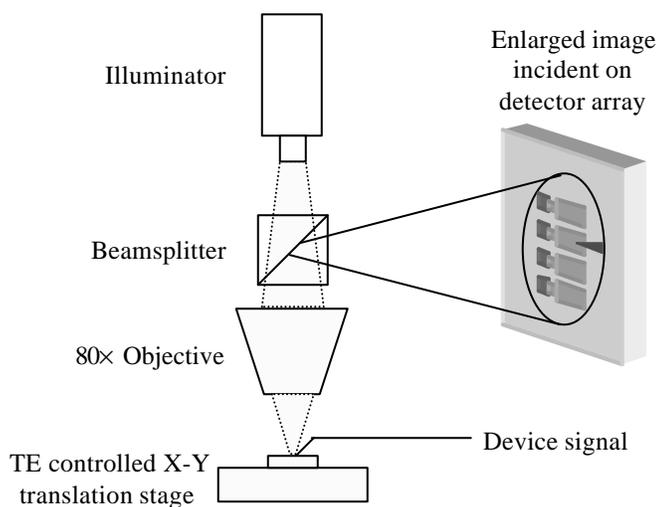
**Figure 6.4** Experimental setup for thermoreflectance measurement system. The diffraction limit of visible white light from the illuminator bounds the spatial resolution to a sub-micron scale.
