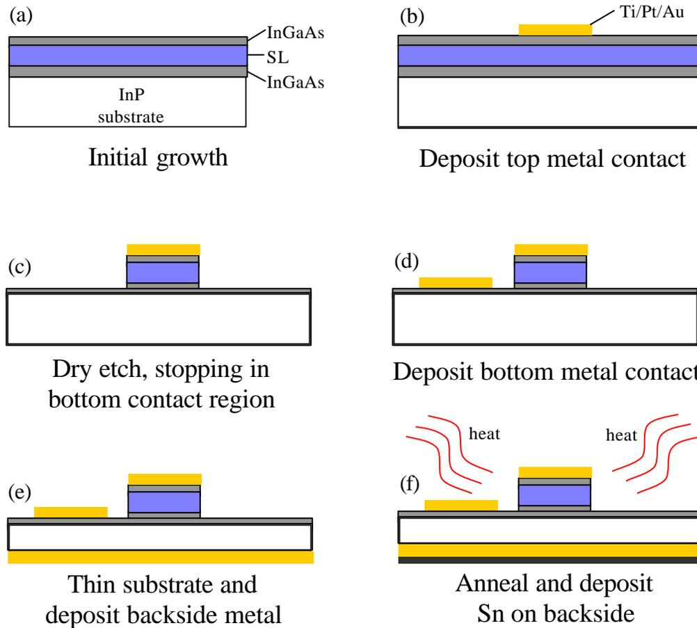
**Figure 5.1** (a) - (f) General processing procedure for heterostructure thermionic coolers. The basic steps involve forming mesas of various size and providing low resistance contacts.
