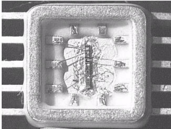
**Figure 5.3** First-generation packaged set of devices. The devices (middle) were cleaved and mounted in the base with InSn solder alloy. A wedge bonder was used for wire bonding with 1 mil diameter wire. The package itself is ceramic with a gold alloy casing and bond pads.
