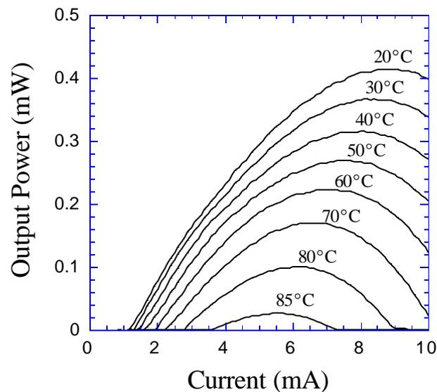
**Figure 7.16** Continuous wave output power versus current for the 1.55  $\mu\text{m}$  VCSELs considered for micro-cooler integration. From A. Karim.
