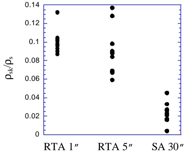
**Figure 5.10** Ratio of alloyed to unalloyed sheet resistivity versus alloying method and hold time for Ni/AuGe/Ni/Au contacts to  $n$ -type InGaAs ( $3 \times 10^{18} \text{ cm}^{-3}$ ). RTA stands for a rapid thermal anneal process while SA represents a slower strip anneal process.
