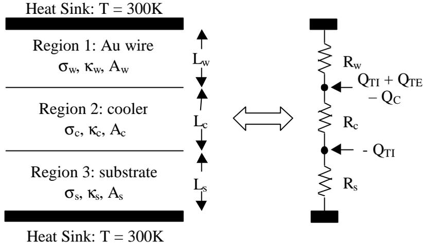
**Figure 6.6** One-dimensional model and boundary conditions. Electrical conductivity ( $\sigma$ ), thermal conductivity ( $\kappa$ ), and area ( $A$ ), are defined in each region. The equivalent circuit model is shown on the right with the arrows indicating sources or sinks of heat flux.  $Q_{TI}$  refers to thermionic heating/cooling,  $Q_{TE}$  to thermoelectric cooling, and  $Q_C$  to heat generation by contact resistance.
