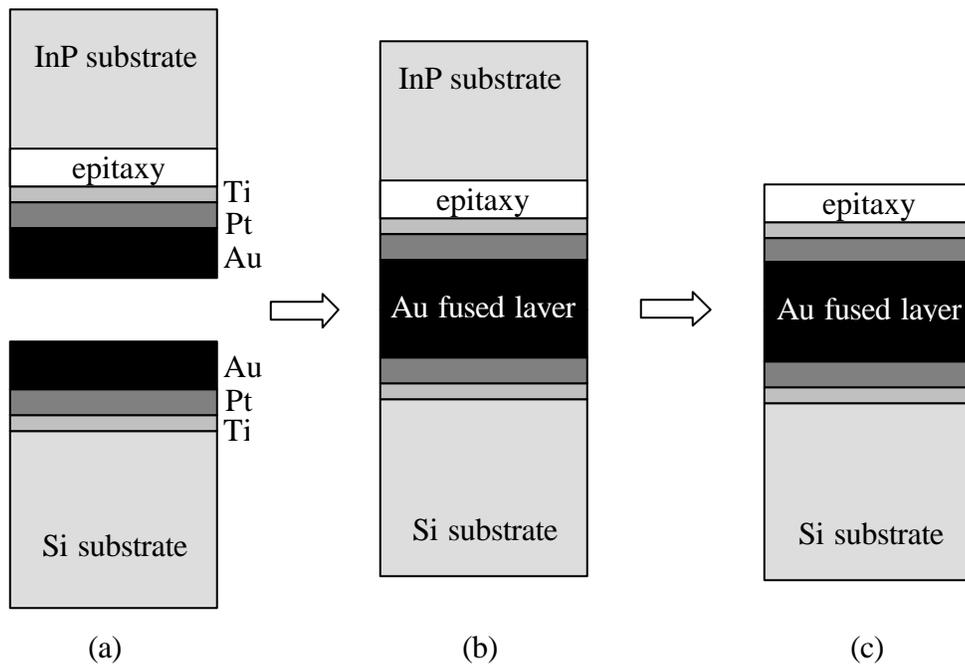
**Figure 5.16** Au-Au fusion process for transferring epitaxial layers from the InP growth substrate to a Si substrate. The steps are (a) E-beam evaporation of Ti/Pt/Au metallization, (b) Au-Au fusion under pressure and at high temperatures, and (c) InP substrate removal. The process can be generalized to any surrogate substrate.
