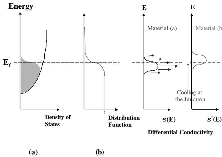
**Figure 2.1** (a) Energy versus density of states and Fermi distribution function for a degenerately doped  $n$ -type semiconductor. (b) The energy distribution of electrons moving in the semiconductor under an electric field is given by  $s(E)$  the differential conductivity that determines the average transport energy of carriers. As the average transport energy increases from material “a” to material “b”, thermal energy is absorbed from the lattice and the junction is cooled.
