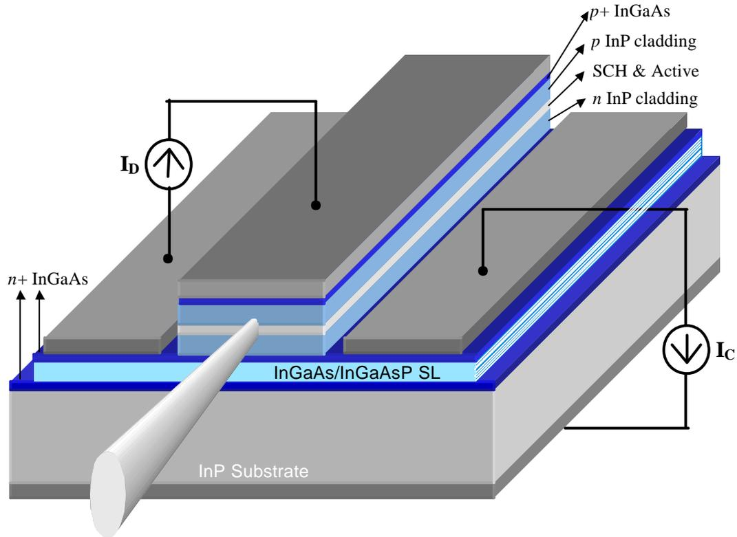
**Figure 7.9** Schematic of thermionic cooler integrated with a ridge waveguide laser showing the laser ( $I_D$ ) and cooler ( $I_C$ ) bias.
