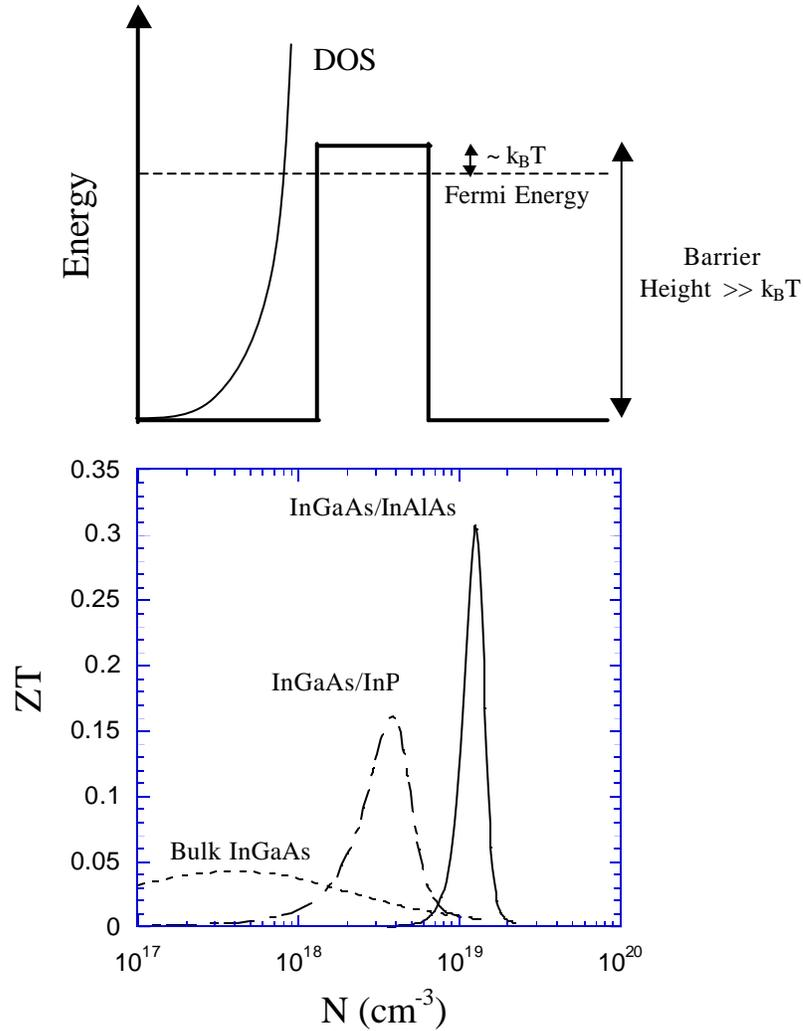
**Figure 2.9** Schematic and calculated  $ZT$  for bulk InGaAs and for high barrier heterostructure thermionic coolers based on InGaAs/InP ( $\Delta E_C=0.24\text{eV}$ ) and InGaAs/InAlAs ( $\Delta E_C=0.51\text{eV}$ ) at various doping densities. The peak in the  $ZT$  characteristic at a given doping corresponds approximately to the Fermi level being  $\sim k_B T$  below the barrier. The thermal conductivity of the composite material is taken to be  $5 \text{ W/mK}$ .
