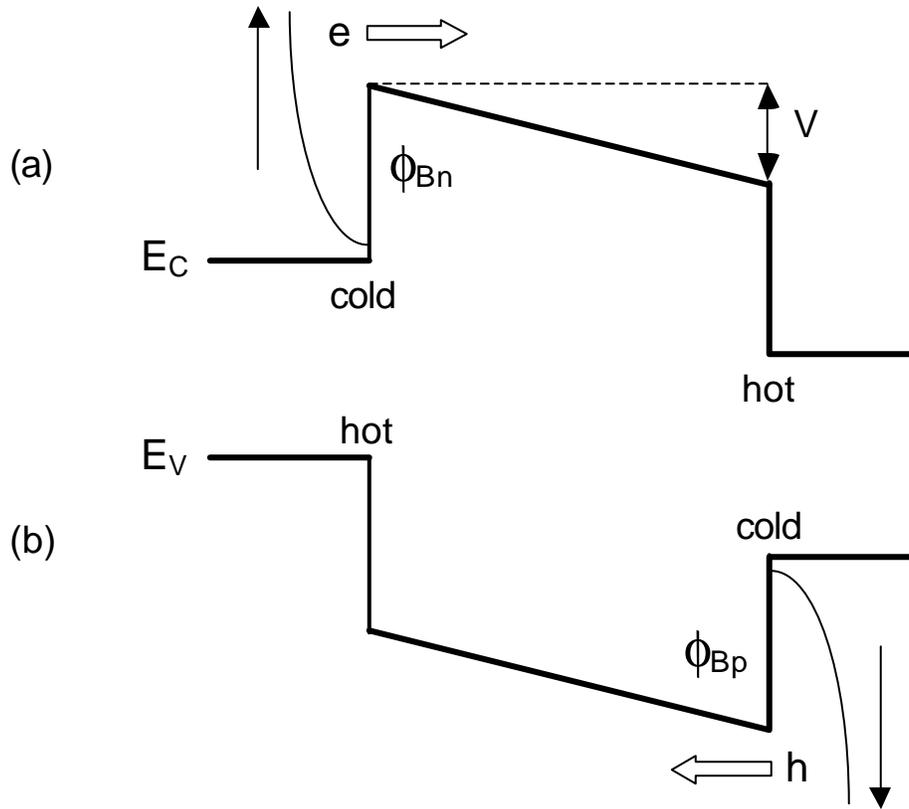
**Figure 2.4** (a) Conduction band diagram of a *n*-type and (b) a valence band diagram of a *p*-type thermionic emission cooler under an applied bias  $V$ . For the same bias polarity, the *n*-type device cools on the left and heats on the right, while the *p*-type device heats on the left and cools on the right.
