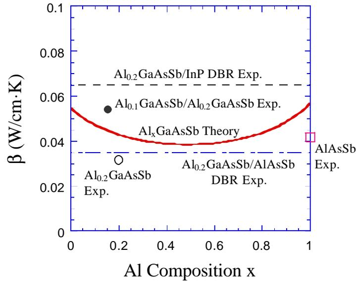
**Figure 4.3** Measured and theoretical thermal conductivity for various  $\text{AlGaAsSb}$  compounds and Al compositions. The superlattice structure investigated for thermionic cooling was 10nm/10nm  $\text{Al}_{0.1}\text{GaAsSb}/\text{Al}_{0.2}\text{GaAsSb}$ . DBR values from G. Almuneau.
