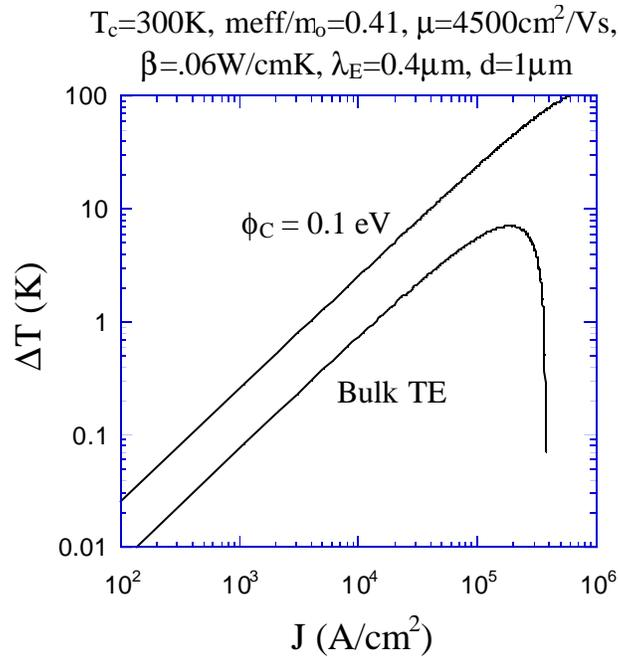
**Figure 2.6** Cooling temperature as a function of current for InGaAs with (0.1 eV) and with out (bulk thermoelectric) a conduction band barrier. The electrical and thermal conductivities were measured experimentally, and the electron relaxation length was taken from previous work [18].
