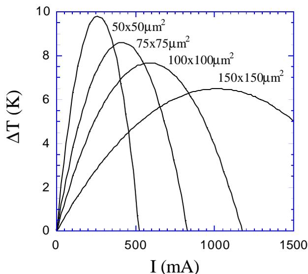
**Figure 6.25** Simulation prediction of cooling versus current for the *p*-type InGaAs/InGaAsP superlattice coolers. The simulation assumes that the side contact losses are minimized and  $r_c$  is reduced to  $5 \times 10^{-7} \Omega \text{cm}^2$ . Simulation by D. Vashaee.
