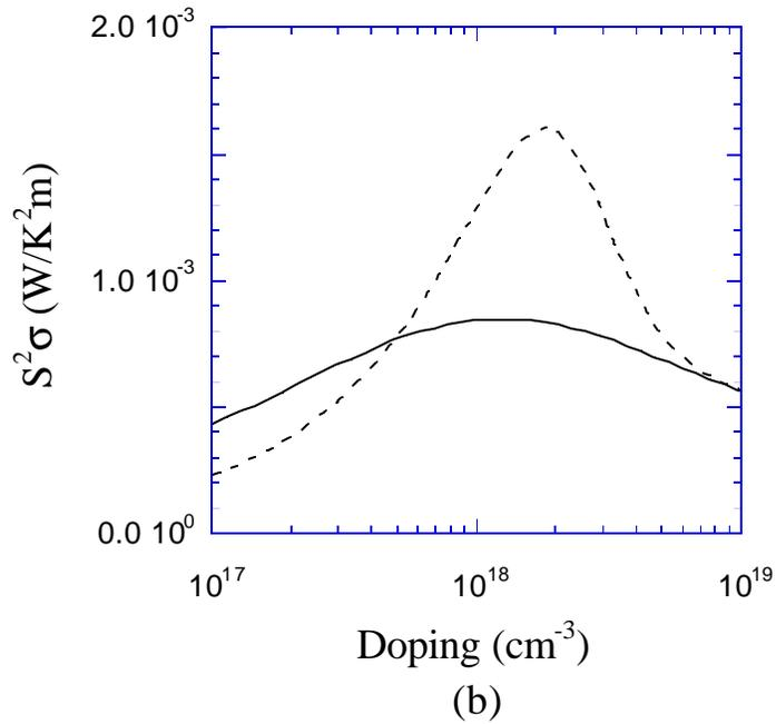
**Figure 2.3** (a) Calculation of Seebeck coefficient squared ( $S^2$ ) and electrical conductivity ( $\sigma$ ) as a function of doping for bulk InGaAs (solid lines) and for InGaAs with an undoped InGaAsP barrier (dashed lines). The impact of the barrier is to increase the Seebeck coefficient with only a slight decrease in electrical conductivity resulting in an improved power factor. (b) The power factor is seen to increase by a factor of two in this example.
