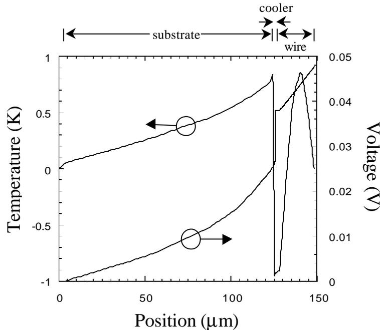
**Figure 6.21** Simulated temperature and voltage profiles along a path through the substrate, cooler, and wire bond. The actual wire bond length was 400  $\mu\text{m}$ , but was scaled by 20 $\times$  to reduce the number of elements in the 3-D simulation.
