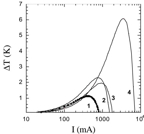
**Figure 6.20** Experimental and simulation results for a  $\mu\text{m}$  thick InGaAs/InGaAsP superlattice cooler. The points and curve 1 correspond to the simulated fit of the experimental data with all non-ideal effects. Curves 2 and 3 are the repeated simulation results when the contact resistance and substrate thermal resistance are taken away respectively. Curve 4 corresponds to both non-ideal effects removed.
