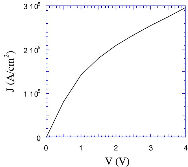
**Figure 3.4** Simulated current-voltage relationship for the structure shown in Figure 3.3. The current is linearly dependent on voltage below  $10^5 \text{ A/cm}^2$ .
