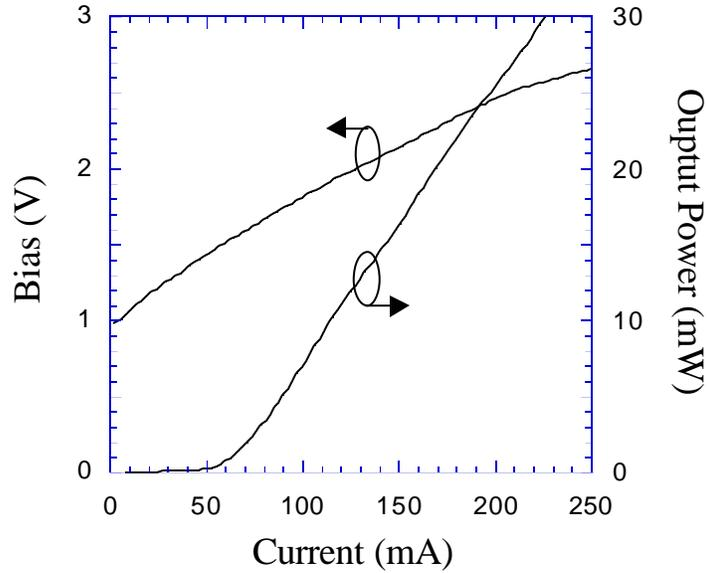
**Figure 7.12** *L-V-I* characteristics of a ridge waveguide laser integrated with a thermionic cooler. Data is shown for a 100  $\mu\text{m}$  long cavity with a 20  $\mu\text{m}$  wide ridge.
