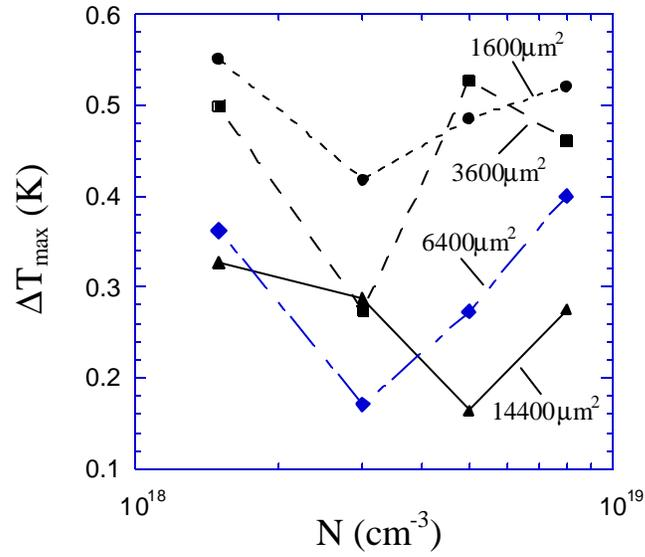
**Figure 6.14** Maximum cooling versus doping for a 1- $\mu\text{m}$ -thick 10/30nm InGaAs/InGaAsP superlattice.
