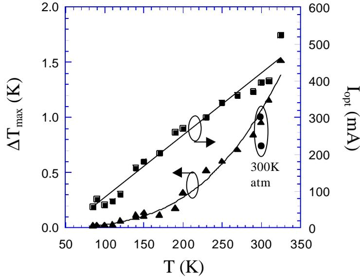
**Figure 6.10** Maximum cooling and optimum current versus heat sink temperature for a 18/7nm InGaAs/InP superlattice design. The measurements were performed in a liquid-N<sub>2</sub> cooled low temperature micro probe system. The chamber pressure was approximately 10<sup>-4</sup> to 10<sup>-5</sup> torr. Two measurements of  $\Delta T_{max}$  at room temperature and pressure are shown for reference.
