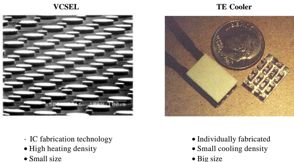
**Figure 1.1** Characteristic incompatibilities between VCSEL's and TE coolers. [VCSEL SEM by N. Margalit et al. 1997]
