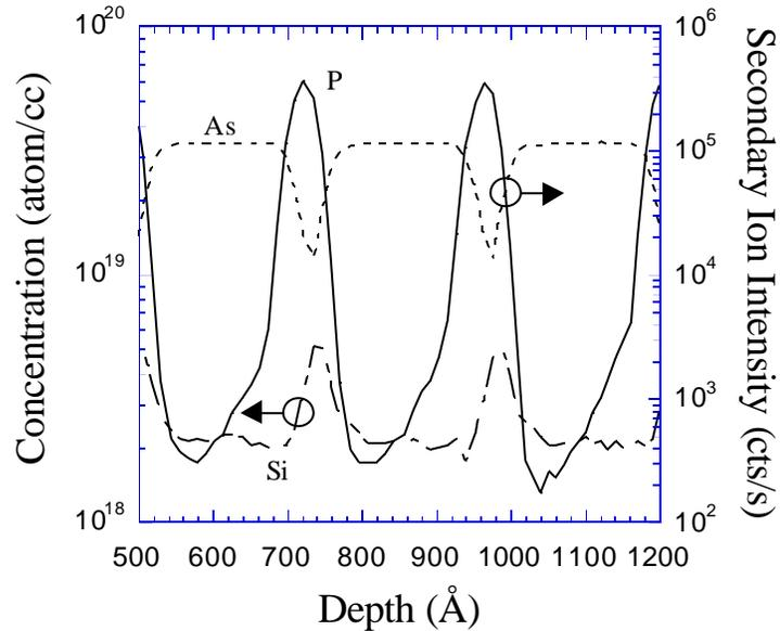
**Figure 4.6** SIMS material analysis of a silicon-doped 20nm/5nm InGaAs/InP superlattice, monitoring As, P, and Si. The InP layers (P peaks) should be undoped, however a significant amount of Si is found to be present.
