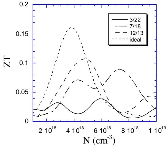
**Figure 2.11** Calculation of ZT for InP/InGaAs superlattices with various ratios of the constituent materials for a 25nm period where the quantum mechanical transmission probability is considered. In the ideal case the period is irrelevant, and the transmission probability is assumed to be zero for energies below the barrier and unity for energies above. Significant decreases can be seen in ZT due to miniband conduction.
