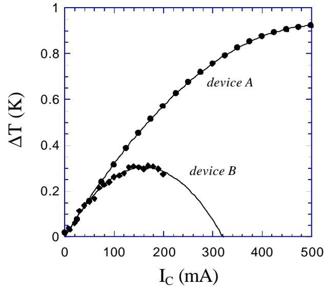
**Figure 7.6** Measured cooling versus cooler current using a micro-thermocouple for a well packaged device (*device A*), and using the integrated *p-i-n* diode with poorer packaging (*device B*). Both device areas were  $70 \times 140 \mu\text{m}^2$ .
