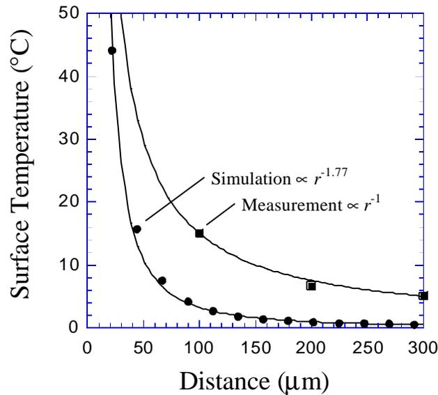
**Figure 7.19** Comparison of simulated and measured surface temperature versus distance from the VCSEL heat source. The two curves show differing area dependence.
