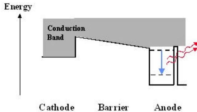
**Figure 8.2** An intersubband light-emitting thermionic cooler. Light emission must be incoherent to not violate the 2<sup>nd</sup> law of thermodynamics. From A. Shakouri
