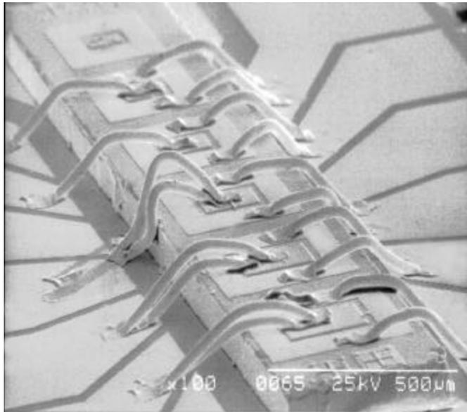
**Figure 5.4** SEM image of a second-generation packaged set of devices. The package was made from an undoped Si substrate where Au contact pads were patterned on the surface.
