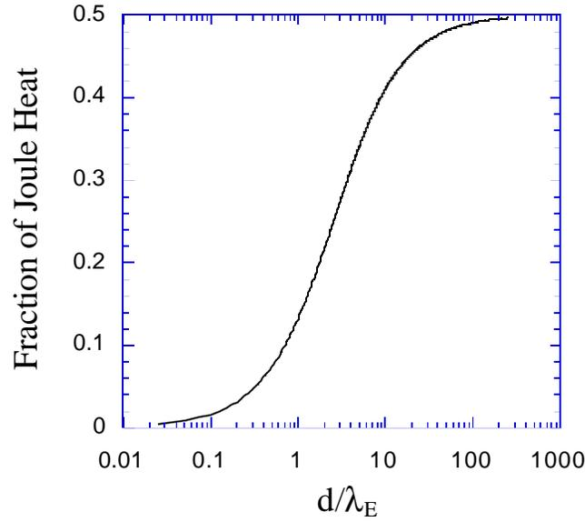
**Figure 2.5** Fraction of the Joule heating generated in the barrier that arrives to the cathode versus the barrier thickness ( $d$ ) normalized by the relaxation length for carriers ( $\lambda_E$ ). The anode side of the barrier is assumed to be in contact with an ideal heat sink.
