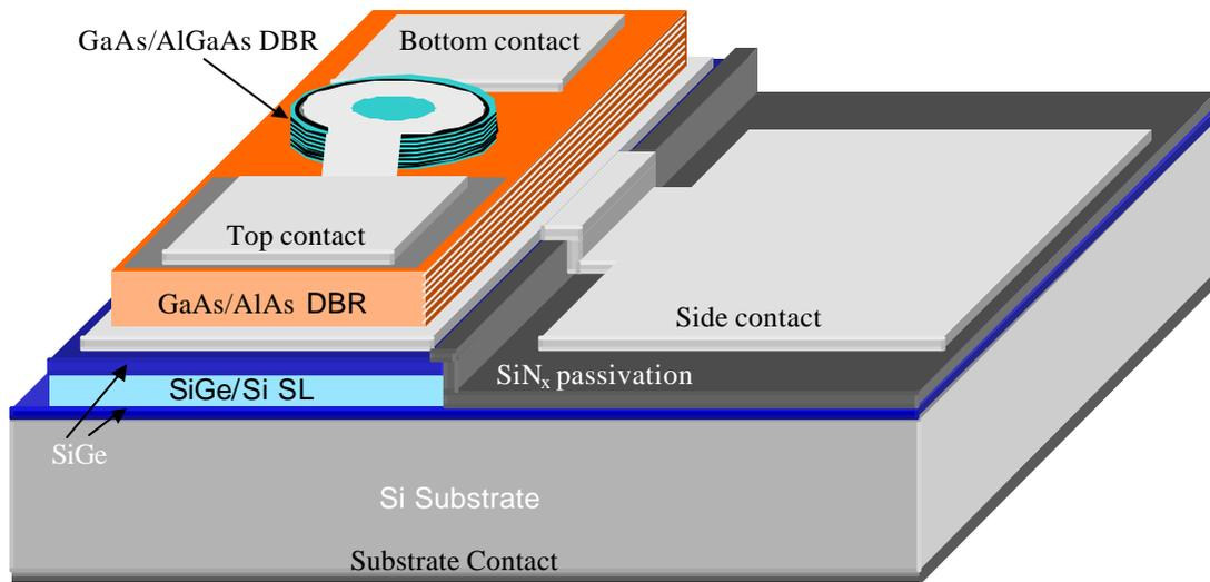
**Figure 7.22** Proposed structure for heterogeneous integration of VCSELs and SiGe/Si superlattice coolers by Au-Au bonding. The laser bias can be applied between the top and side contact, or be made intracavity with two different etch steps. The cooler bias is applied between the side and substrate contacts.
