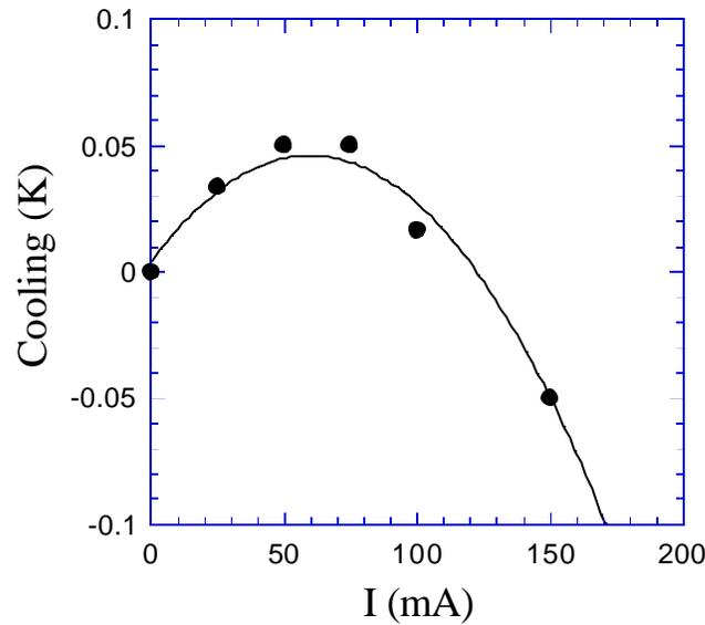
**Figure 6.5** One of the first experimental results demonstrating cooling. The thermionic cooler structure consisted of a simple  $1\ \mu\text{m}$  thick  $n$ -type InGaAsP-barrier ( $1 \times 10^{17}\text{cm}^{-3}$ ) between InGaAs emitter and collector regions ( $2.8 \times 10^{18}\text{cm}^{-3}$ ). The device area was  $3200\ \mu\text{m}^2$ . Small cooling in this early device was limited by the packaging and contact resistance.
