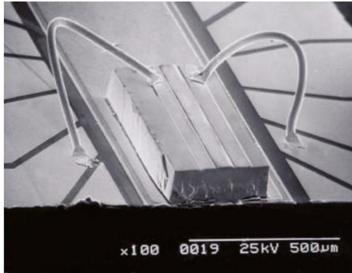
**Figure 7.10** SEM of a processed and packaged ridge laser and monolithically integrated cooler. The laser was mounted at the edge of a cleaved Si package to allow for coupling to a fiber probe. The wire bond for the center stripe  $p$ -contact is not shown.
