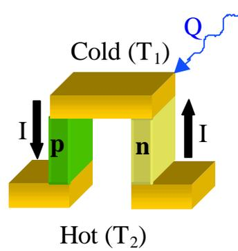
**Figure A.2** Single element of a cooler in a conventional thermoelectric configuration, with  $n$ - and  $p$ -type thermoelements electrically in series and thermally in parallel.
