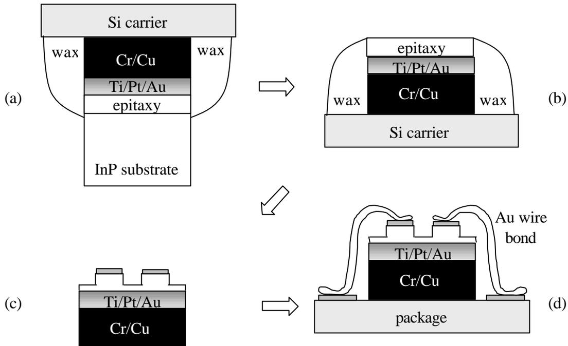
**Figure 5.14** Thin Cu-substrate transfer process. The steps are (a) E-beam evaporate ohmic metal, copper substrate, and solder layers, and mount epi side down to a silicon carrier with wax. (b) Remove InP substrate with a wet etch and (c) deposit top metal to etch mesas. Dice samples and remove the wax. (d) Package and wire bond devices. (Sn soldering layer not shown)
