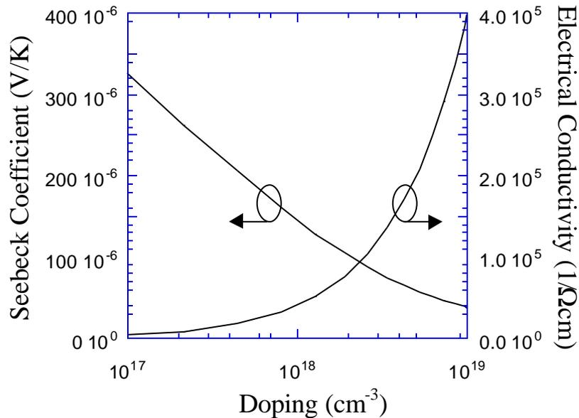
**Figure 2.2** Calculation of Seebeck coefficient ( $S$ ) and electrical conductivity ( $\sigma$ ) as a function of doping for InGaAs bulk material. The substantial decrease in  $S$  at high dopings and  $\sigma$  at low dopings is the cause of low power factor and thus poor  $ZT$ .
