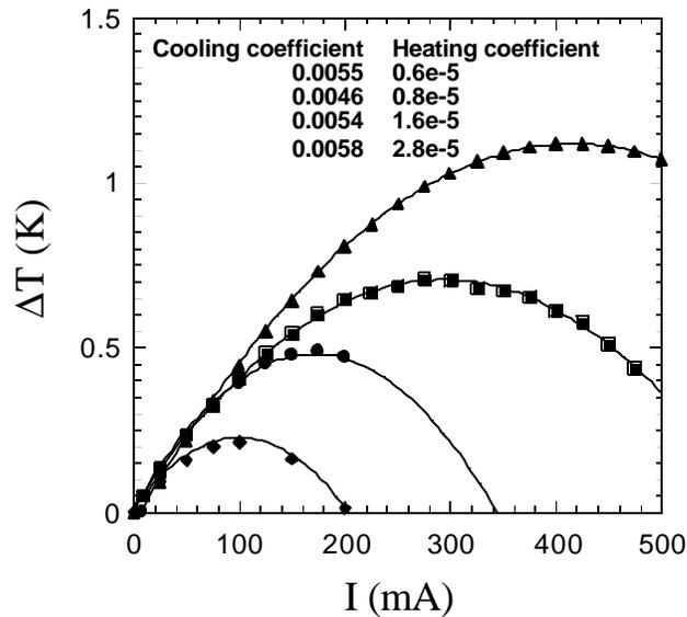
**Figure 6.11** Measured cooling for a 1  $\mu\text{m}$  InGaAs/InGaAsP thermionic cooler with various packages. The cooling (linear) and heating (quadratic) coefficients correspond to a second order polynomial fit. The cooling coefficients remain nearly constant while the heating coefficients are reduced. All temperatures are relative to the value at zero current with a heat sink temperature of 20  $^{\circ}\text{C}$ .
