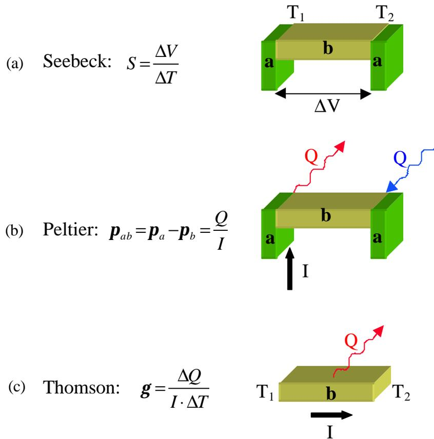
**Figure A.1** Physical description of thermoelectric phenomenon of interest, (a) Seebeck effect, (b) Peltier effect, and (c) Thomson effect.
