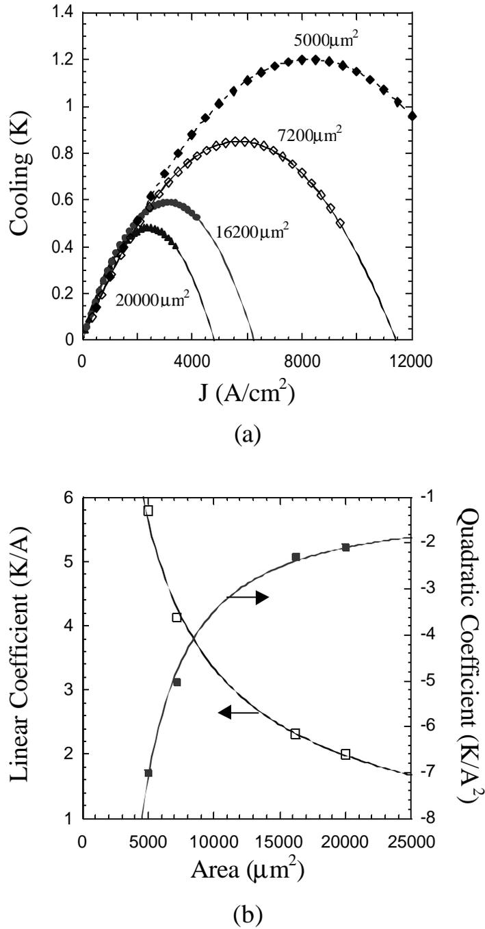
**Figure 6.7** (a) Cooling versus current density for several device sizes and (b) the corresponding linear (cooling) and quadratic (heating) coefficients from a second order polynomial fit as in Equation 6.1. The points are the experimental values, and the curves are simulated from Equation 6.1. Measurements were performed with a heat sink temperature of 300K.
