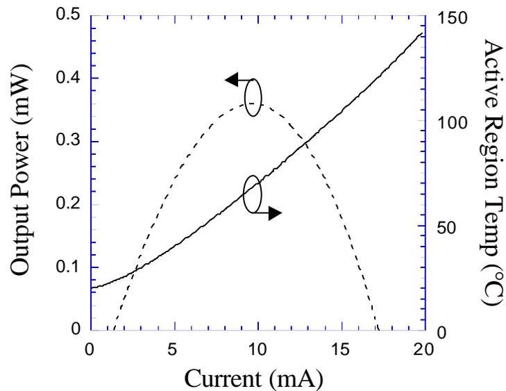
**Figure 7.17** Active region temperature versus current plotted alongside output power for a heat sink temperature of 20 °C. From A. Karim.
