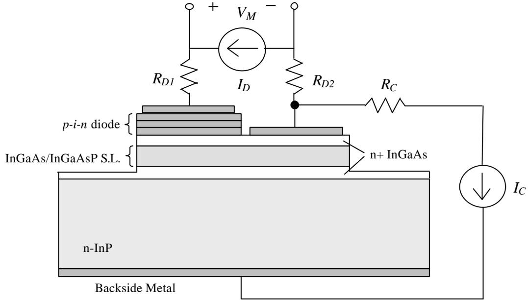
**Figure 7.5** Set-up for measuring the temperature of the integrated diode versus the current through the cooler ( $I_C$ ) and the diode ( $I_D$ ).  $R_{D1}$ ,  $R_{D2}$ , and  $R_C$  are the wire bond resistances.
