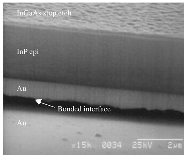
**Figure 7.23** SEM of a Au-Au bonded test structure. While the quality of the bond is difficult to see visually, the mesas remained attached after violent agitation with solvents.
