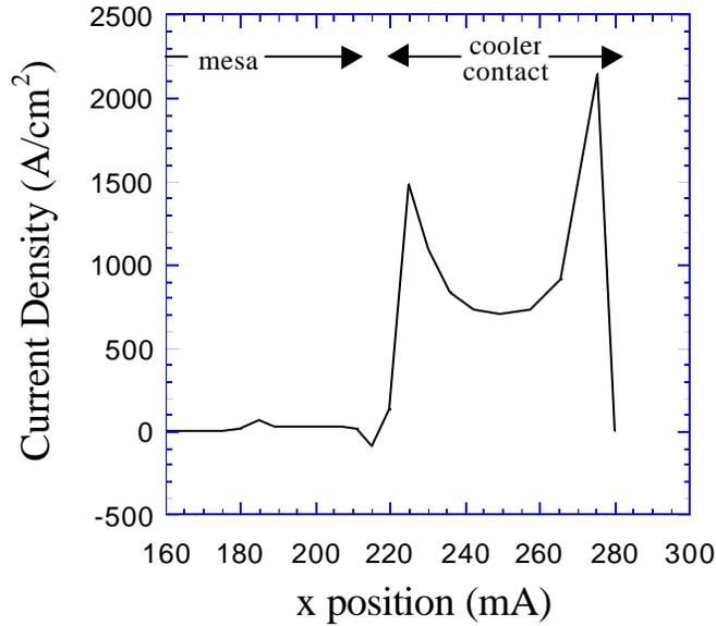
**Figure 7.13** Simulation of current density perpendicular to the cooler at the interface of the InGaAs and cooler superlattice regions. The current does not spread to cool underneath the laser mesa. Simulation by D. Oberle.
