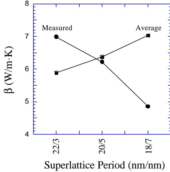
**Figure 4.2** Thermal conductivity versus the ratio of InGaAs/InP for a constant superlattice period. The circles are experimentally measured values while the squares were calculated geometrical averages from experimental bulk values of the constituent materials. Opposite trends are observed even though the same number of interfaces are present. Experimental values from S. Huxtable.
