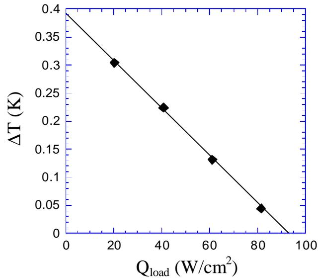
**Figure 7.7** Cooling versus applied heat load density from the integrated photodiode. The points are experimental data while the linear curve fit corresponds to Equation 7.3.
