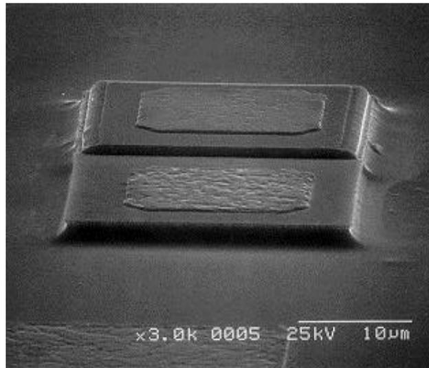
**Figure 7.4** SEM of a processed device showing the monolithically integrated  $p$ - $i$ - $n$  photodiode on top of the  $1\text{-}\mu\text{m}$ -thick InGaAs/InGaAsP thermionic cooler.
