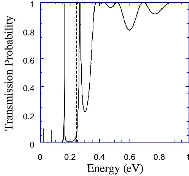
**Figure 2.10** Quantum mechanical transmission probability versus energy for two periods of 7nm/18nm InP/InGaAs superlattice. The dashed line indicates the barrier height of 0.24 eV where the zero on the energy scale corresponds to the minimum conduction band energy in the InGaAs emitter region.
