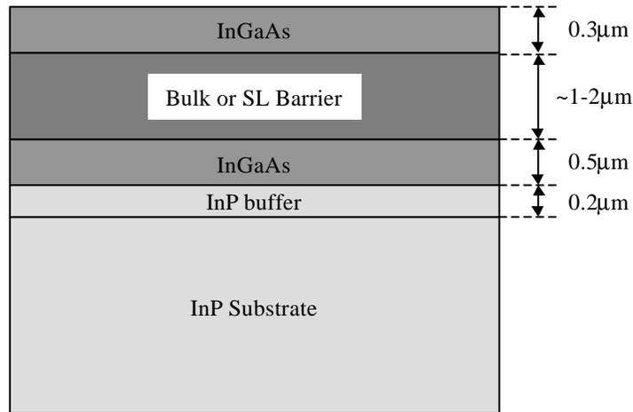
**Figure 3.2** A generic cooler structure consists of the bulk or superlattice barrier sandwiched between two InGaAs emitter and collector regions all grown lattice matched to an InP substrate. Typical layer thickness is indicated.
