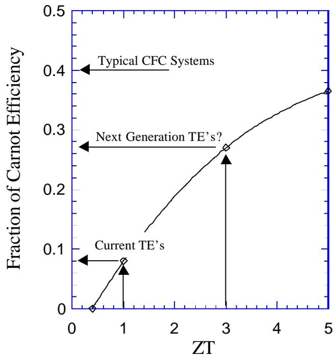
**Figure 1.4** Fraction of Carnot efficiency versus the  $ZT$  of thermoelectrics.  $ZT$ 's greater than 3 will be required to begin competing with conventional CFC cooling systems.
