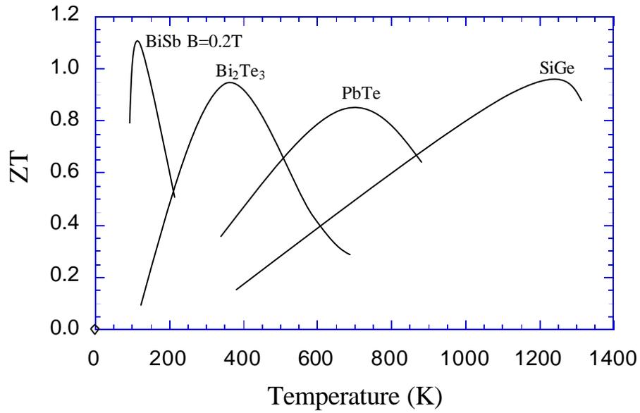
**Figure 1.3**  $ZT$ 's of various thermoelectric materials versus temperature.
