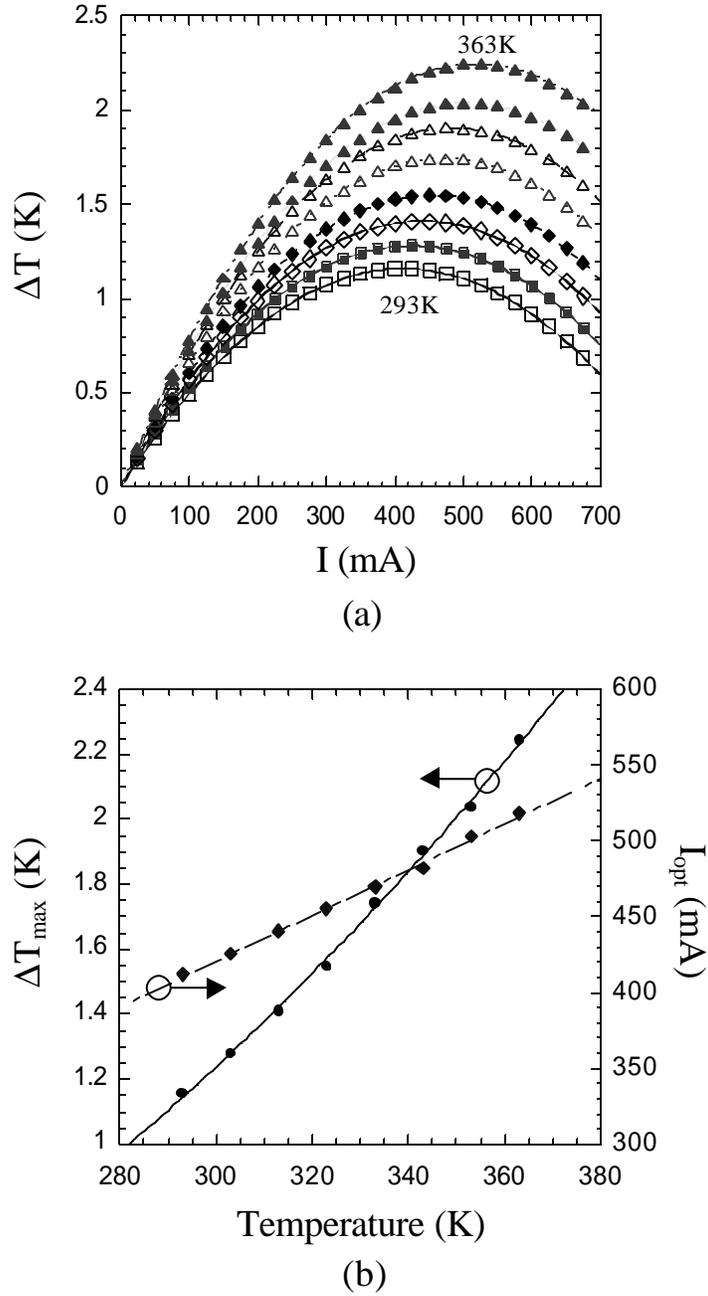
**Figure 6.9** (a) Cooling versus current bias for heat sink temperatures of 293-363K in 10K increments. (b) Corresponding maximum cooling (solid) and optimum current (dashed) versus heat sink temperature. The points are the experimental values and the curves are the theoretical curve fits,  $\Delta T_{\max} \propto T^{1.4} + T^{2.4} + T^{3.4}$ ,  $I_{\text{opt}} \propto T$ .  $\Delta T$  is measured with respect to the heat sink temperature.
