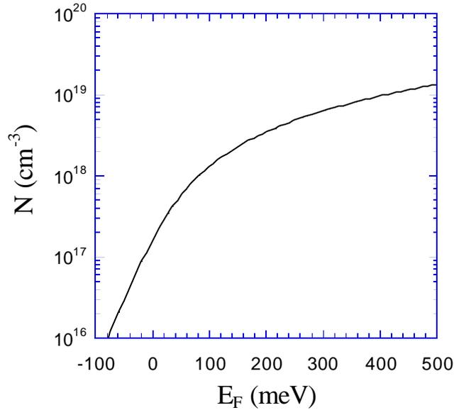
**Figure 2.8** Calculated doping concentration versus Fermi level for InGaAs emitter region. The zero energy references the conduction band minimum.
