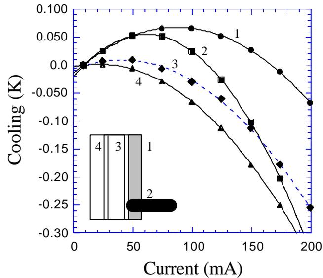
**Figure 7.14** Cooling versus cooler current at different points on the laser and cooler. Only small amounts of cooling are seen on the side contact (1&2), and nearly zero cooling on the laser mesa (3). Measurements were taken with the  $\mu$ -thermocouple system.
