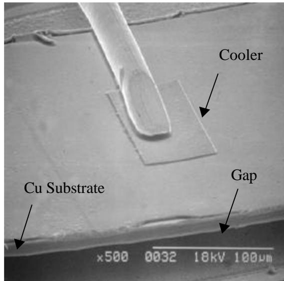
**Figure 5.15** SEM of a packaged thin-film thermionic cooler on a 10- $\mu\text{m}$ -thick copper substrate. It is clear from the photo that there are large gaps that the solder did not spread to during packaging.
