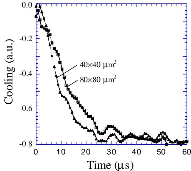
**Figure 7.2** Transient response of two different sized SiGe thin film coolers as a function of time. The response time is on the order of 15-25  $\mu\text{s}$ . Measured by A. Fitting.
