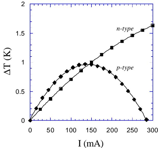
**Figure 6.16** Measured cooling versus current bias for a *p*-type ( $100 \times 100 \mu\text{m}^2$ ) and *n*-type cooler ( $50 \times 100 \mu\text{m}^2$ ) at a heat sink temperature of  $70^\circ\text{C}$ .
