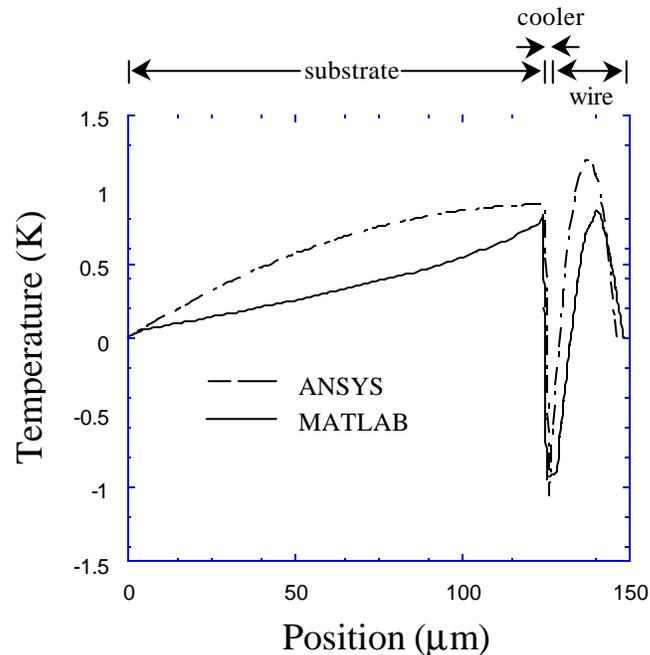
**Figure 6.23** Comparison of simulated temperature profiles through the substrate, cooler, and wire bond for the three-dimensional (ANSYS) and one-dimensional (MATLAB) models. The zero temperature axis is relative to 300 K.
