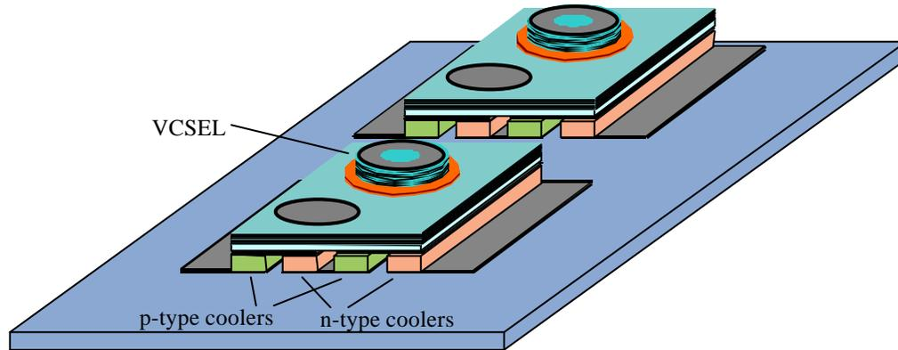
**Figure 8.1** Example of *n*- and *p*-type cooler integration for small scale cooling of individual VCSELs
