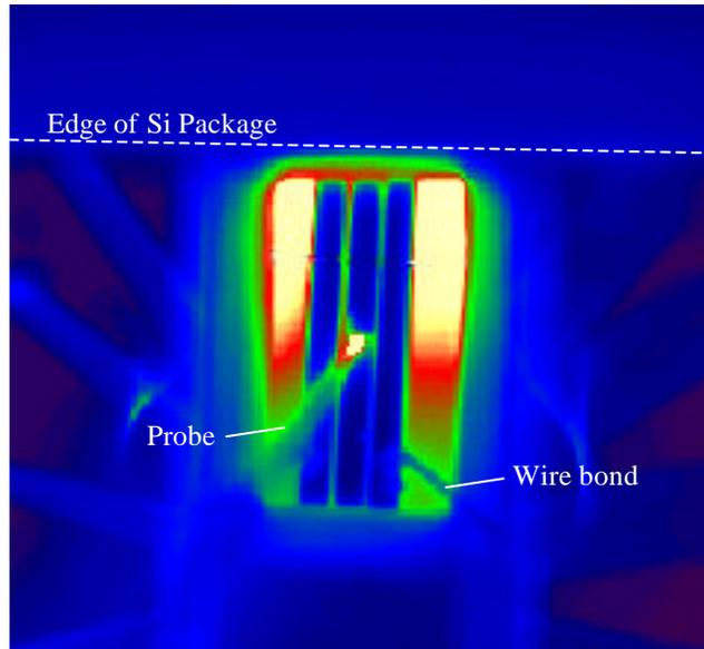
**Figure 7.15** Thermal image of a packaged laser with integrated cooler. The blue regions on the device are the metal contacts and the other regions InP. Larger color changes are seen in the InP due to the larger emissivity constant. Less thermal spreading at the edge of the Si package causes increased heating on one side of the laser chip. The IR-camera measurement system was described in Chapter 6.
