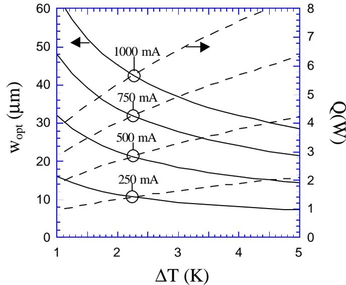
**Figure 5.8** Optimum contact width (solid lines) and corresponding cooling power loss (dashed lines) versus bias currents and temperature differences for integrated side contact geometry.
