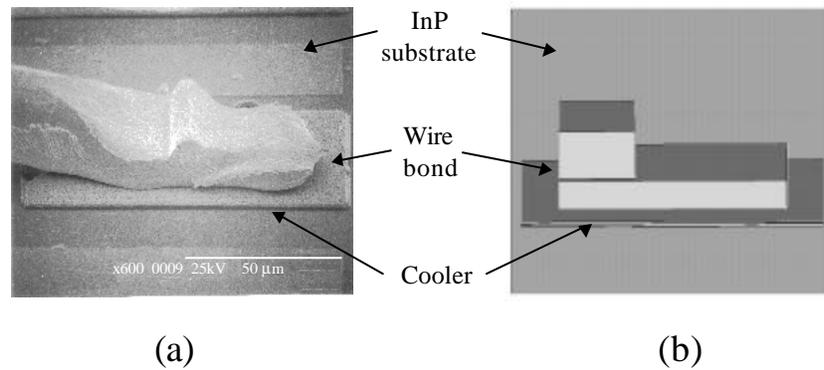
**Figure 6.18** (a) Scanning electron micrograph of a thin-film thermionic cooler and (b) the simulated structure. The cooler mesa is 1.4 μm high, and the uppermost wire bond length is scaled to reduce the element count in the mesh.
