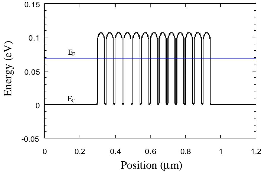
**Figure 3.3** Simulated conduction band diagram and Fermi level at equilibrium for a 10nm/40nm InGaAs/InGaAsP ( $\lambda_{\text{gap}}=1.3\mu\text{m}$ ) superlattice barrier with InGaAs emitter and collector regions. The InGaAs regions are doped to  $3 \times 10^{18} \text{ cm}^{-3}$  and the InGaAsP regions are undoped. All compositions are lattice matched to InP.
