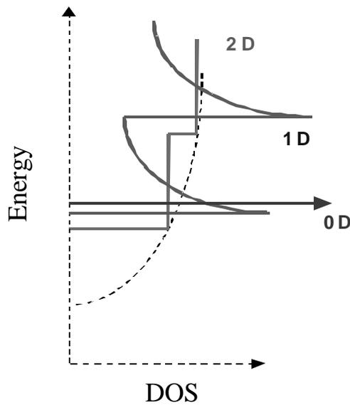
**Figure 1.5** The electronic density of states (DOS) versus energy for various dimensionalities (3D, 2D, 1D, and 0D). The first two quantified states are plotted.
