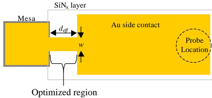
**Figure 5.7** Top view of the side contact geometry. The optimized region is the area close to the device mesa where Joule heating and heat conduction are most important.
