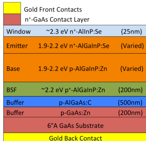
Fig. 2. Schematic showing the structure of the epitaxially grown layers and metallization of the AlGaInP solar cells studied in this paper. The diagram is not to scale.
