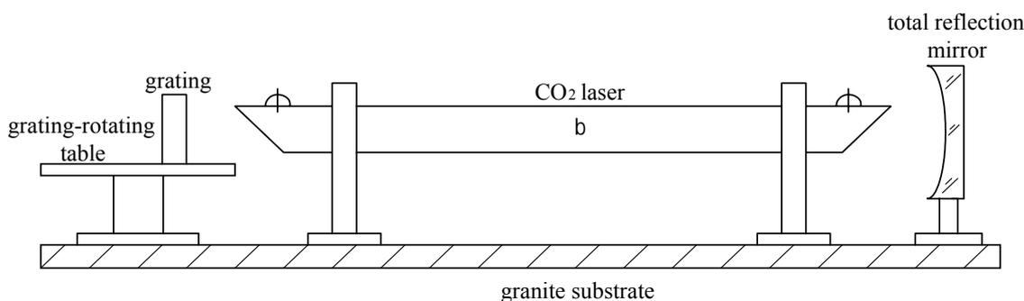
Fig.1 the cavity configuration of the CO<sub>2</sub> laser with a completely external cavity
