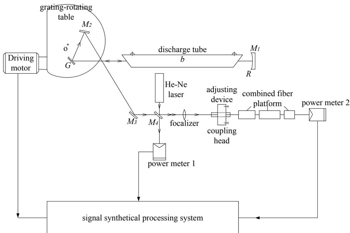
Fig.2 testing system for the transmission characteristics of the infrared fiber
