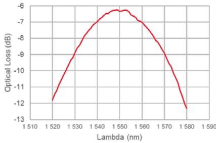
Fig. 6. Fiber-to-fiber optical transmission loss through two grating couplers.
