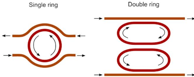
Fig. 10. Single and double micro-ring geometries.
