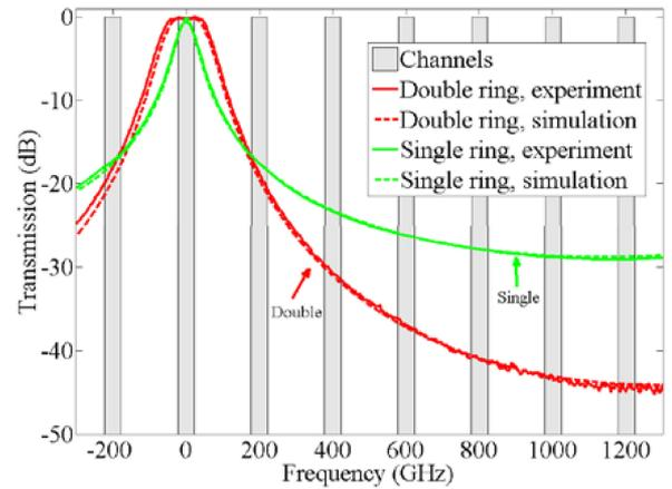
Fig. 11. Transmission response of single (red) and double micro-rings (green). Solid lines represent the experiment, and dashed lines, the simulation. The 200 GHz-spaced channel positions are indicated with grey rectangles. Zero frequency corresponds to approximately 1552 nm.
