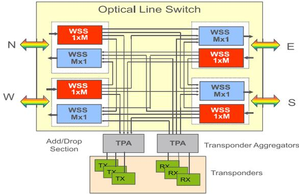
Fig. 1. Colorless-directionless and contentionless ROADM.
