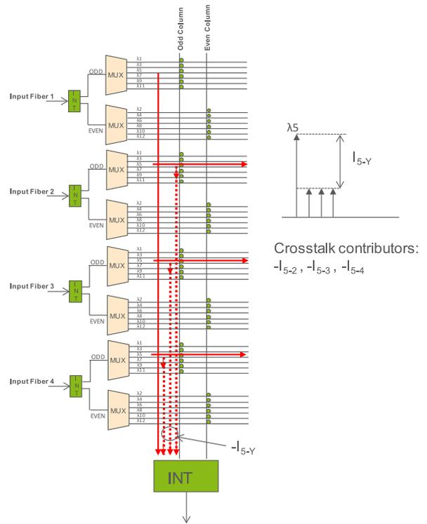
Fig. 5. Interferometric crosstalk components in the drop TPA.
