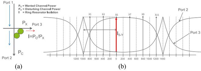
Fig. 4. (a) Crosstalk in MRR set in OFF. (b) Position of MRR in OFF for both add and drop TPA.
