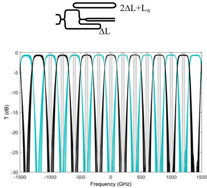
Fig. 7. Schematic of the interleaver design and simulated yield analysis with fabrication deviations (considering both heaters in optimum conditions for each case). Bar and cross spectra are shown in black and blue respectively. Channel positions are indicated with gray rectangles, channel spacing is 200 GHz and central frequency is set to 193.1 THz (1552 nm).
