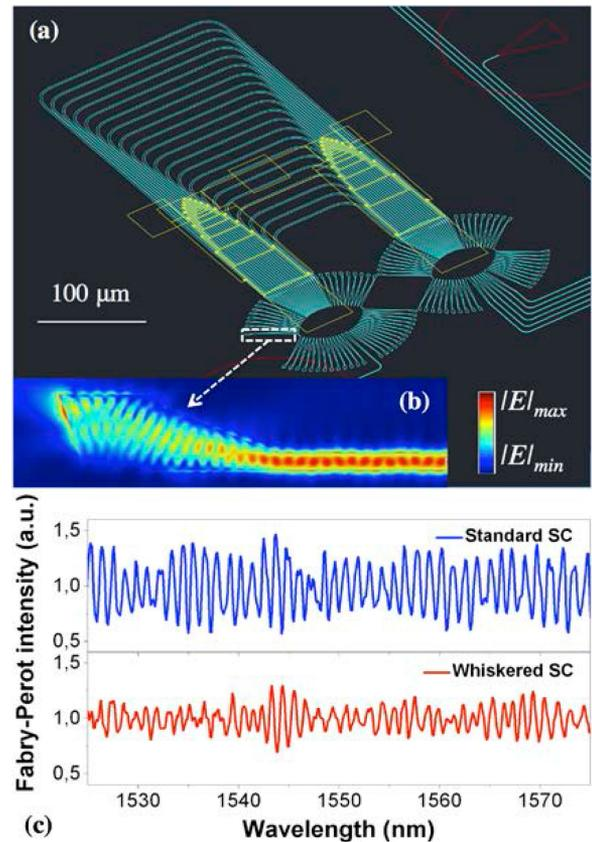
Fig. 8. (a) AWG layout realized for the IRIS full matrix. Different colors represent different design layers: in cyan the silicon waveguides, in yellow the Ti/TiN heaters, the micro-pillars and the electrical pads, in red the grating couplers. (b) FEM simulation of the electric field profile propagating through a reflection killer. Back-reflections are about 18 dB. (c) Fabry-Perot oscillations that rise in an AWG with a standard SC, upper plot, and with a whiskered SC, lower plot.
