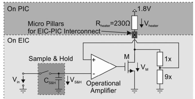
Fig. 14. Block diagram of one heater control circuit
