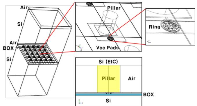
Fig. 18. Layout of thermal simulation including  $5 \times 5$  ring switches connected to EIC for thermal control through Cu pillars.
