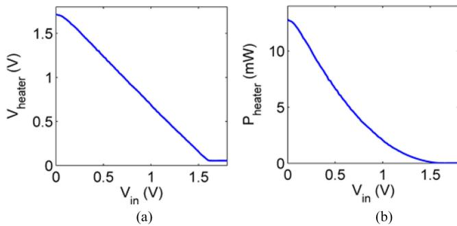
Fig. 16. Heater voltage (a) and heater power (b) depending on the input voltage of the S&amp;H element.
