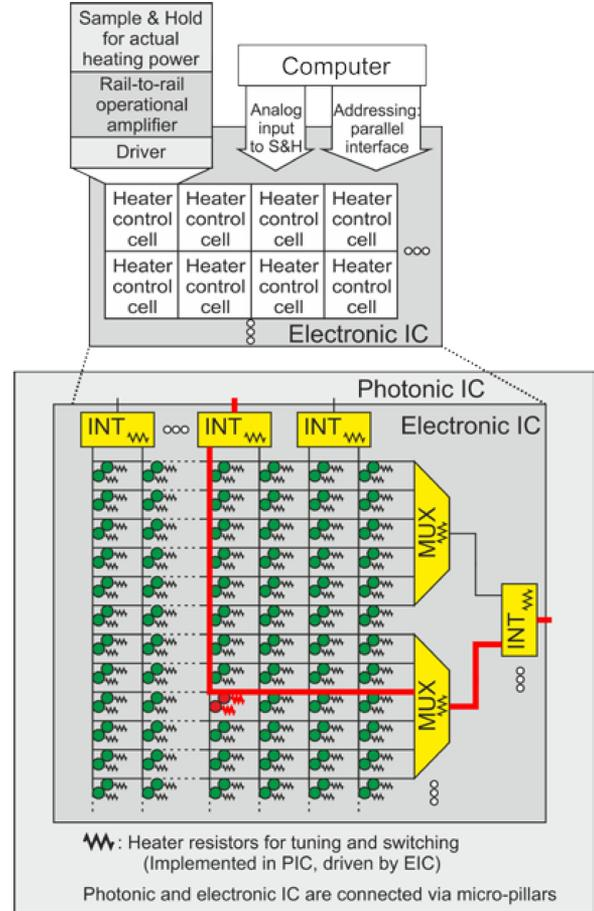
Fig. 13. Control of the heater resistors in the PIC by the EIC.
