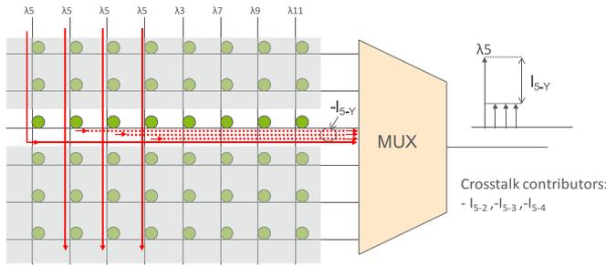
Fig. 3. Interferometric crosstalk components in the add TPA.
