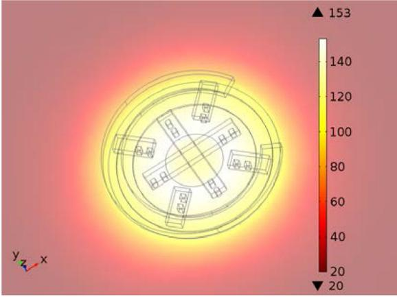
Fig. 12. Simulation of a single micro-ring integrated heater. Temperature variation ( $^{\circ}\text{C}$ ) for  $V = 0.9\text{ V}$ .
