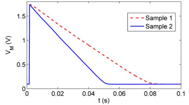
Fig. 17. S&amp;H voltage drop for two different S&amp;H elements over time caused by leakage.
