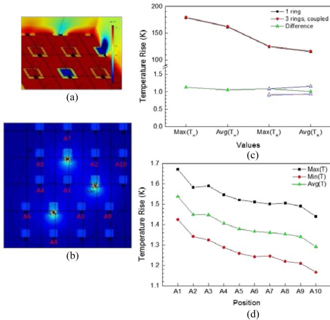
Fig. 19. Results of thermal simulation: (a) voltage distribution, (b) temperature distribution, (c) temperature rise of three heated micro-rings, and (d) temperature rise of neighboring micro-rings.
