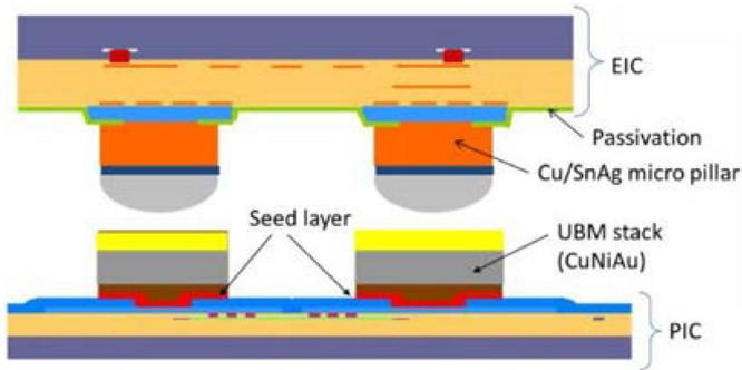
Fig. 21. Cross section of PIC and EIC dies with UBM stack and micro pillars.
