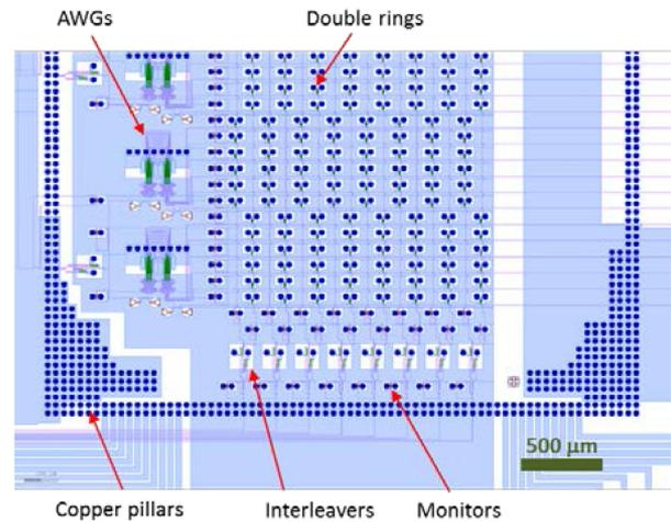
Fig. 20. Mask layout showing the bottom part of the matrix with double-ring switches.
