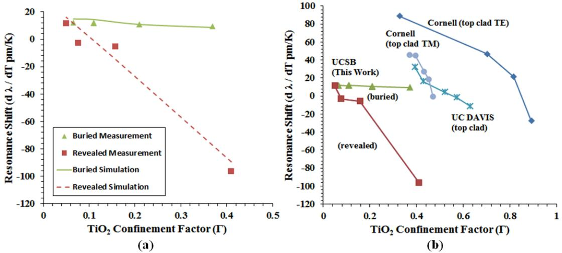
**Figure 2.5:** (a) Measured thermal drift with *confinement models* based on Eq. 2.9 with separately fitted TiO<sub>2</sub> TOC for buried ( $-10^{-6}K^{-1}$ ) and revealed ( $-2.5 \times 10^{-4}K^{-1}$ ) rings. (b) Measurements compared to other literature with TiO<sub>2</sub> cladding demonstrate a unique suppression of TOC in buried TiO<sub>2</sub>.
