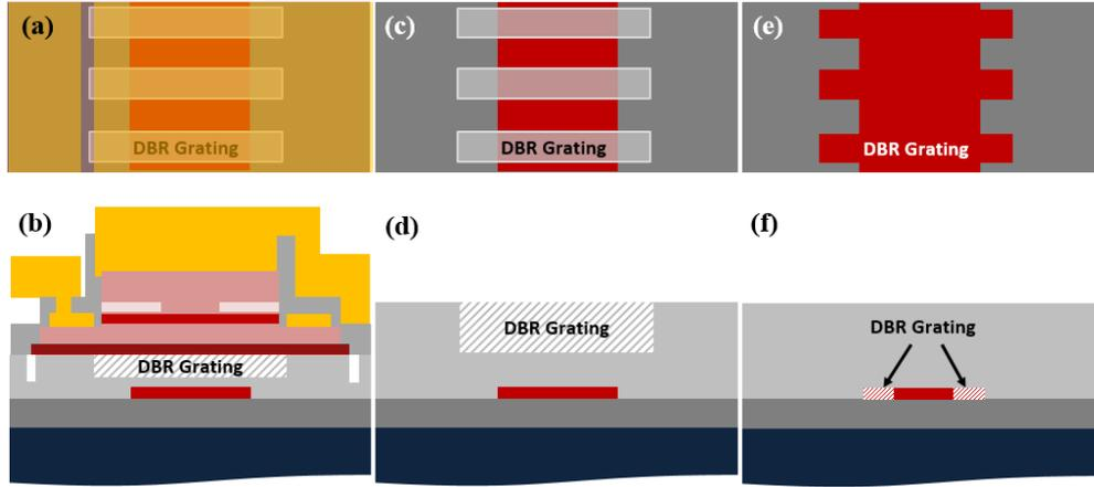
**Figure 3.11:** (a-b) Top and cross-section of surface corrugated gratings underneath bonded III-V lasers (c-d) Top and cross-section of surface corrugated gratings into top cladding of passive waveguide. (e-f) Top and cross-section of sidewall passive gratings.
