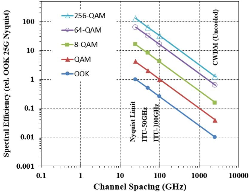
**Figure 2.1:** This plot compares two methods of improving spectral efficiency in a transmission link. Assuming the link is uncooled you are limited to coarse WDM (20 nm) spacing if you can not thermally stabilize your channels. If you can make a link with athermal components you gain a factor of 100 that makes on-off-keying comparable to the highest order modulation schemes.
