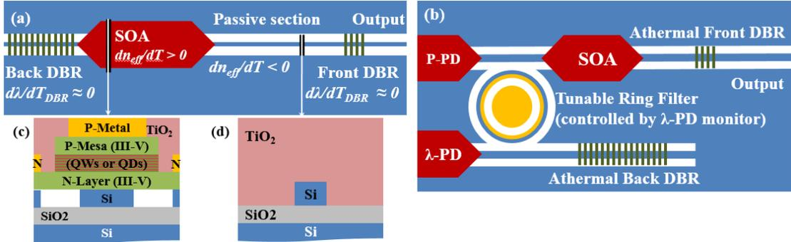
**Figure 2.13:** (a) Passively Athermal DBR Laser (b) Athermal Ring Filtered DBR (ARF-DBR) Laser (c) cross section of III-V/Si Hybrid SOA or PD with  $\text{TiO}_2$  cladding. (d) cross section of Si waveguide clad with  $\text{TiO}_2$  for a thermal compensator.
