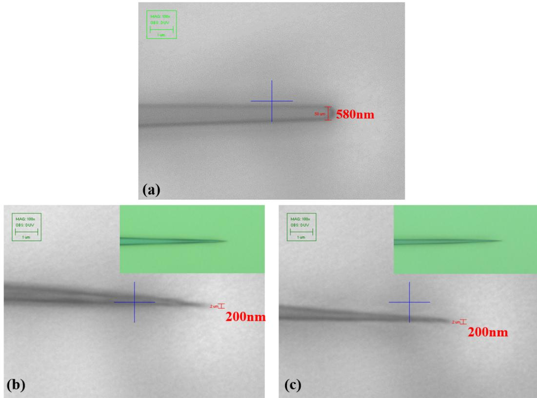
**Figure 4.18:** (a) Initial taper tip width from SPR955-0.9. (b-c) CUV microscope images of the split in final tapered PMGI patterns post-process. (b) 6x2min exposure, 3x60s develop (c) 3x4min exposure, 3x60s develop. Figure insets are visible microscope images.
