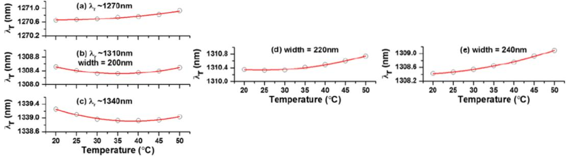
**Figure 2.11:** Measured (black circle) and quadratically fitted (red line) resonance wavelength as a function of temperature. The device with a waveguide width of 200 nm is measured at various spectral ranges around (a) 1270 nm, (b) 1310 nm and (c) 1340 nm and across different waveguide widths (b) 200 nm, (d) 220 nm, (e) 240 nm [74].
