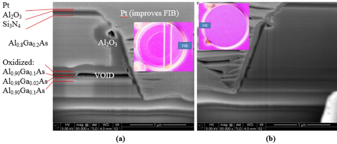
**Figure 4.13:** Comparison of FIB cross sections in adjacent mesas labeled in Fig. 4.12 and placed in the inset of each SEM image. (a) Shows oxidized area of protected feature of mesa and a 1  $\mu\text{m}$  void at the oxidation layer. (b) Shows an entirely protected mesa with no signs of oxidation at all and no void.
