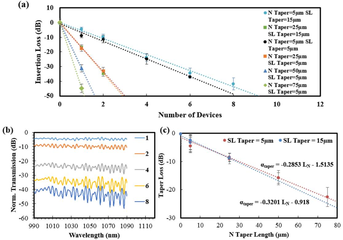
**Figure 3.10:** (a) Measured insertion loss for repeated passive III-V to Si<sub>3</sub>N<sub>4</sub> tapers plotted by number of serial repeats of a single device. (b) Normalized transmission spectra for (1, 2, 4, 6 & 8) repeats of lowest loss taper. (c) Taper loss is plotted from the repeated taper data in (a) after removing bulk loss.
