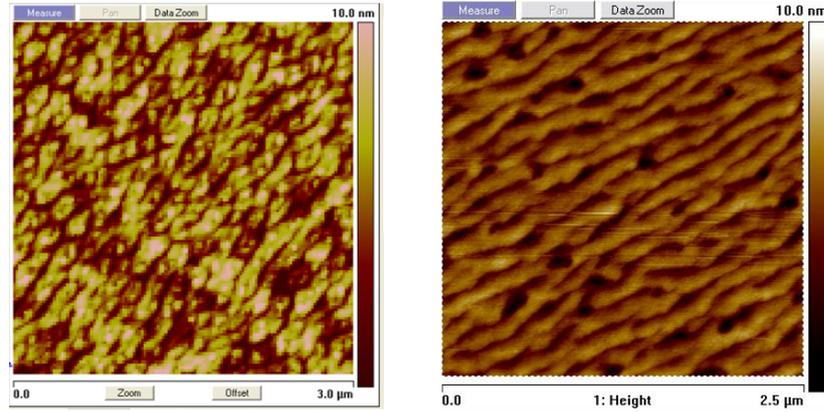
**Figure 4.3:** AFM scans of SL surface before bonding; (a) initial growth with InGaP SL (2.8 nm RMS) resulted in unsuccessful bonding; (b) second growth substituting the InGaP SL with InGaAs/GaAsP (1.1 nm RMS) resulted in successful bonding.
