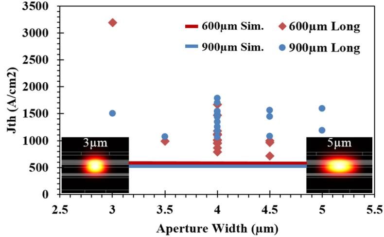
**Figure 3.8:** Threshold current densities of pulsed laser as a function of their aperture width.
