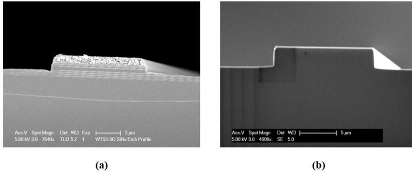
**Figure 4.8:** SEM cross sections of Unaxis ICP AlGaAs etches. (a) Initial house Cl<sub>2</sub>/N<sub>2</sub> recipe. (b) Developed Cl<sub>2</sub>/N<sub>2</sub>/H<sub>2</sub> recipe.
