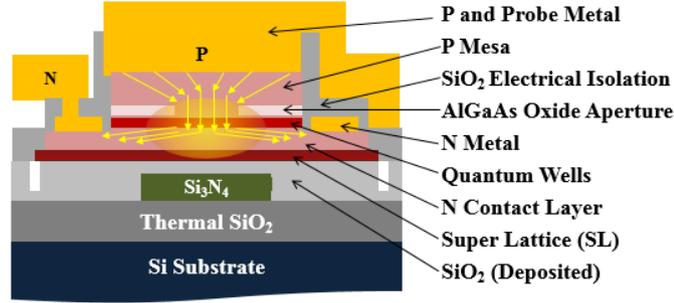
**Figure 3.2:** Laser cross-section. In bulk of the gain region, mode is entirely in III-V so Si<sub>3</sub>N<sub>4</sub> waveguide width reduces to zero over the course of the tapered mode converter and the mode is guided by the AlO<sub>x</sub> aperture
