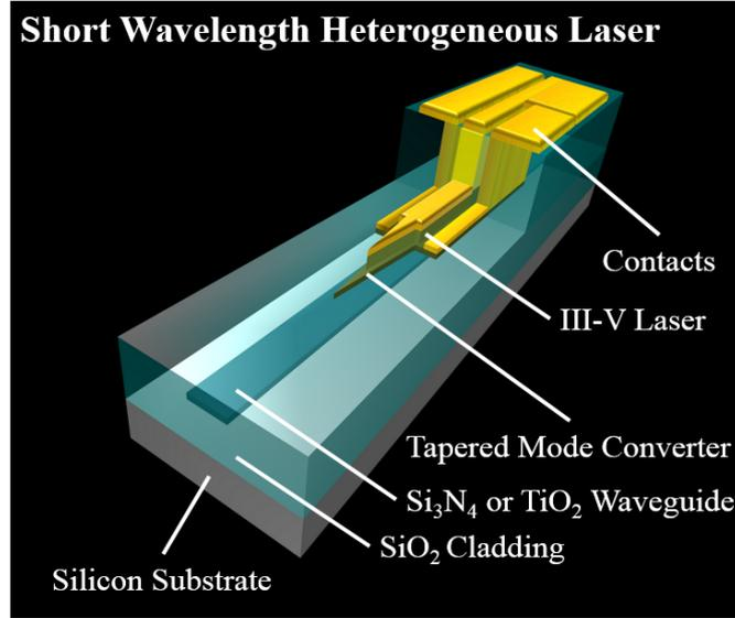
**Figure 1.1:** Schematic of heterogeneous integration of III-V laser with broadband Si<sub>3</sub>N<sub>4</sub> or TiO<sub>2</sub> waveguide. (artwork courtesy of Martijn Heck)
