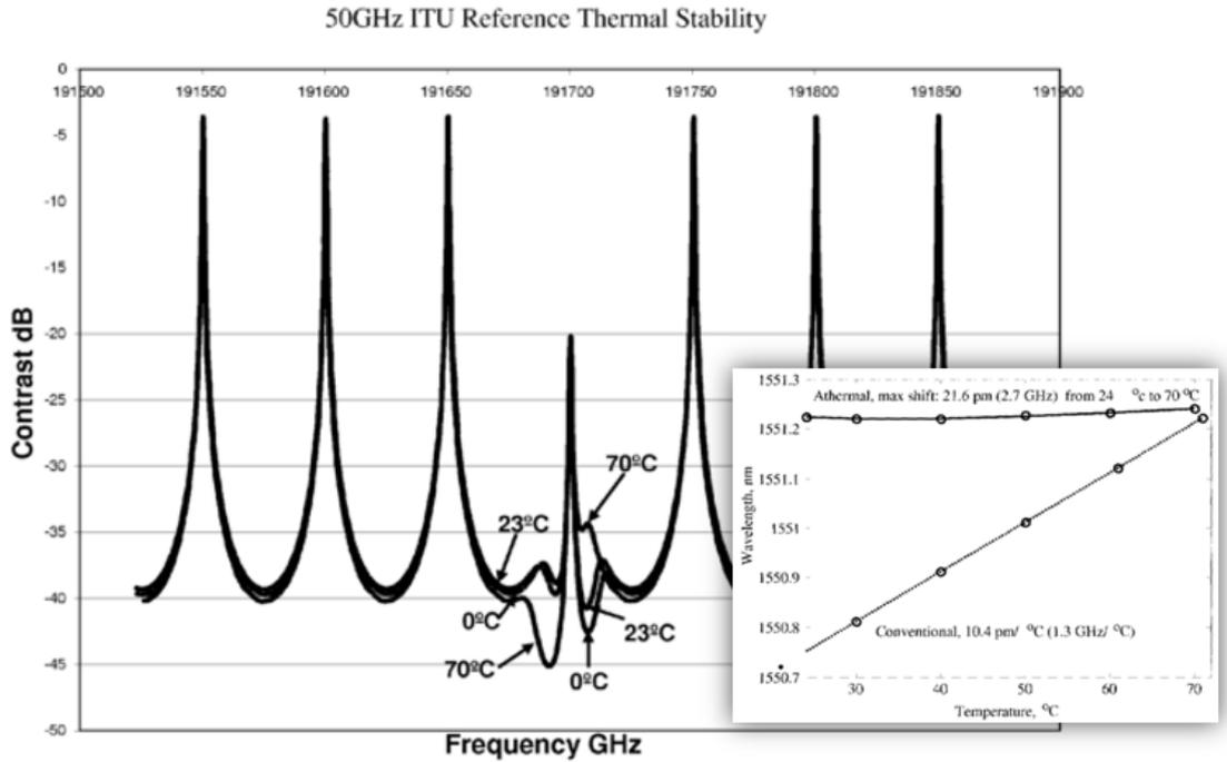
**Figure 1.4:** Spectral response and temperature dependent Bragg wavelength plots for athermally packaged fiber Bragg grating. [10].
