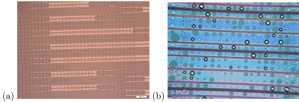
**Figure 4.6:** (a) Microscope image of the original placement of VCs under thin n-contact material. (b) Microscope image following a high-temperature process with a full thin n-layer. Most VCs burst and redeposited material onto the sample.
