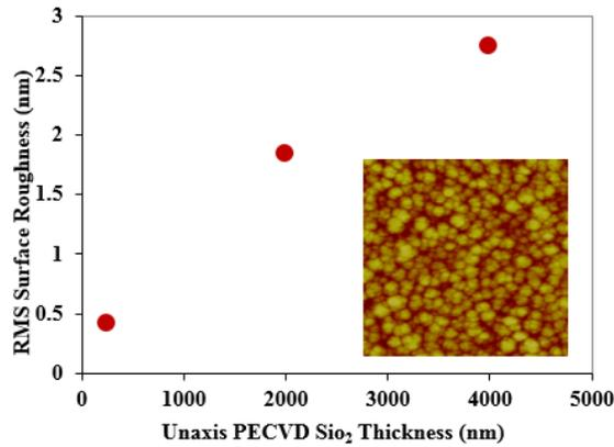
**Figure 4.4:** Roughness from AFM scans of Si with different thicknesses of SiO<sub>2</sub> deposited with the Unaxis PECVD 100°C UCSB standard recipe. Inset shows typical topology of SiO<sub>2</sub> on Si.
