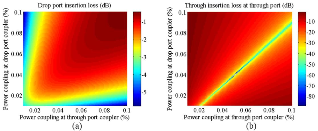
**Figure 2.15:** (a) Drop port insertion loss in dB of a ring filter (i.e. from the SOA to the rear mirror in Fig. 2.13(a)). (b) Through port insertion loss in dB (i.e. from the SOA to the P-PD in Fig 2.13(a)). Assumes 1dB/cm propagation loss, 25  $\mu\text{m}$  ring radius.
