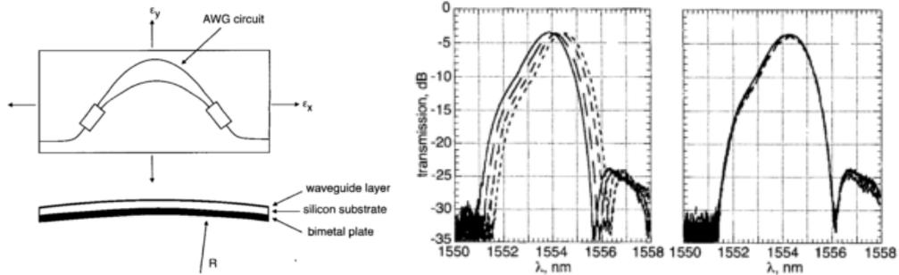
**Figure 1.3:** Schematic configuration of AWG multiplexer with bimetal plate and the corresponding change in temperature dependent spectral response. [9].
