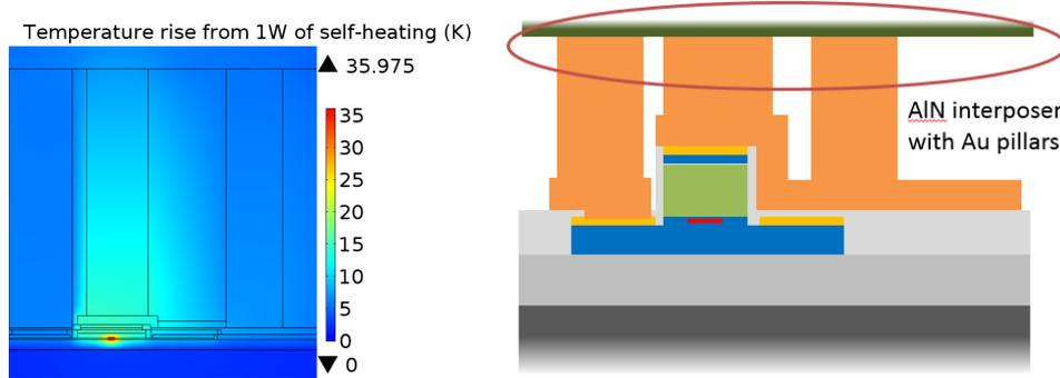
**Figure 3.22:** Thermal simulation showing the release of thermal energy primarily out of the mesa. Mesa is 20  $\mu\text{m}$  wide with 1.520  $\mu\text{m}$  tall mesa and made of  $\text{Al}_{0.8}\text{Ga}_{0.2}\text{As}$ .
