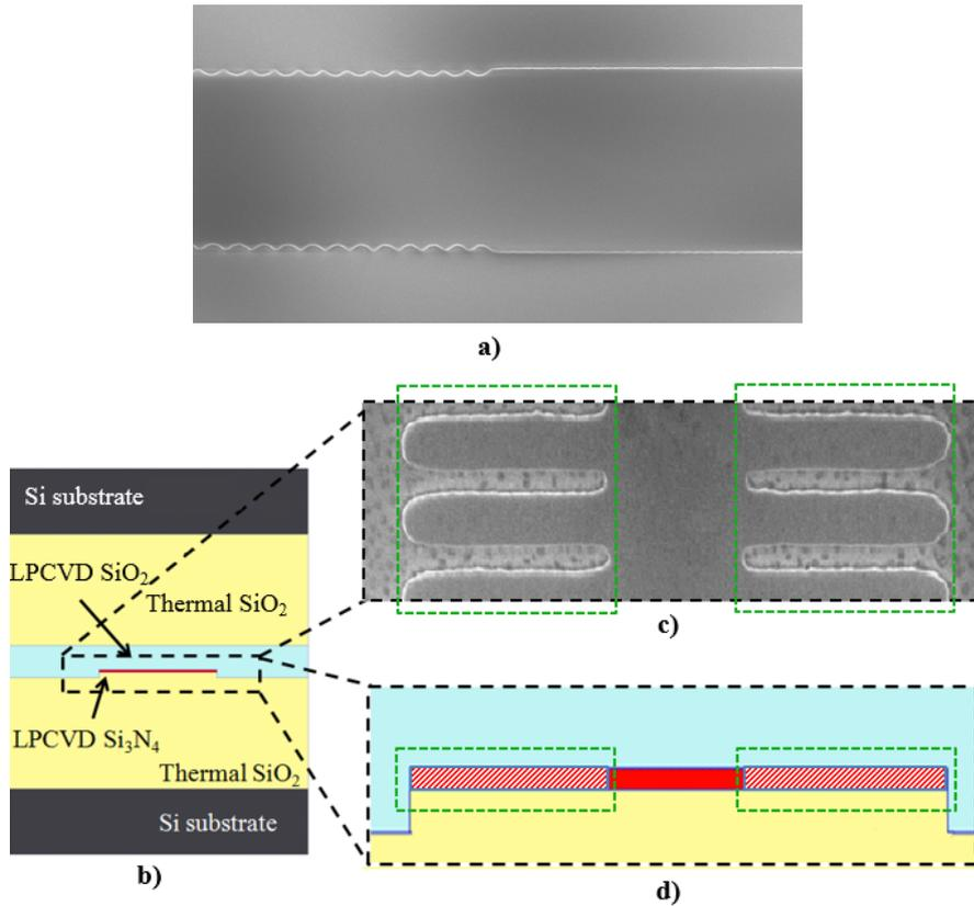
**Figure 3.12:** (a) SEM image of sidewall DBR in LPCVD Si<sub>3</sub>N<sub>4</sub> strip with subtle perturbation. (b) Waveguide cross-section for C-band ultra-low loss waveguide. (c) SEM image of strong perturbation for reference to (d) a zoomed in cross-section with shaded grating areas.
