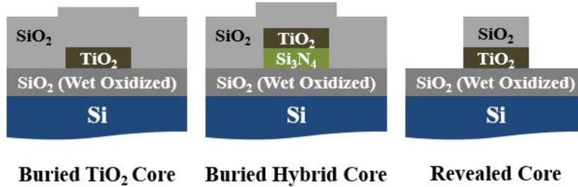
**Figure 2.4:** Cross section of waveguide designs with  $TiO_2$  or hybrid cores.
