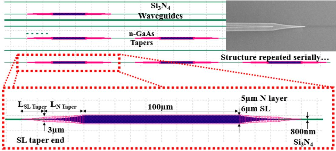
**Figure 3.9:** Layout of repeated taper structures with labels on key geometries. Mask splits included length of SL taper, and length of N Taper. Taper tips  $\sim 200$  nm. Structures do not include active quantum well mesa.
