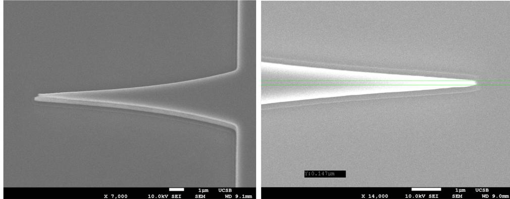
**Figure 4.19:** Characteristic p-mesa tapers following Cl<sub>2</sub>/N<sub>2</sub> dry etch with SiO<sub>2</sub> hardmask and H<sub>2</sub>SO<sub>4</sub>:H<sub>2</sub>O<sub>2</sub>:H<sub>2</sub>O (1:1:10) wet etch. (right) measurement of hard-mask taper tip width is 147 nm.
