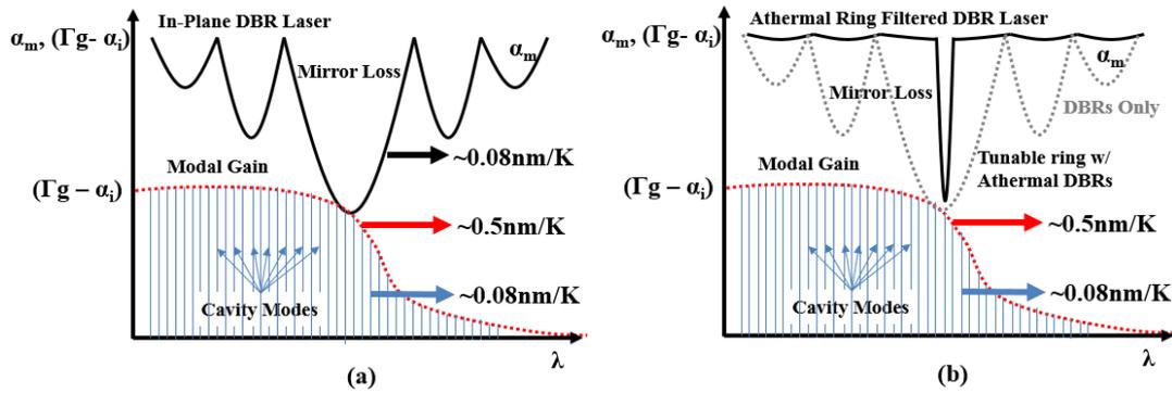
**Figure 2.12:** (a) Diagram of typical in-plane semiconductor laser with dense cavity modes where thermal drift is typically dominated by cavity loss. (b) A similar DBR laser design with an intra-cavity ring filter to achieve a narrower reflectivity bandwidth.
