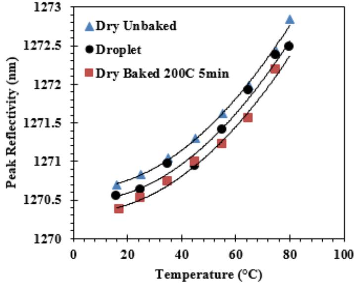
**Figure 2.9:** Peak reflectivity of 200 nm wide, 200 nm height third order DBR gratings as a function of temperature. Sample was tested following cleaning and N<sub>2</sub> drying, first without baking (typical), second with a water droplet on top (high humidity), and finally after a 5 min 200°C dehydration bake (low humidity) [74].
