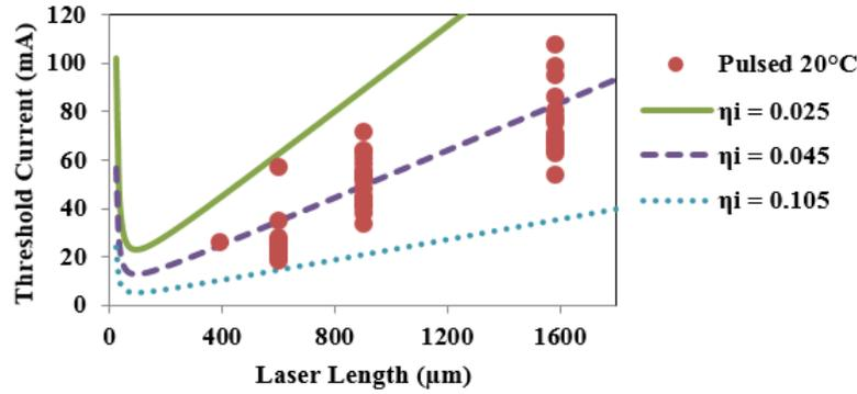
**Figure 3.6:** 20°C pulsed threshold current data for 12  $\mu\text{m}$  mesas with 4  $\mu\text{m}$  wide current apertures 300°C O<sub>2</sub> plasma assisted bonded to 5  $\mu\text{m}$  of SiO<sub>2</sub> on Si.
