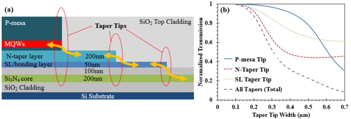
**Figure 4.16:** Analysis of transmission through tips in 3 layer taper from III-V to Si<sub>3</sub>N<sub>4</sub>. (a) Side view of each tip and the simulated layer thicknesses. Indices can be found in Table 3.2. (b) Transmission for each taper and the product of all of them plotted vs. the taper tip width.
