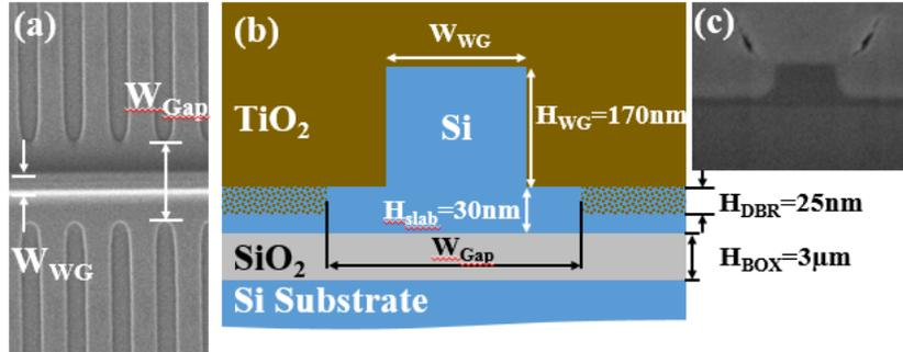
**Figure 2.8:** Waveguide geometries. (a) top down SEM image of DBR before TiO<sub>2</sub> top cladding deposition, (b) cross-sectional diagram of DBR. (c) Cross-sectional SEM of TiO<sub>2</sub> clad Si waveguide with small voids visible in the TiO<sub>2</sub> [74].
