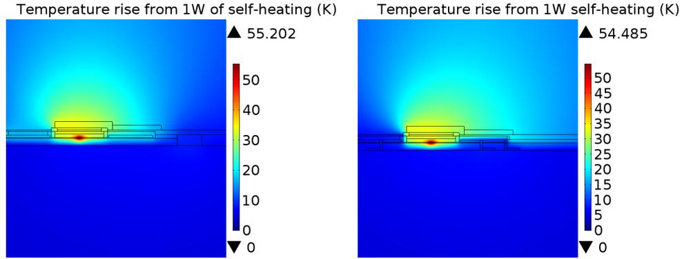
**Figure 3.18:** Comparison of probe and n-metal shunts. N-metal shunts  $1.5 \mu\text{m}$  wide were added  $25 \mu\text{m}$  from the center of the  $20 \mu\text{m}$  mesa. A single  $10 \mu\text{m}$  wide probe shunt is added to the  $2 \mu\text{m}$  thick p-probe and shunted  $40 \mu\text{m}$  from the mesa.
