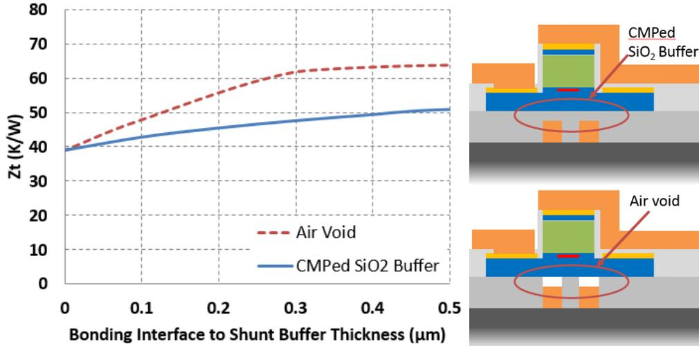
**Figure 3.20:** Two buffers between the shunt and the bonding interface are compared, an air void and CMPed SiO<sub>2</sub>.
