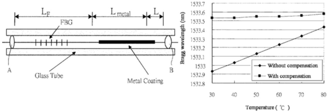
**Figure 1.5:** Schematic and temperature dependent wavelength response of an athermal packaging solution for a fiber Bragg grating [11].
