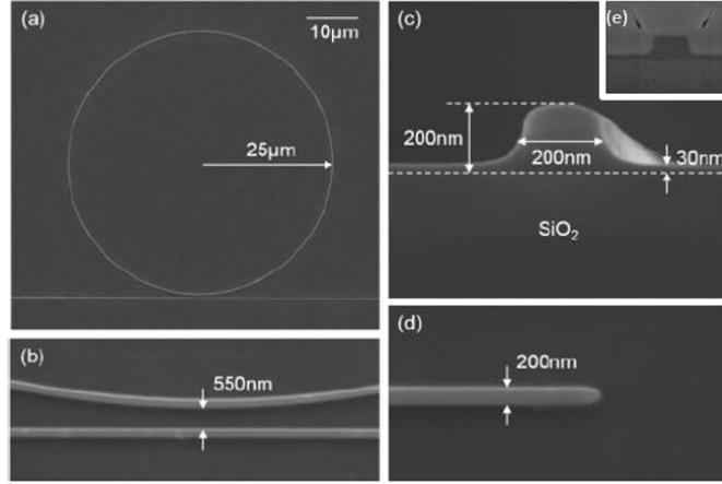
**Figure 2.10:** (a) Top-view SEM image of ring resonator before TiO<sub>2</sub> cladding deposition; (b) Ring-to-bus waveguide coupling region; (c) Cross-sectional SEM image of waveguide before TiO<sub>2</sub> cladding deposition; (d) Top-view SEM image of inverse taper. (e) Shows the waveguide following TiO<sub>2</sub> cladding with small voids in the deposited film [74].
