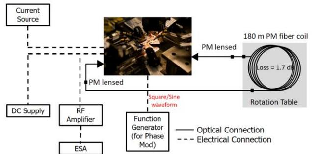
Figure 4: Gyroscope measurement setup
