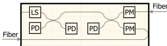
Figure 1: Schematic of the chip layout. LS: Light Source, PD: Photodiode, PM: Phase Modulator. Interfaces with single mode/polarization maintaining fibers are realized on two facets of the chip.
