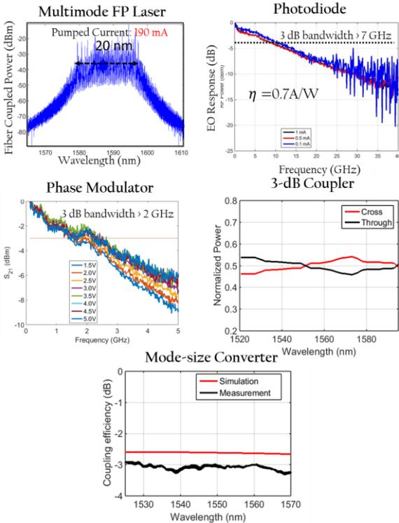
Figure 3: Performances of individual components of the IOD chip. All measurements were carried out at room temperature.
