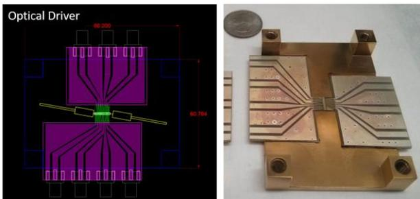
Figure 6: (Left) Schematic of the electrical and optical packaging for the IOD chip (Right) A photograph of the carrier.
