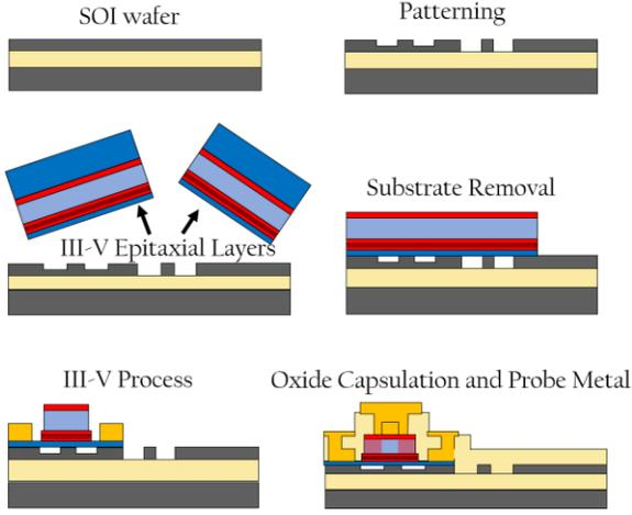
Figure 2: Fabrication process flow for the IOD chip on Si/III-V heterogeneous integration platform (from left to right, up to down).
