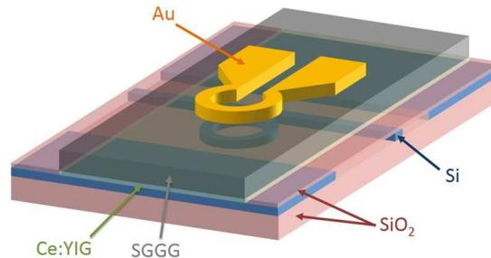
Figure 2: Schematic of the heterogeneous isolator
