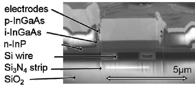
Figure 1: Cross section of a heterogeneous Si<sub>3</sub>N<sub>4</sub>/Si/InP device
