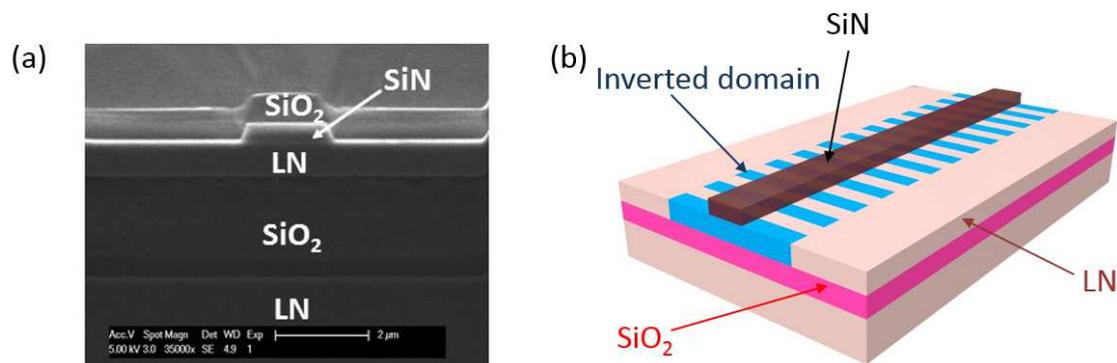
Figure 5: (a) Cross-section SEM of fabricated Si<sub>3</sub>N<sub>4</sub>-LNOI waveguide, (b) schematic of thin film PPLN wavelength converter.
