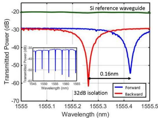
Figure 3: Spectral transmission of the forward and backward propagating light
