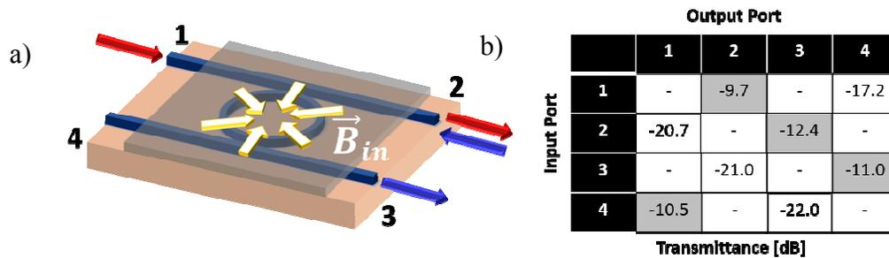
Figure 4: a) Schematic of the circulator, and b) scattering matrix values for the device
