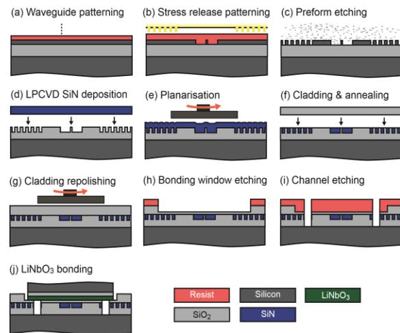
Figure 2: Processing flow.
