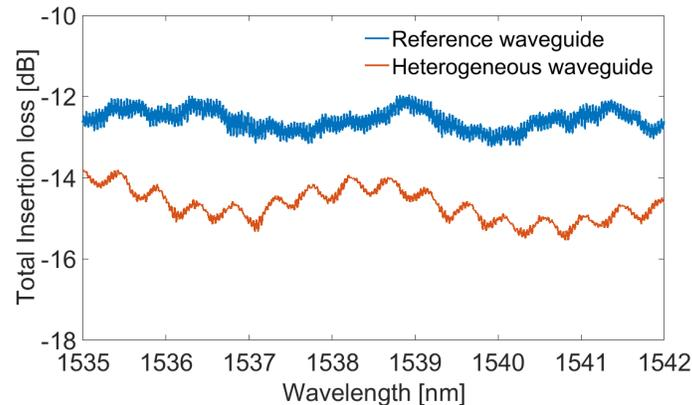
Figure 3: Spectra of total insertion loss.
