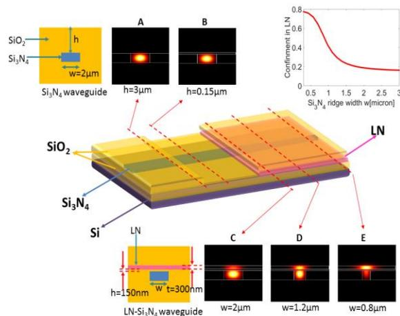
Figure 1: Cross-section schematics of waveguide and taper, and mode profile simulations.
