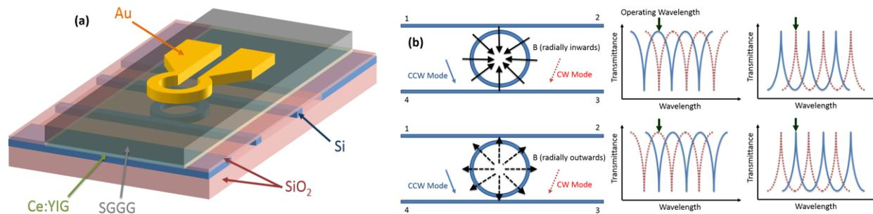
Figure 1: (a) Schematic of the microring optical circulator. (b) The optical circulator can be configured on one of two ways depending on whether the magnetic field is radially inwards (top) or outwards (bottom).
