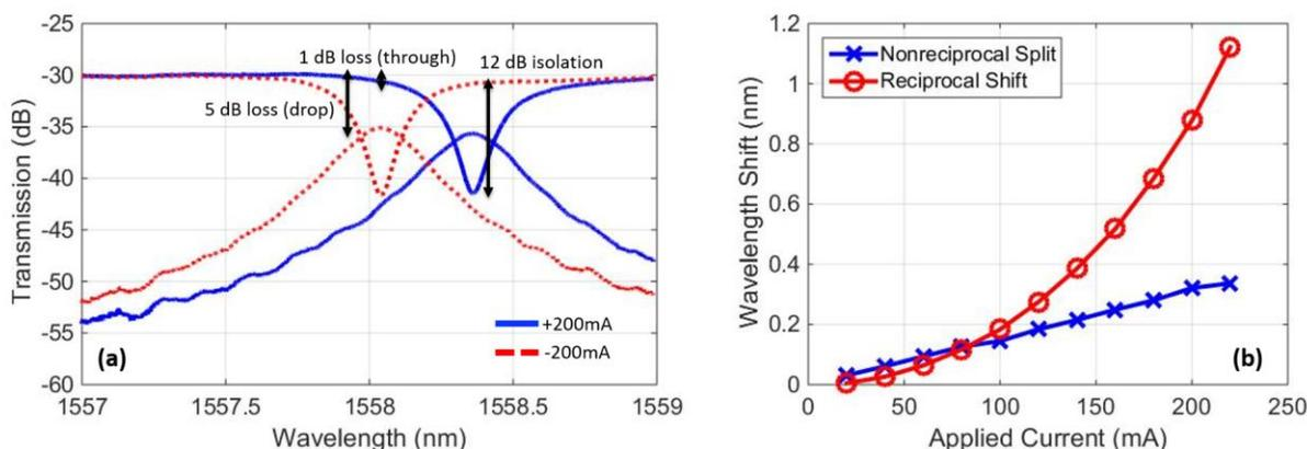
Figure 2: (a) Transmission spectrum at the through and drop ports of the circulator. (b) The nonreciprocal split (blue) and thermal induced redshift (red) of the resonance wavelength as a function of the applied current in the device.
