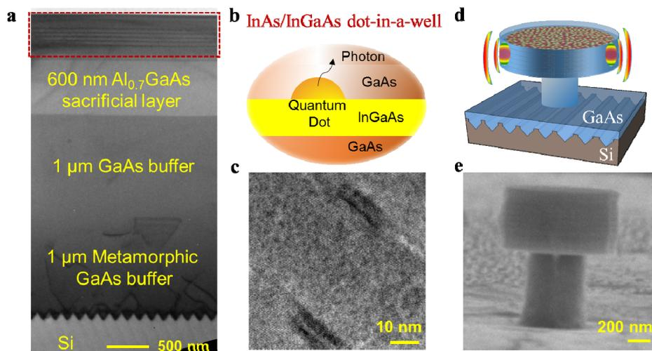
A schematic illustration of the epitaxial layers and QDs active region are shown in Fig. 1(a) and Fig. 1(b) respectively. A high resolution transmission electron microscope (TEM) image in Fig. 1(c) reveals the typical dot size, which has a diameter of  $\sim 21$  nm and height of  $\sim 6$  nm. By combining the colloidal lithography, dry-etching and subsequent wet-
