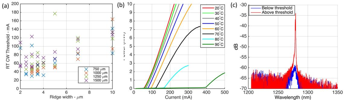
Fig. 2. (a) Threshold current for various cavity sizes. (b) Continuous wave lasing up to 90°C by a 1500x3.5  $\mu\text{m}^2$  device. (c) Electroluminescence spectra near and above threshold at room temperature demonstrating ground state lasing at 1280 nm.
