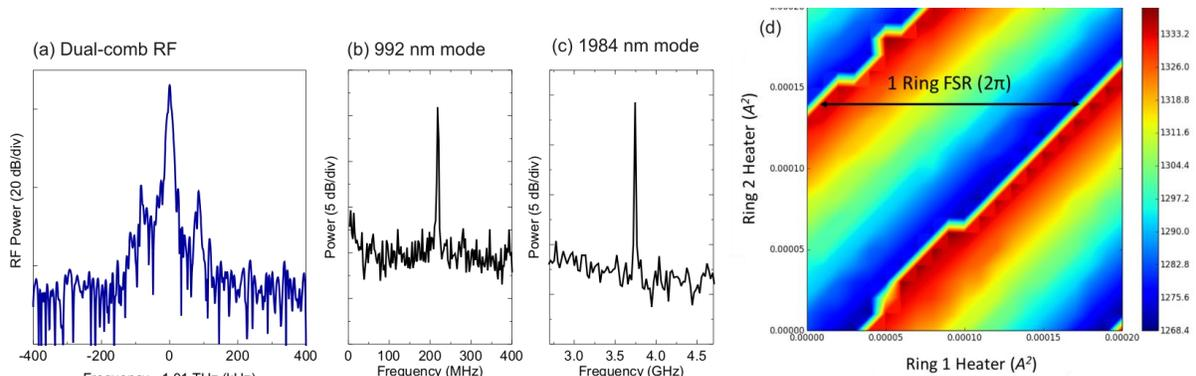
**Figure 2: RF outputs of the dual Kerr comb indicating low-noise operation. (a) Repetition rate beat between the pump THz and silica comb, (b) 992 nm heterodyne beat with the second harmonic generation of the ECDL, and (c) 1984 nm heterodyne with the ECDL. (d) Tuning map of the O-band tunable laser for this demonstration, showing mode hopping free tuning using the two ring resonators.**
