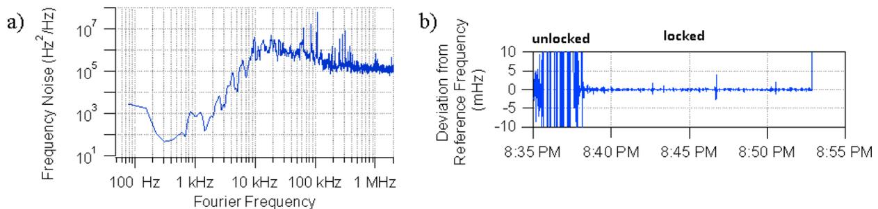
**Figure 3: Results of the O-band tunable laser locked to the THz comb. (a) In-loop PSD of locked frequency noise, and (b) 1 second gate in-loop counter measurement for locking greater than 15 minutes.**
