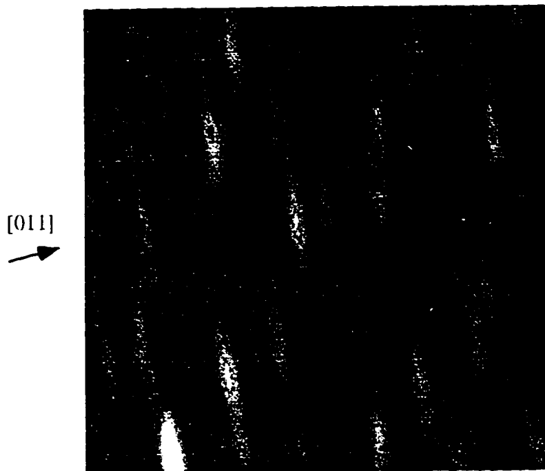
Figure 4-6 3\ \mu\text{m} \times 3\ \mu\text{m} \times 4\ \text{nm} AFM image of QDAFM-02, which is the GaAs buffer layer on which the InGaAs is grown.
