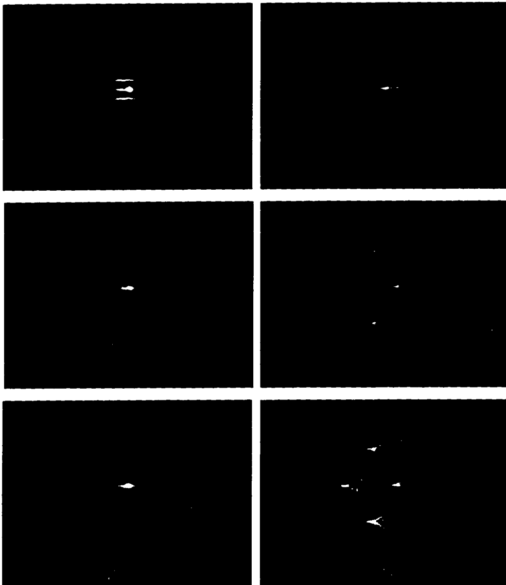
Figure 4-1 RHEED images along the [0\bar{1}1] azimuth after deposition of (a) 0 MLs, (b) 3.5 MLs, (c) 7.1 MLs, (d) 8.0 MLs, (e) 8.8 MLs, and (f) 9.7 MLs of \text{In}_{0.3}\text{Ga}_{0.7}\text{As} by alternating MBE..
