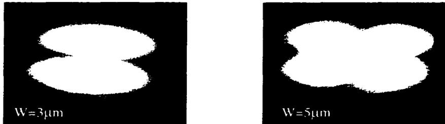
Figure 4.10. The near field patterns of the fundamental mode and the second order mode of fused vertical couplers.
