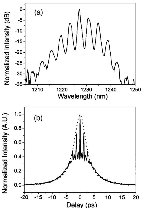
Fig. 5. (a) Output spectrum and (b) its corresponding autocorrelation trace of the multiwavelength Cr:forsterite laser output when the cover glass is turned  $50^\circ$  from normal incidence. The dotted curve in (b) is a Lorenzian fit.
