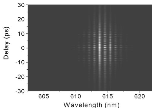
Fig. 3. SHG FROG trace of the multiwavelength Cr:forsterite laser output when the cover glass is inserted normally to the laser beam.
