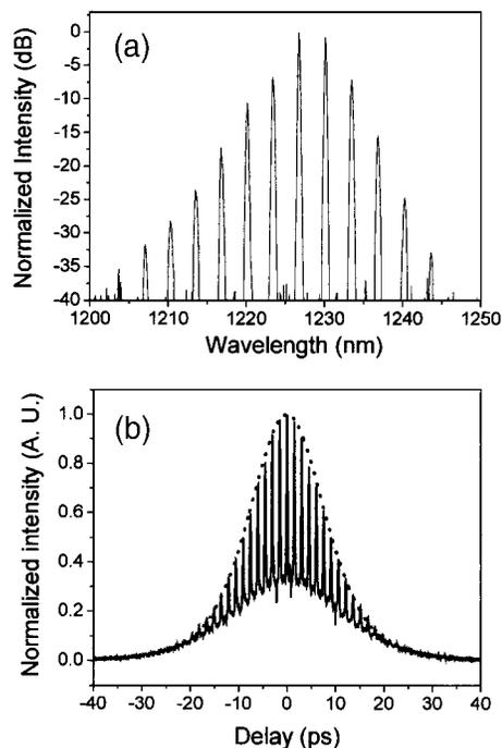
Fig. 2. (a) Output spectrum and (b) its corresponding autocorrelation trace of the multiwavelength Cr:forsterite laser output when the cover glass is inserted normally to the laser beam. The dotted curve in (b) is a  $\text{sech}^2$  fitting.
