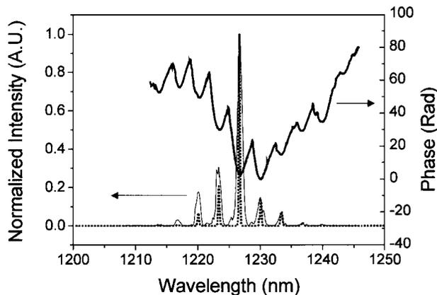
Fig. 4. Recovered intensity and phase spectra for the condition of Fig. 3. Dotted curve, the measured spectrum.
