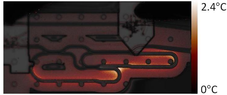
Figure 3.17. Thermal image of the heater when supplied with 30mW(4V), showing non-uniform heating at the hairpin bend in the center due to crosstalk.
