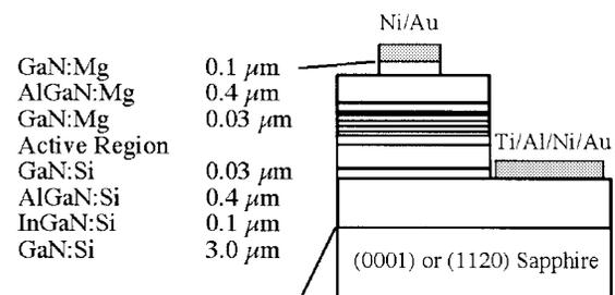
Fig. 1. Epitaxial layer structure and contacting scheme for laser diodes.
