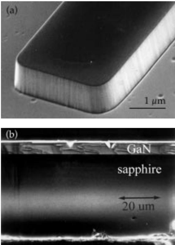
Fig. 2. SEM photographs of (a) RIE etched facets on c-plane sapphire test structures and (b) cleaved facets on a-plane sapphire.
