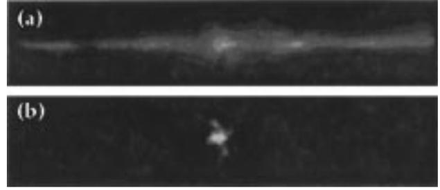
Fig. 5. Near-field of cleaved facet laser diode (a) below threshold and (b) above threshold under pulsed operation.
