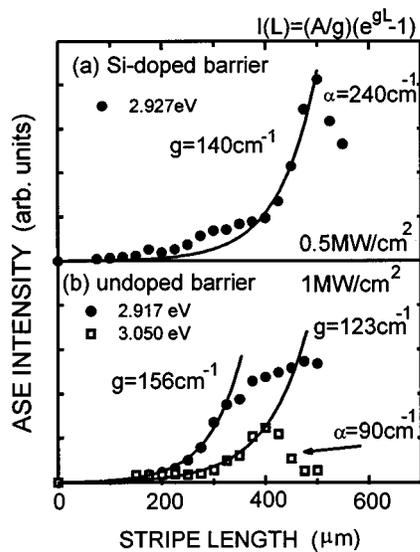
FIG. 2. ASE intensity as a function of  $L$  for MQW LD wafers with (a) Si-doped and (b) undoped barriers measured with the excitation power densities of 0.5 and 1 MW/cm<sup>2</sup>, respectively. Net modal gain  $g$  was obtained through fitting the data using Eq. (1), the fitting curves being drawn by solid lines.
