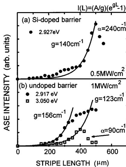
FIG. 2. ASE intensity as a function of  $L$  for MQW LD wafers with (a) Si-doped and (b) undoped barriers measured with the excitation power densities of 0.5 and 1 MW/cm<sup>2</sup>, respectively. Net modal gain  $g$  was obtained through fitting the data using Eq. (1), the fitting curves being drawn by solid lines.
