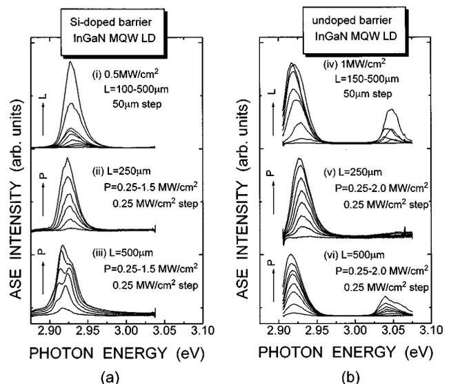
FIG. 1. ASE spectra of InGaN/InGaN MQW LD wafers having ten QWs with (a) Si-doped and (b) undoped In<sub>0.04</sub>Ga<sub>0.96</sub>N barriers. ASE spectra were recorded for different excitation stripe lengths ( $L$ ) [traces (i) and (iv)] and pumping power densities ( $P$ ) [(ii), (iii), (v), and (vi)].
