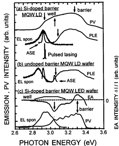
FIG. 3. Comparison of PV, PLE, spontaneous EL, EA, ASE, and lasing EL spectra for wafers of (a) Si-doped barrier MQW LD, (b) undoped barrier MQW LD, and (c) Si-doped barrier MQW LED. Respective resonance energies in the wells and barriers are indicated by arrows or an arc.
