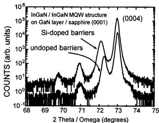
FIG. 4. Logarithmic plots of  $2\theta/\omega$ -scan XRD patterns for the Si-doped and undoped barrier MQW structures grown under the same conditions as LD wafers.
