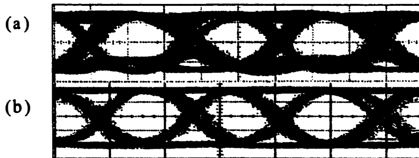
Figure 2.8 Eye diagrams of (a) the 30 Gbit/s input (100 mV/div; 13 ps/div), and (b) the 3 Vpp output of three cascaded amplifiers (750 mV/div; 20 ps/div).
