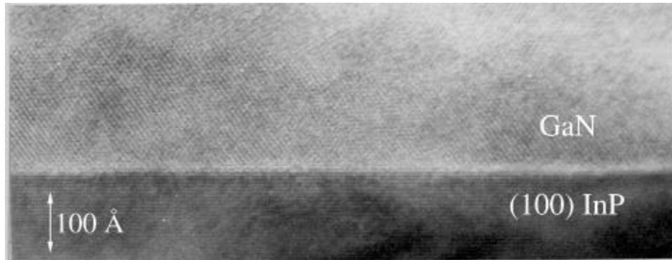
Figure 10. A TEM micrograph of an InP/GaN fused interface is shown. Fusion was performed at 750°C for 60 minutes.
