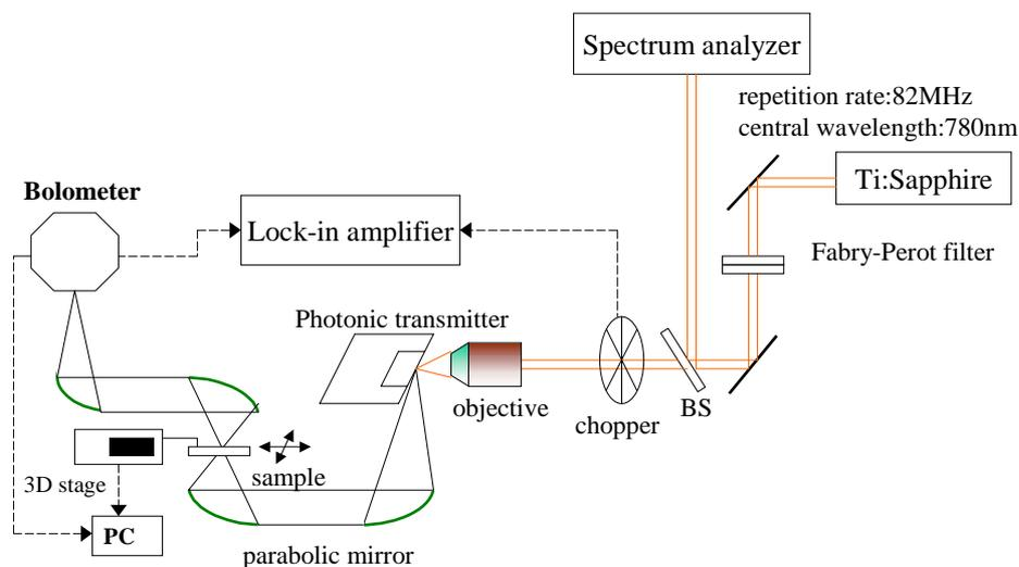
Fig. 1 Schematic diagram of the quasi-CW THz imaging system.
