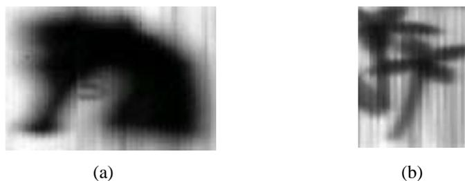
Fig. 2. Quasi-CW THz images of various samples. (a) A dried seahorse acquired with a 1THz radiation frequency. (b) Fresh flowers with water acquired with a 945GHz radiation frequency.
