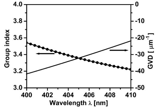
Fig. 1. Measured group index and GVD of an InGaN MQW laser diode at a current of 30 mA.
