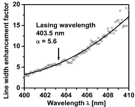
Fig. 2. Measured linewidth enhancement factor of an InGaN MQW laser diode under bias current of 25–30 mA with 1-mA step. The open circles are the measured data and the solid line is a polynomial fit to the data.
