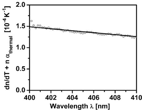
Fig. 3. Measured temperature variation of refractive index of an InGaN MQW laser diode under bias current of 25 mA and temperatures of 20.0 °C–21.5 °C. The open circles are the measured data and the solid line is a linear fit to the data.
