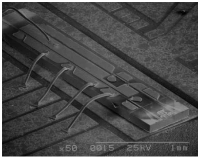
Fig. 2. Electron micrograph of transmitter device.
