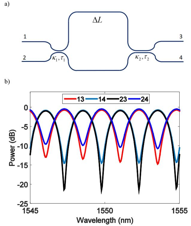
Fig. 1. a) Schematic of an UMZI. b) Optical spectra of transmissions through a UMZI structure. The spectra were simulated with the coupling ratios of the two couplers being 0.3 and 0.4, path length difference  $\Delta L = 500 \mu\text{m}$  and a couplers, which are what we want to calculate. In the next step, we will derive the values of  $\alpha$ ,  $\theta_1$  and  $\theta_2$  from the directly measurable values of  $R_{13}$ ,  $R_{14}$ ,  $R_{23}$  and  $R_{24}$ .
