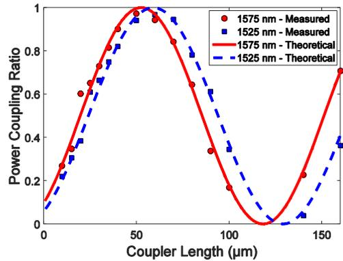
Fig. 5. The coupling ratio versus coupler length of the Si directional couplers at two wavelengths 1525 nm and 1575 nm. The measured data are plotted together with theoretical fitting curves.
