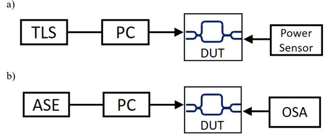
Fig. 2. a) The measurement setup using a tunable laser source (TLS), a single mode fiber polarization controller (PC) and a power sensor. b) An alternative configuration using a broadband source (e.g. ASE) with an optical spectrum analyzer (OSA).
