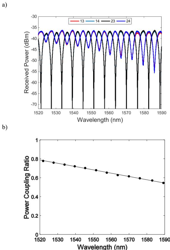
Fig. 4. a) Optical spectra of the transmissions through the UMZI fabricated on Si waveguides. The path length difference is 150  $\mu\text{m}$ . b) Coupling coefficients of the directional coupler calculated from the transmission spectra shown in 4.a.
