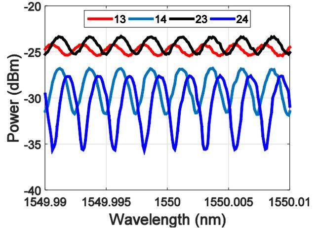
Fig. 3. Optical spectra of the transmissions through the UMZI fabricated on  $\text{Si}_3\text{N}_4$  waveguide platform. The path length difference is 62.1 cm. The peaks and valleys do not line-up due to the limited  $\pm 1$  pm of swept wavelength repeatability.
