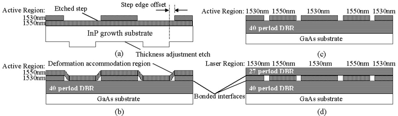
Fig. 1. Process flow cross-sections for fabrication of dual-wavelength VCSEL array
