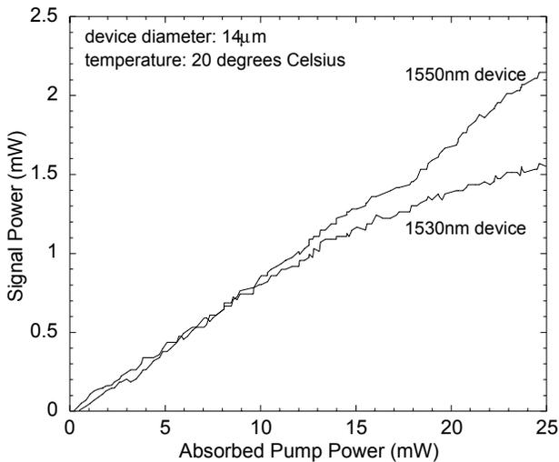
Fig. 2. Signal power versus absorbed pump power for the dual-wavelength VCSEL chip
