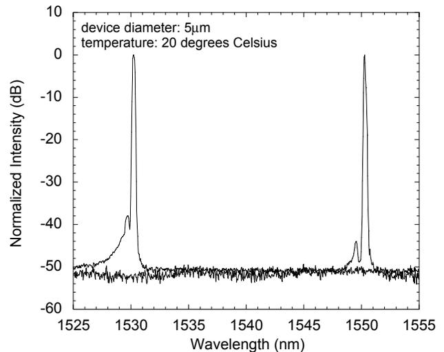
Fig. 3. Superimposed lasing spectra of dual-wavelength VCSEL chip
