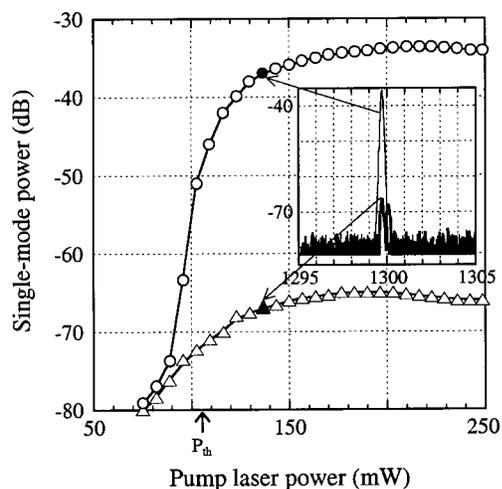
FIG. 5. Polarization-resolved single-mode output power of the VCSEL vs pump laser power. The polarizer was at  $[233]$  axis (circle) or at  $[0\bar{1}1]$  axis (triangle) of the VCSEL. Inset is spectra at 137 mW pump power (filled marks).
