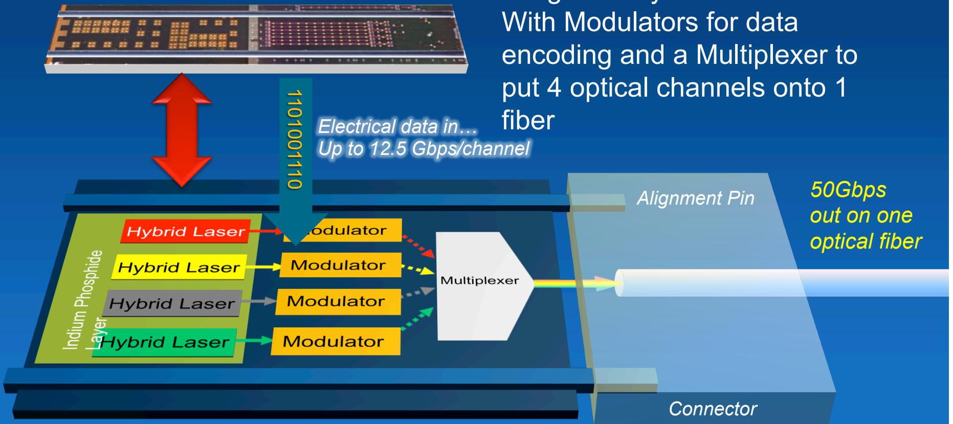
Parallel channels are key to scaling bandwidths
