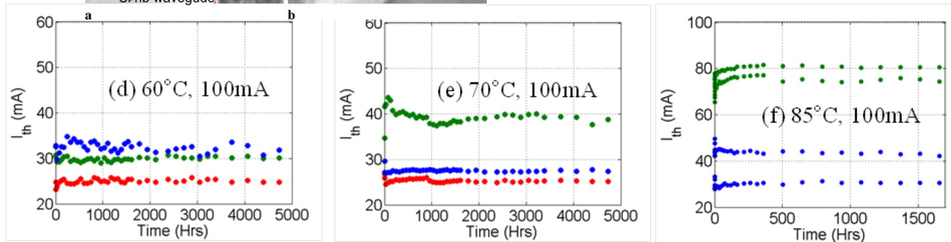
Time to reach 50% degradation in threshold current at 70°C is >40,000hrs
