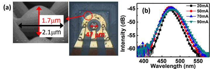
Figure 2. (a) A top-view of the demonstrated LED chip and the zoom in picture of light-emitting aperture and PS substrate. (b) Measured EL spectra of demonstrated LED.
