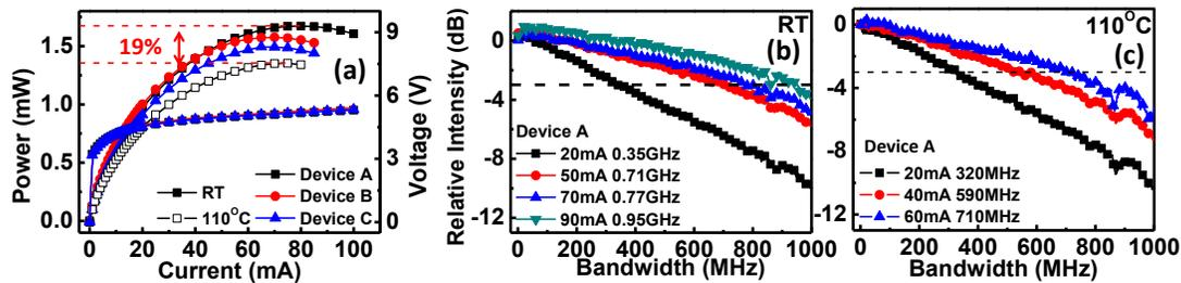
Figure 3. (a) Measured L-I-V curves under RT (solid symbols) and 110°C (open symbols) operations of demonstrated LEDs. Measured bias dependent E-O frequency responses of device A under RT (b) and 110°C operations, respectively.
