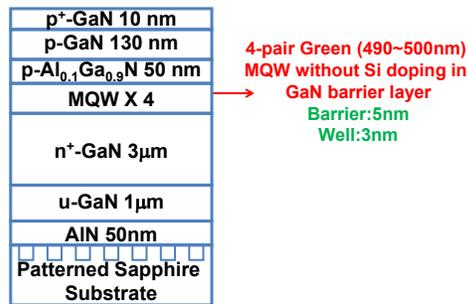
Figure 1. The conceptual cross-sectional view of epitaxial layer structure of demonstrated device. Such Figure was not drawn according to scale for clearness
