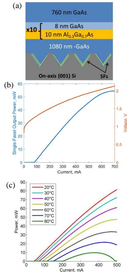
Fig. 3 (a) A schematic of GaAs template on V-groove Si (001). (b) L-I curves from the quantum laser diodes grown on V-groove Si. (c) Temperature-dependent CW L-I curve from an  $8 \times 1200 \mu\text{m}^2$  HR coated device.
