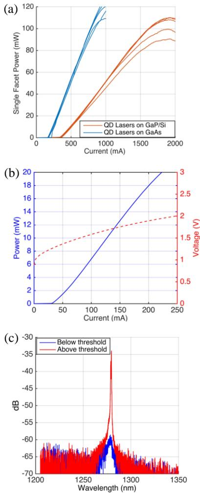
Fig. 2 (a) L-I curves measured from InAs QD broad-area ( $20 \mu\text{m}$ ) lasers grown on GaAs (blue) and GaP/Si (red), (b) RT CW L-I-V curves and (c) lasing spectra from GaP/Si laser diode.
