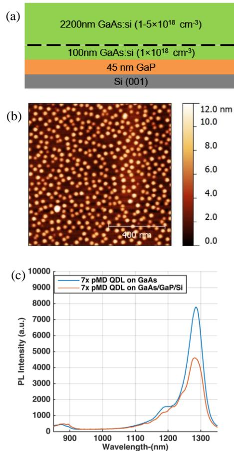
Fig. 1 (a) A schematic illustration of the GaAs/GaP/Si (001) template. (b) A  $1 \times 1 \mu\text{m}^2$  AFM image of InAs QD grown on GaAs. (c) Room-temperature PL spectra from InAs QDs grown on GaAs substrate and on on-axis GaP/Si substrate,
