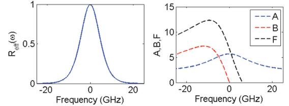
Fig. 3. (left) Normalized reflection of ring-resonator and cavity mirror combination (right) Linewidth reduction factor of the laser as a function of frequency offset from resonance calculated using eqs. 1,2,3 and 4 ( $\alpha_H=4$ ). The combined effect of both contributions is maximized at slight offset to lower frequencies than the ring resonance. [3].
