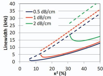
Fig. 5 Instantaneous linewidth as a function of high- $Q$  ring coupling strength for various propagation losses. (Full lines) Minimum linewidth with detuning, (Dashed lines) Linewidth at ring resonance. [11]
