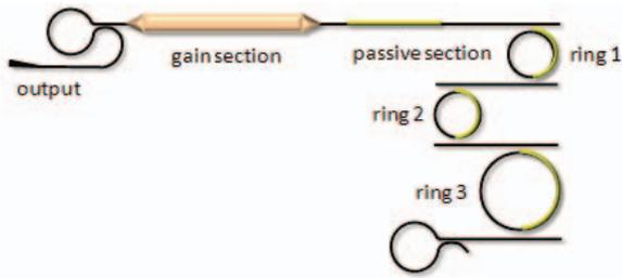
Fig. 4 Schematic of laser with high- $Q$  ring (ring 3) inside the cavity.
