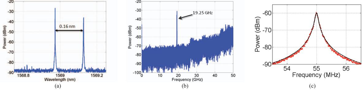
Fig. 2. (a) Optical spectra of two lasers comprising a photonic microwave generator (captured with high-resolution 20 MHz optical spectrum analyzer) (b) RF beat tone after high-speed detector (c) Measured linewidth and Lorentzian fit (50 kHz) of narrow-linewidth widely-tunable laser with monolithically integrated external cavity [3].
