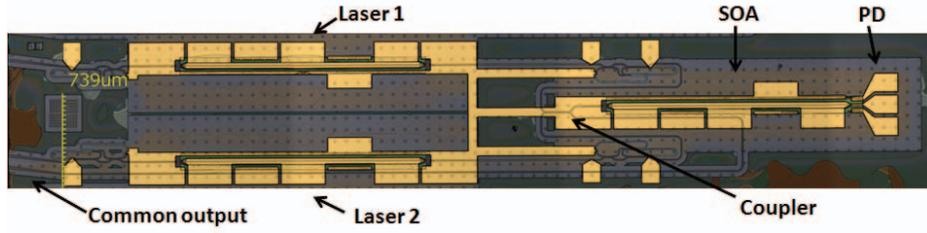
Fig. 1. Microscope image of the photonic microwave generator comprising of two tunable lasers, a coupler, booster semiconductor optical amplifier (SOA) and photodetector (PD). One arm of the 2x2 coupler goes to SOA and PD, other arm goes to the edge facet (common output).
