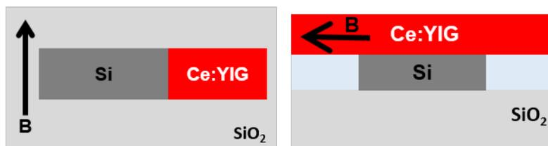
Figure 6. (left) The waveguide geometry required for magnetic field induced nonreciprocal phase shift for transverse electric (TE) modes. (right). The waveguide configuration required for TM modes.
