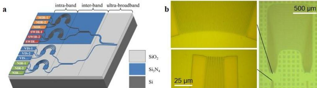
Fig. 1. (a) Integrated spectral beam combining application for this AWG. (b) Micrograph of the fabricated AWG showing detail of the free propagation region interface.
