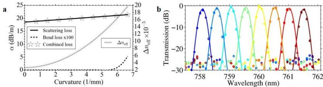
Fig. 2. (a) Scattering and bend losses simulated for a 760 nm wavelength. Also shown is the index shift,  $\Delta n_{\text{eff}}$ , from a nominal value of  $n_{\text{eff}} = 1.4945$  for all curvature, inverse of the bend radius, in each bend of the arrayed waveguides. (b) Measured transmission spectra (circles) and theoretical calculations (solid lines) for each channel represented by different colors.
