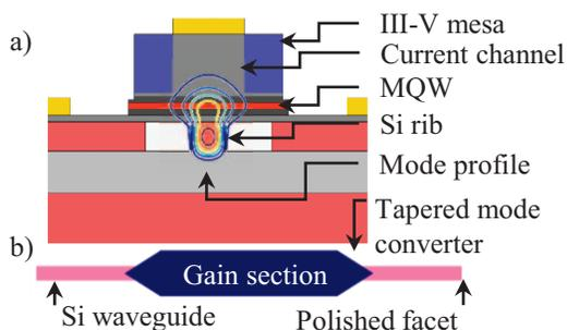
Fig. 1. a) Cross section of gain region b) plan-view schematic of amplifier
