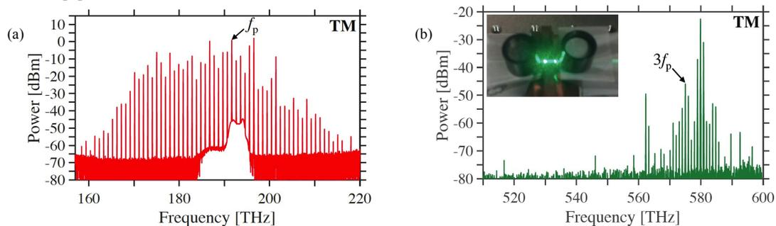
Fig. 2. (a) IR Kerr comb generated with a TM pump and (b) the corresponding GLC with 30 spectral lines. In (b), the inset shows a photograph of the probed device. The pump frequency  $f_p = 191.6$  THz and both IR and green combs have FSR = 977.2 GHz.
