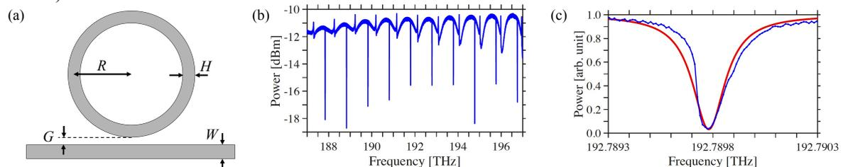
Fig. 1. (a) Top-view schematic of the ring microresonator. (b) Transmission spectrum and (c) fitting (in red) of the resonance near 192.8 THz.
