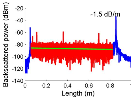
Figure 3: Optical backscatter reflectometer measurement of the ultra-low loss waveguide
