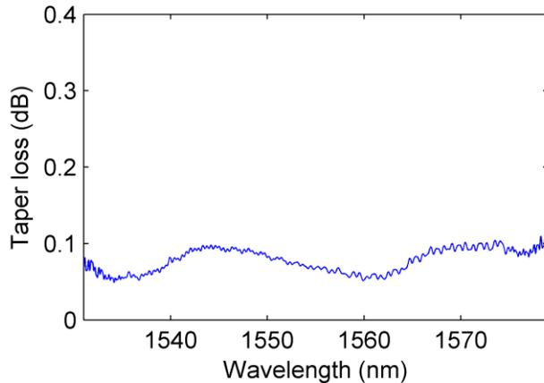
Figure 2: Transmission loss for a single taper versus wavelength.
