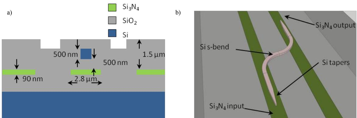
Figure 1: a) Cross section of the coupler region of the device. b) Overview of the taper test structure.
