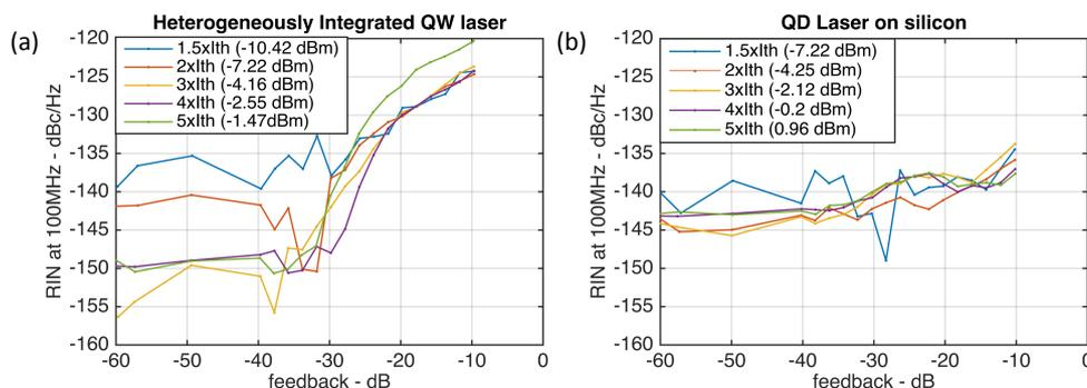
Fig. 3. RIN at 100 MHz versus feedback at five bias currents for a) a heterogeneously integrated quantum well laser on silicon with a 1.05 mm long gain section and 4  $\mu\text{m}$  wide current channel. b) A 1mm long by 3  $\mu\text{m}$  wide quantum dot laser on silicon.
