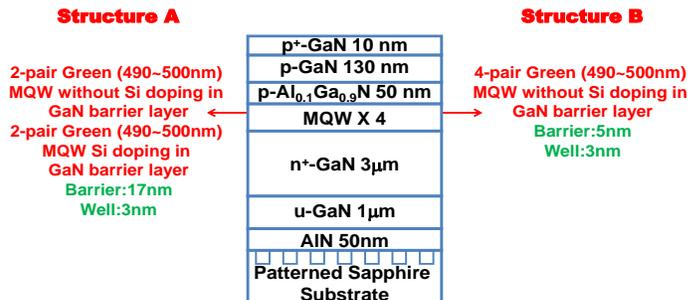
Figure 1. A conceptual cross-sectional view of epitaxial layer structures A and B. For clarity this figure is not drawn according to scale.
