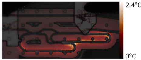
Fig. 10. Thermal image of the heater when supplied with 30 mW (4 V), showing non-uniform heating at the hairpin bend in the center due to crosstalk.
