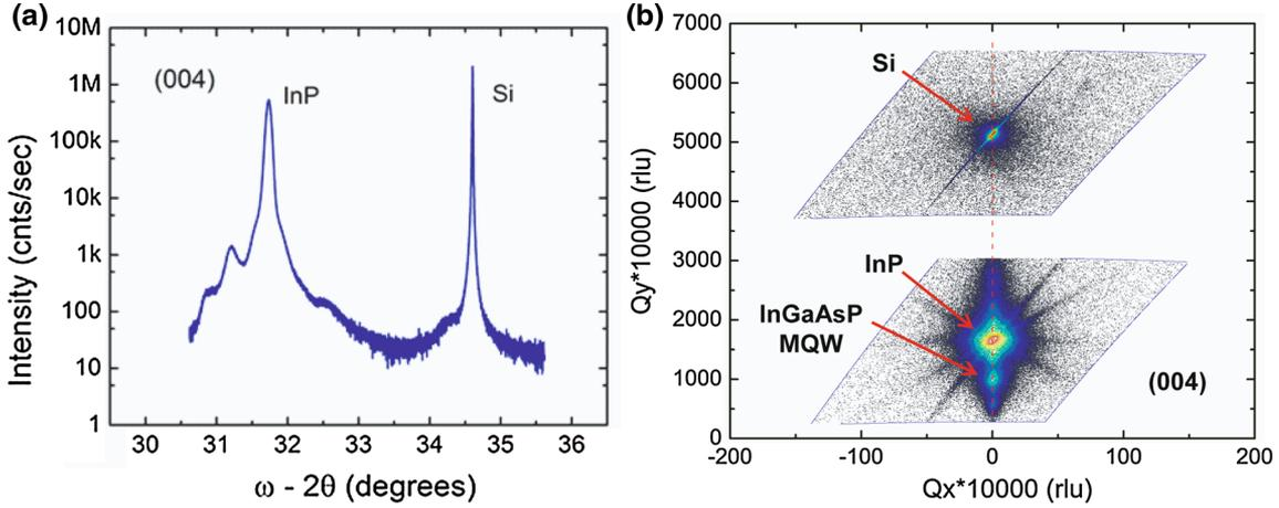
Fig. 3. (Color online) (a)  $\omega/2\theta$  scan centered on InP and showing the InP and Si diffraction peak around (004) Bragg reflections, (b) reciprocal space map of the PIN MQW structure around (004) Bragg reflections.
