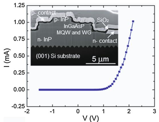
Fig. 7. (Color online)  $I$ - $V$  for a 900- $\mu\text{m}$ -long by 2.5- $\mu\text{m}$ -wide ridge fabricated on patterned (001) Si after InP nanowires regrow. Inset: SEM-focussed ion beam cross-section of one of the ridges fabricated on patterned (001) Si.
