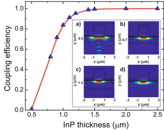
Fig. 4. (Color online) Dependency of the coupling efficiency on the InP buffer layer thickness for an input  $TE_0$  mode for a laser diode structure fabricated on coalesced InP on Si. Inset Simulations of  $TE_0$  mode profile when the InP coalesced thickness is (a) 500 nm, (b) 700 nm, (c) 1.2  $\mu\text{m}$ . (d) Simulation of the  $TE_0$  mode profile of the same structure grown on a native InP substrate.
