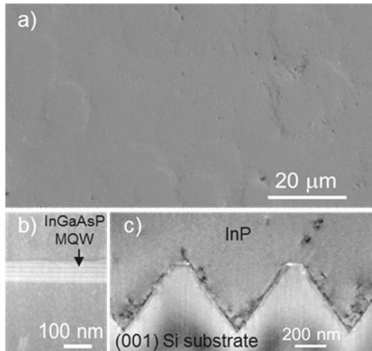
Fig. 5. (Color online) (a) SEM top-view image of the final surface after regrowth without any intermediate CMP step, (b) bright field TEM image of the MQW, (c) high-angle annular dark field scanning transmission electron microscopy image of the v-groove patterned on the Si and GaAs/InP seed layer.
