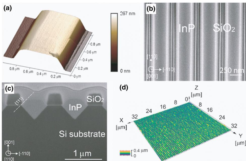
Fig. 2. (Color online) (a) AFM scan of InP nanowires, SEM (b) plan-view and (c) cross-section image of InP nanowires. (d) confocal 3D image of InP nanowires showing good uniformity in height over  $30 \times 30 \mu\text{m}^2$  large area. The small variation in color indicates small height variation.
