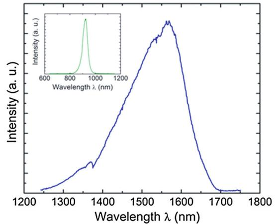
Fig. 6. (Color online) Photoluminescence of final laser structure showing 1567 nm emission after regrowth and (inset) of initial InP nanowires.
