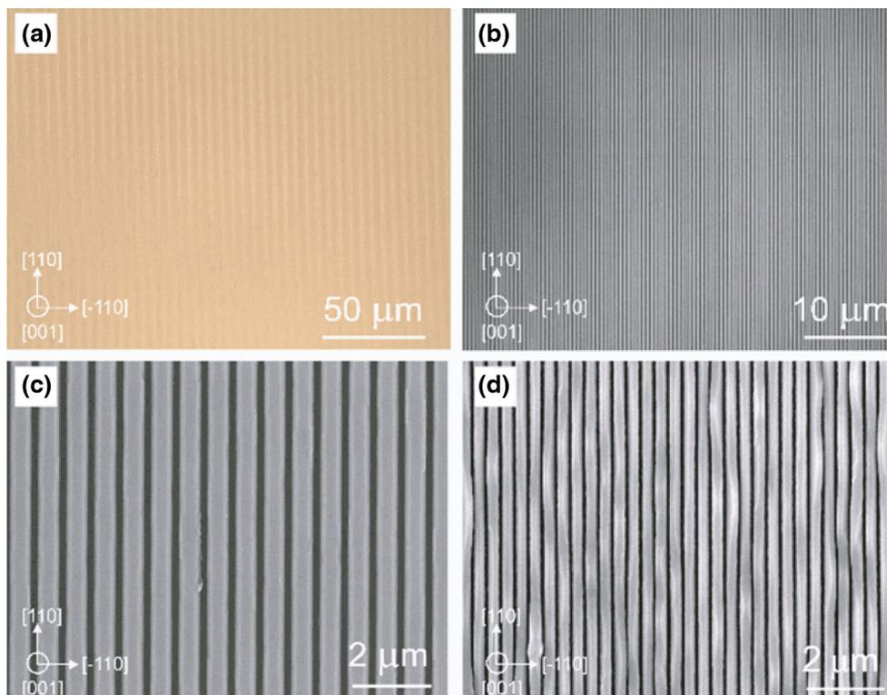
Fig. 1. (Color online) (a) Bright field optical and (b) SEM images of millimeter-long InP nanowires showing good uniformity over a large area, (c, d) SEM plan-view images showing difference in uniformity and smoothness of InP nanowires grown on two different trenches width and pitch size.
