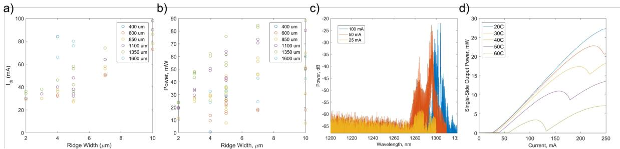
Figure 3. Scatterplots of (a) threshold current and (b) single facet output power for laser ridges of varying width and length grown on Si. (c) Lasing spectra of a 2.5x2.5x750  $\mu\text{m}^2$  ridge above threshold. (d) Power output versus bias current at elevated temperature for a 5x850  $\mu\text{m}^2$  device.
