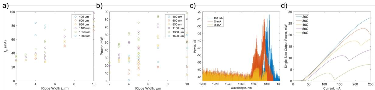
Figure 3. Scatterplots of (a) threshold current and (b) single facet output power for laser ridges of varying width and length grown on Si. (c) Lasing spectra of a  $2.5 \times 2.5 \times 750 \mu\text{m}^3$  ridge above threshold. (d) Power output versus bias current at elevated temperature for a  $5 \times 850 \mu\text{m}^2$  device.
