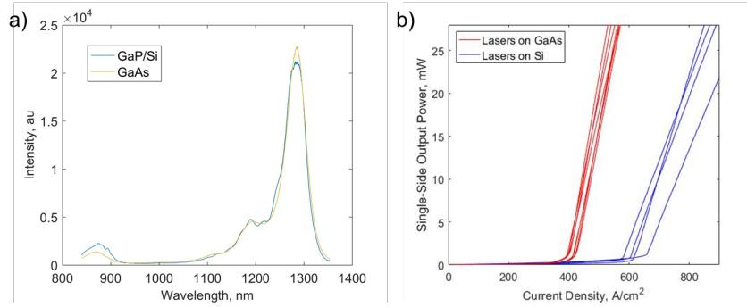
Figure 2. (a) Photoluminescence of as-grown laser material on GaAs and Si substrates. (b) Light output versus bias current density for 50x3100  $\mu\text{m}^2$  broad area devices on GaAs and Si showing a 1.5x increase in threshold.
