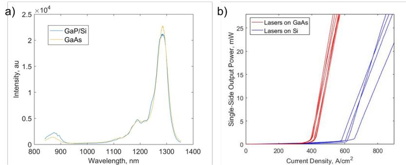
Figure 2. (a) Photoluminescence of as-grown laser material on GaAs and Si substrates. (b) Light output versus bias current density for  $50 \times 3100 \mu\text{m}^2$  broad area devices on GaAs and Si showing a 1.5x increase in threshold.
