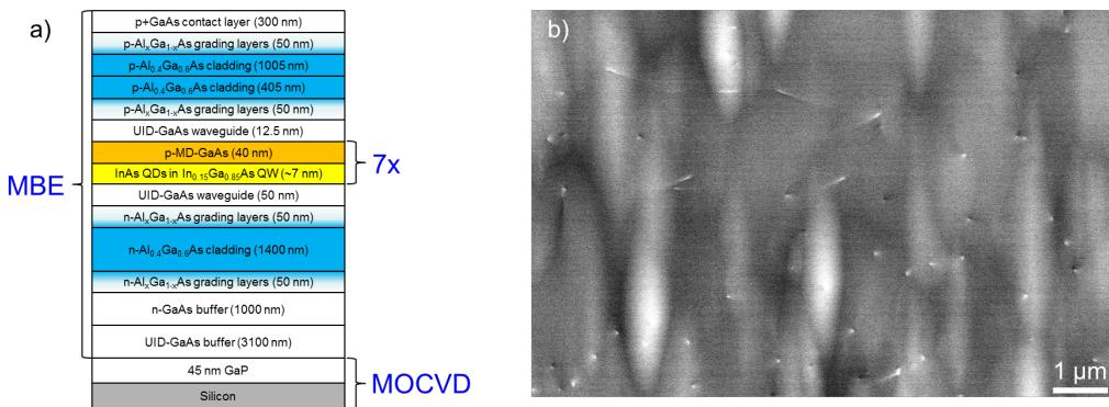
Figure 1. (a) Schematic of the laser structure. (b) Electron channeling contrast image of the uid-GaAs buffer surface. Pinpoints indicate threading dislocations.
