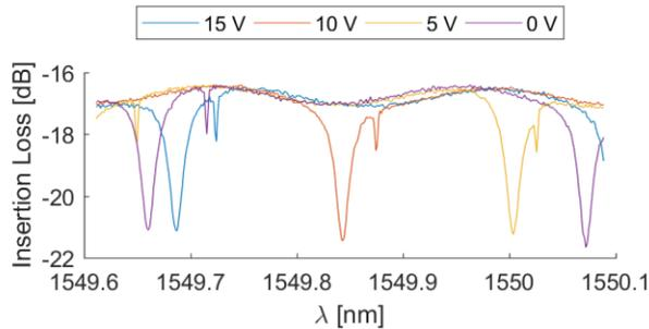
Fig 4. Ring resonator transmission spectrum for varying electrical bias and 86  $\mu\text{m}$  undercut. The deeper peak corresponds to the resonance of the (designed) fundamental TM mode, whereas the shallower peak corresponds to the fundamental TE mode.
