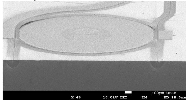
Fig 2. SEM of suspended nitride resonator with PZT actuator
