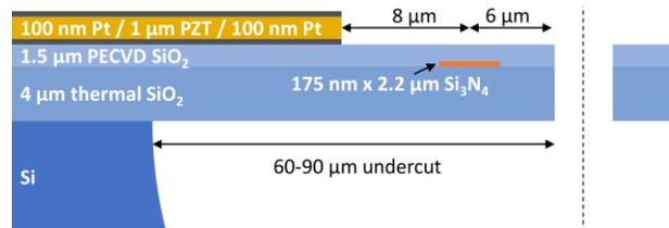
Fig 1. Cross-sectional schematic of ring resonator with PZT. The dotted line represents the symmetry of the cladding and substrate due to the isotropic  $\text{XeF}_2$  etch
