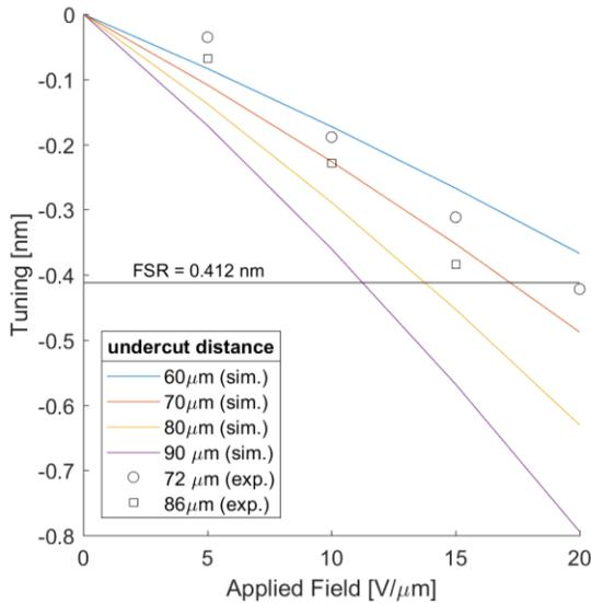
Fig. 3. Tuning vs applied electric field. Solid lines indicate simulation results. Data points indicate experimental results for varying undercut.
