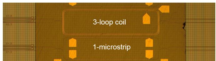
Fig. 10. Micrograph of integrated MZI optical circulators. Two electromagnetic configurations are shown in the figure, named 3-loop coil and 1-microstrip.
