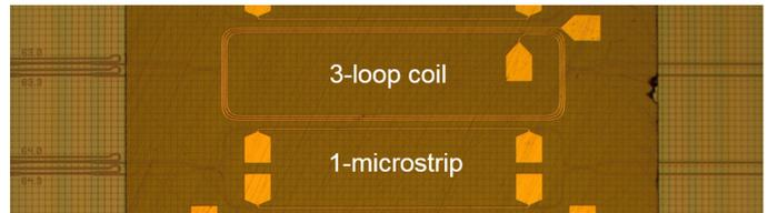
Fig. 10. Micrograph of integrated MZI optical circulators. Two electromagnetic configurations are shown in the figure, named 3-loop coil and 1-microstrip.
