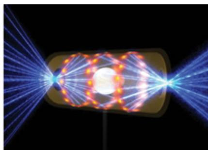
*This artist's rendering shows an NIF target pellet inside a hohlraum capsule with laser beams entering through openings on either end. The beams compress and heat the target to the necessary conditions for nuclear fusion to occur. Ignition experiments on NIF will be the culmination of more than 30 years of inertial confinement fusion*
