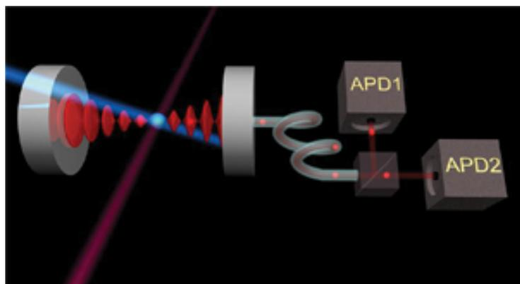
*A high-finesse optical cavity consisting of two mirrors traps and accumulates the photons emitted by the ion into a mode. The ion is excited cyclically by an external laser and at each cycle a photon is added to the cavity mode, which amplifies the light. (University of Innsbruck © Piet Schmidt)*
