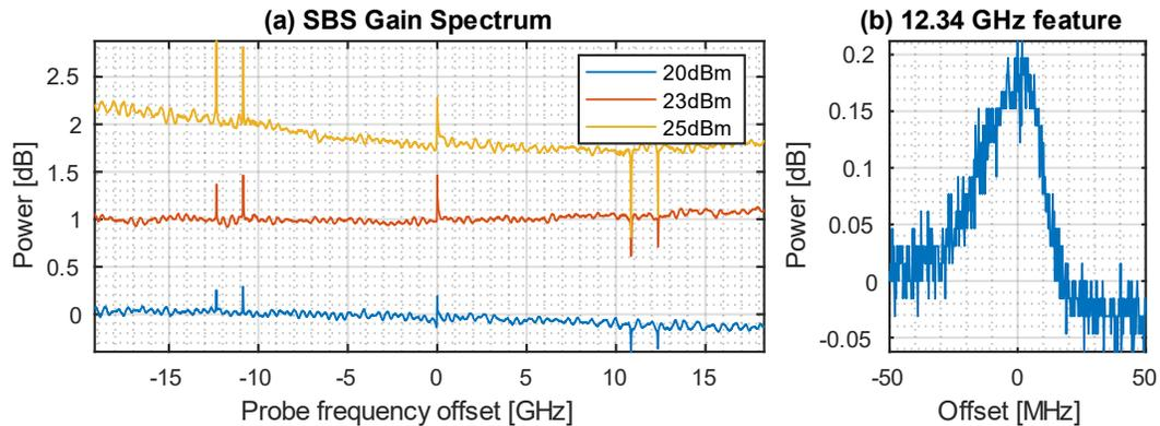
Fig. 2. (a) SBS gain spectrum of the probe with respect to a pump wavelength at 1550.1 nm, with pump power (into fiber) between 20 dBm and 25 dBm. (b) High resolution scan of the 12.34 GHz Brillouin peak with 25 MHz FWHM for 20 dBm power launched into fiber.
