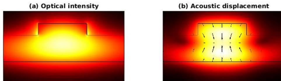
Fig. 1. (a) Optical intensity of the fundamental TE mode in the SBS waveguide at 1550 nm. (b) Physical displacement of the acoustic mode at 12.2 GHz, superimposed with arrows indicating the transverse components of displacement
